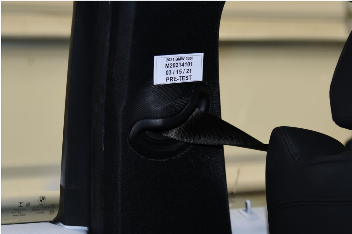
FIGURE 33. Pre-Test View of Belt Anchorage for Dummy
