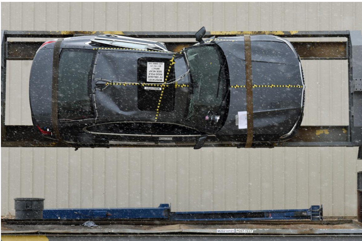
FIGURE 66. FMVSS No. 301 Static Rollover 90 Degrees
