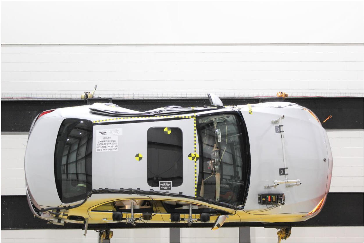
Figure A-97: FMVSS No. 301 Static Rollover 90 Degrees
