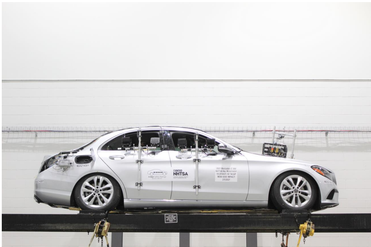
Figure A-96: FMVSS No. 301 Static Rollover 0 Degrees
