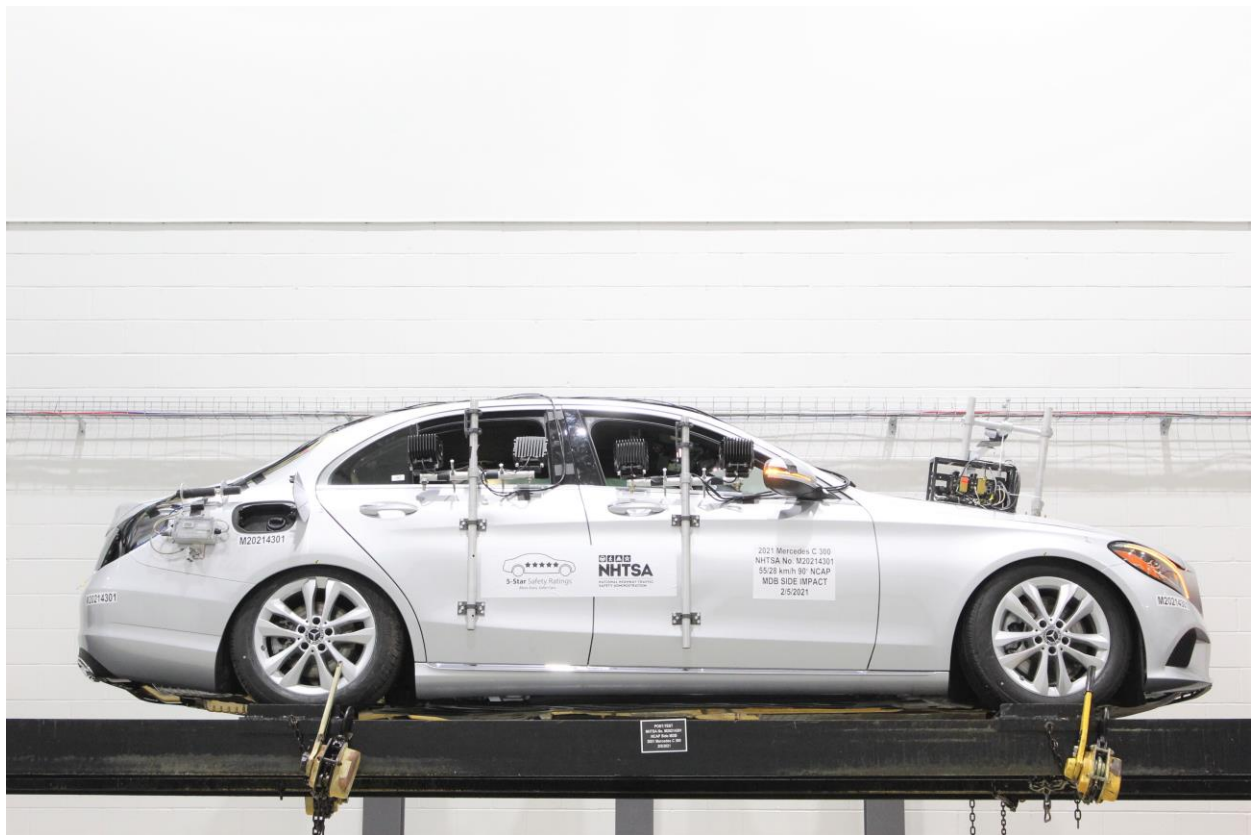
Figure A-100: FMVSS No. 301 Static Rollover 360 Degrees
