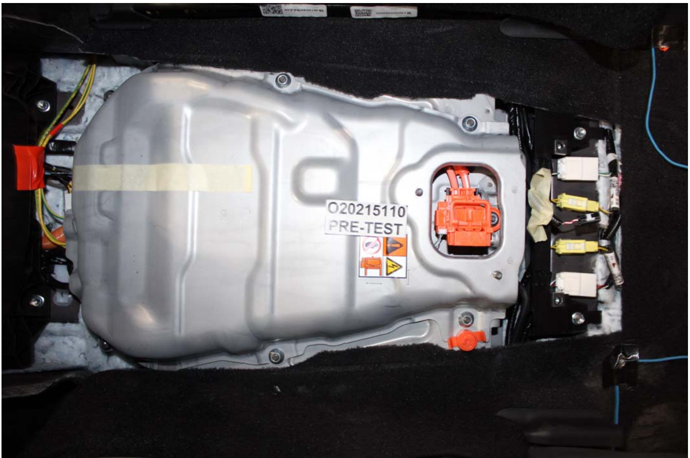
Photo No. 305-09 - Pre-Impact View of Propulsion Battery
