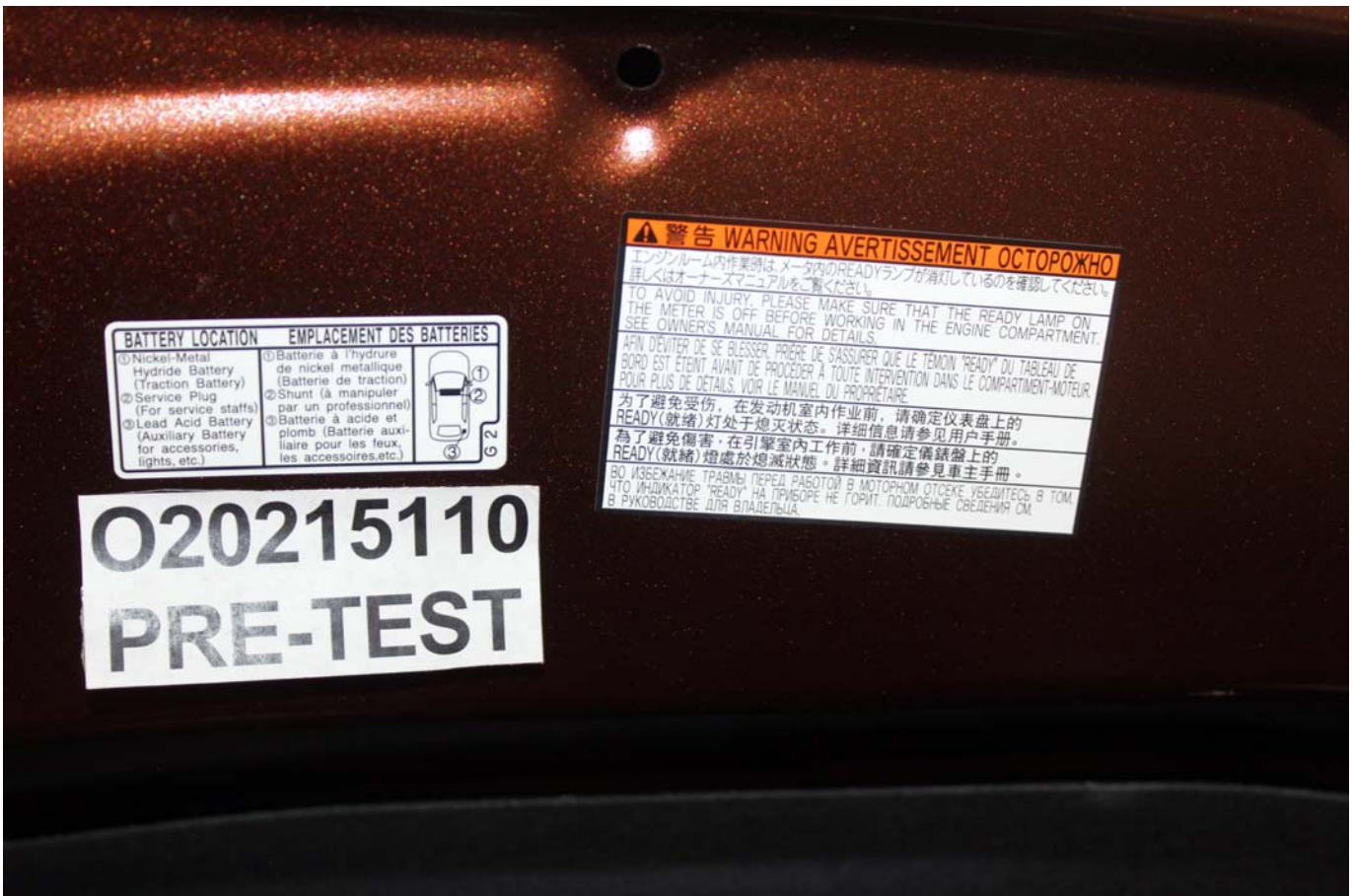
Photo No. 305-03 - First Responder Warning Label
