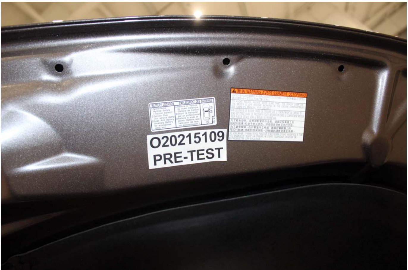
Photo No. 305-03 - First Responder Warning Label
