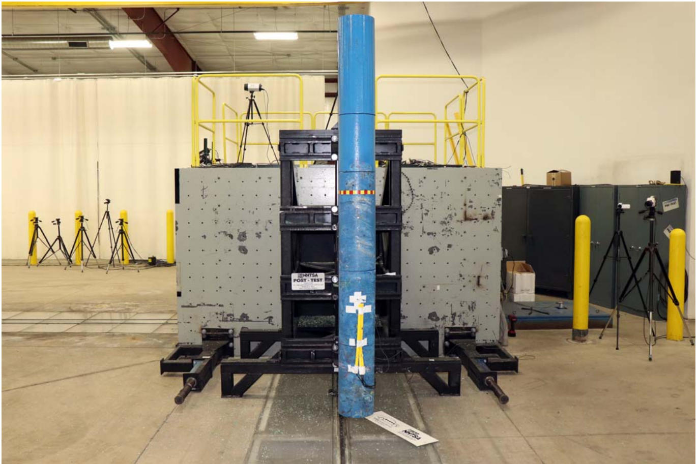
Photo No. 060 - Post-Test Pole Barrier Front View
