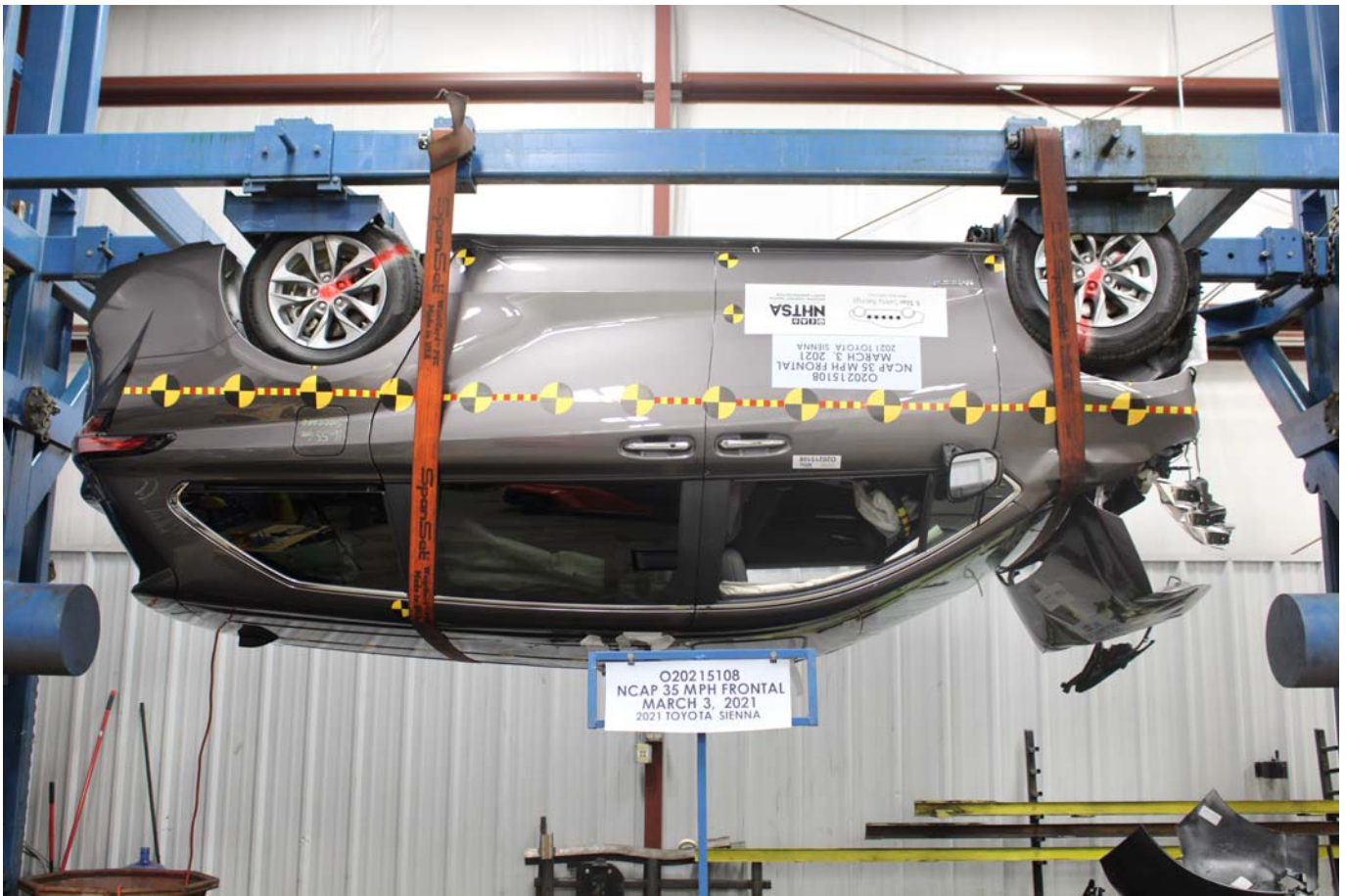
Photo No. 305-29 - FMVSS No. 305 Static Rollover at 180 Degrees
