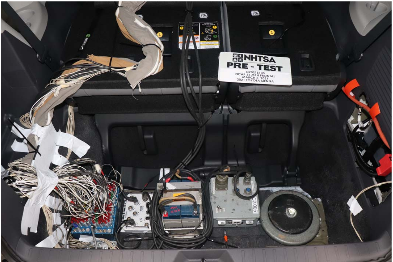
Photo No. 074 - Ballast Installed in Vehicle
