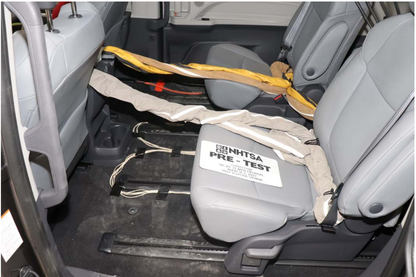
Photo No. 028 - Pre-Test Dummy Cable Routing
