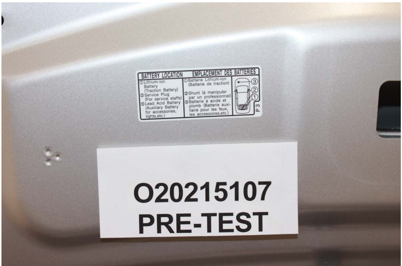
Photo No. 305-03 - First Responder Warning Label
