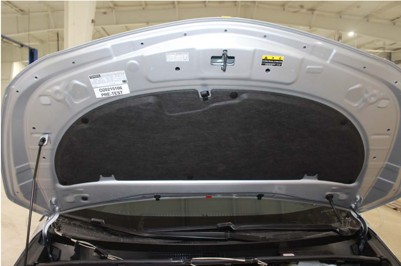
Photo No. 305-04 - First Responder Warning Location
