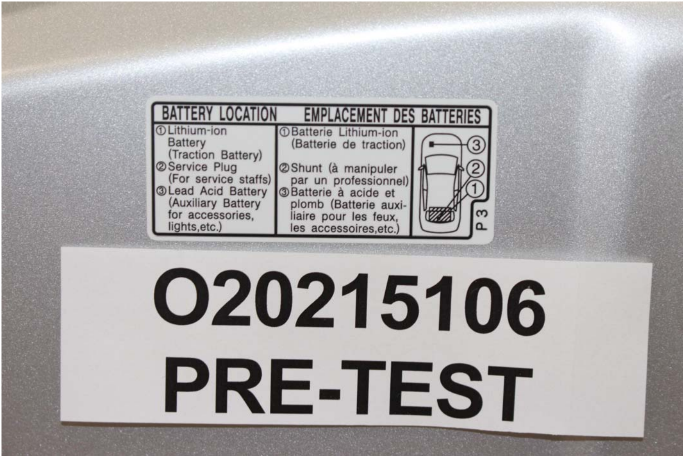
Photo No. 305-03 - First Responder Warning Label
