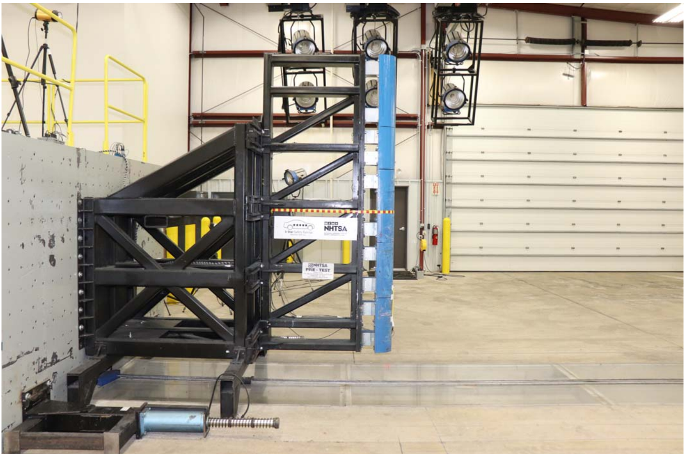
Photo No. 061 - Pre-Test Pole Barrier Side View
