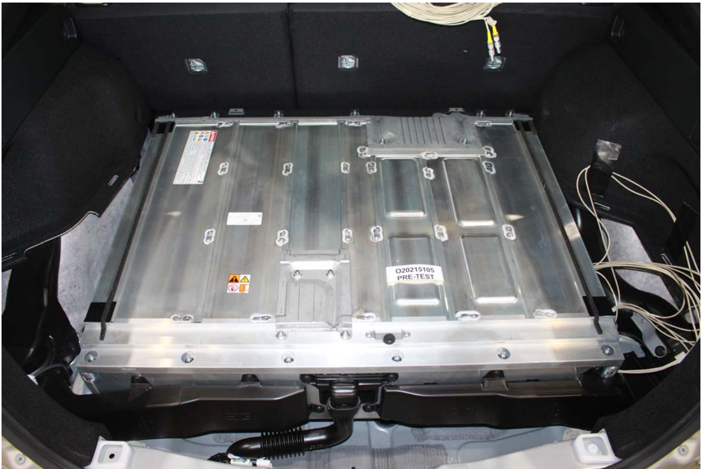
Photo No. 305-09 - Pre-Impact View of Propulsion Battery
