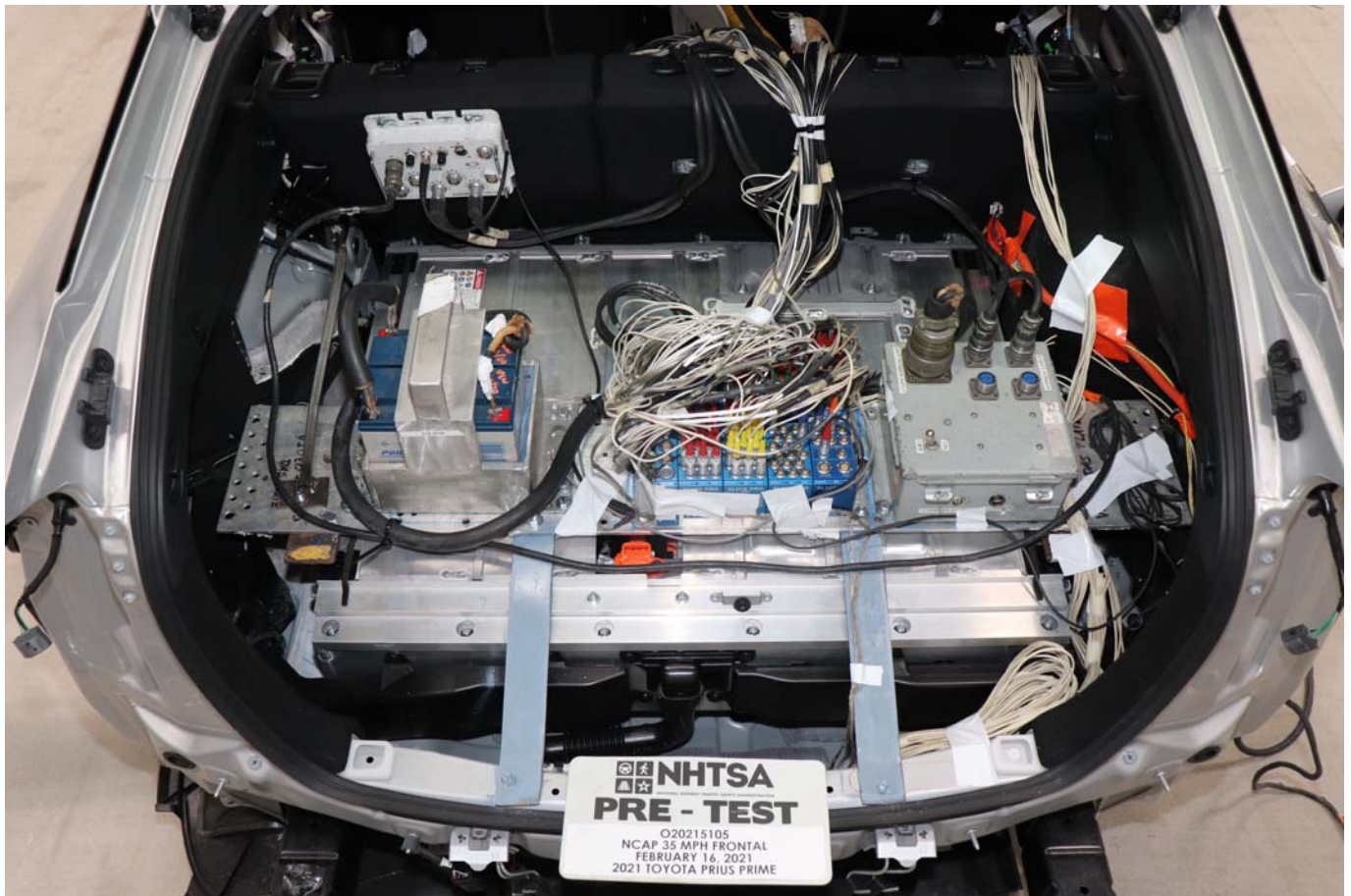
Photo No. 074 - Ballast Installed in Vehicle
