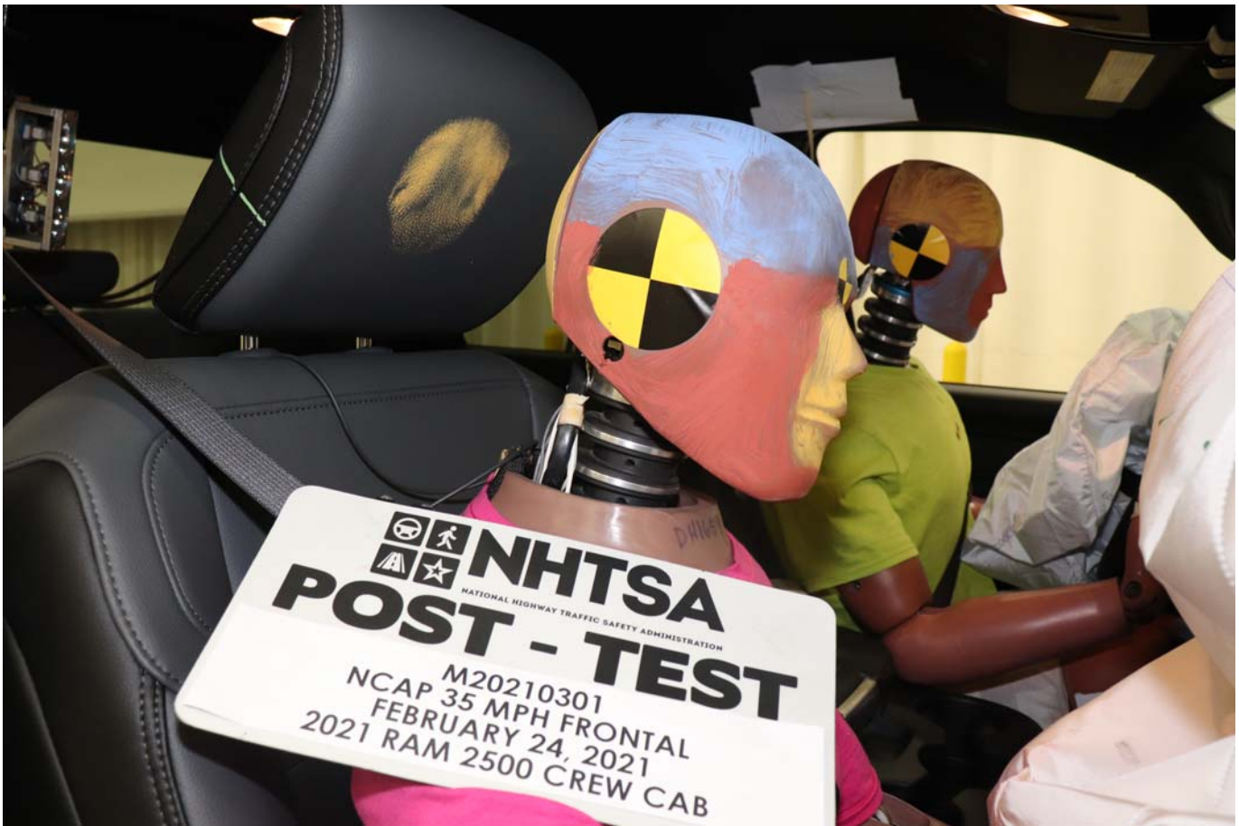
Photo No. 071 - Post-Test Passenger Dummy Face
