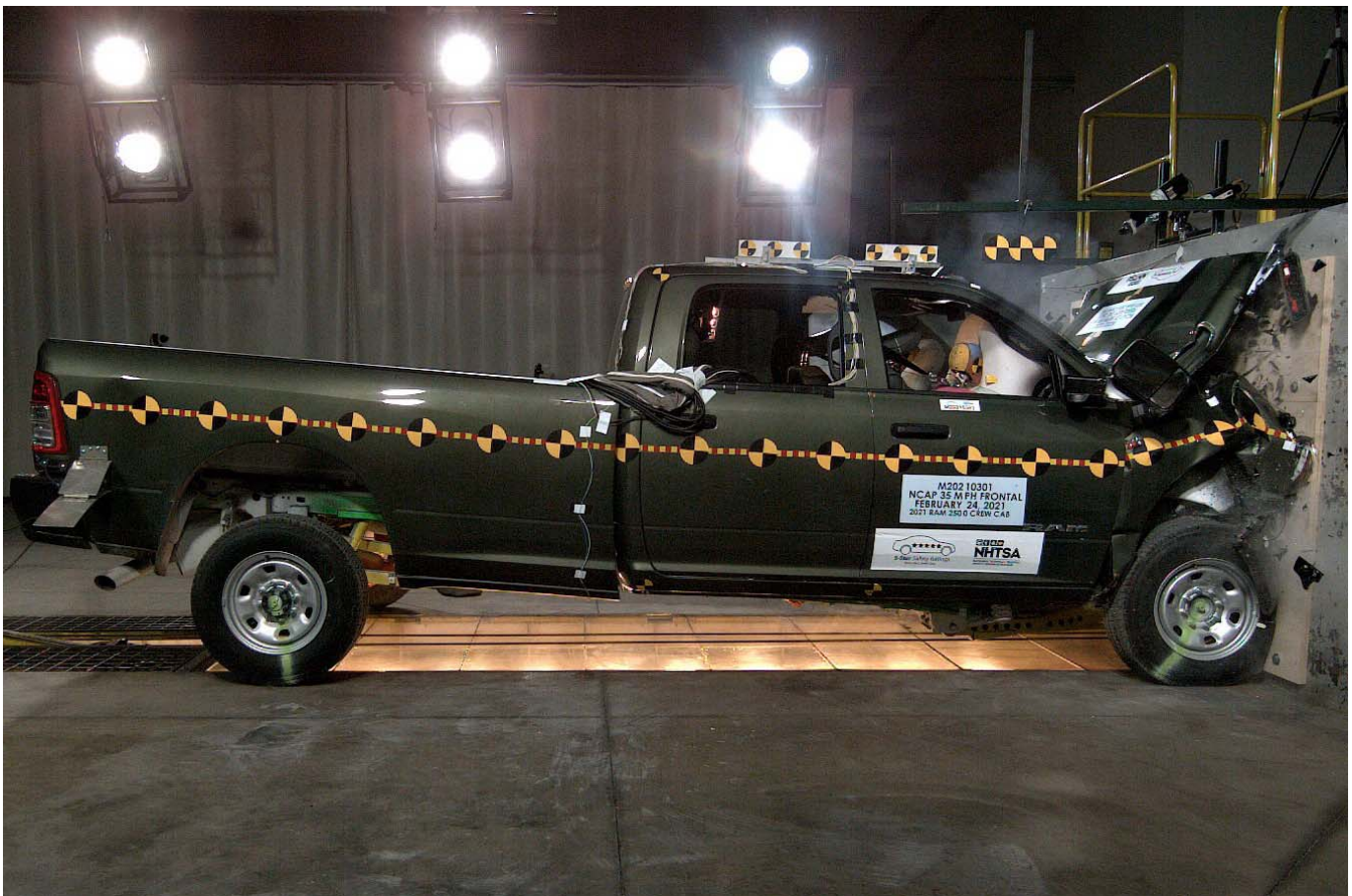
Photo No. 082 - 2021 Ram 2500 Crew Cab 4x4 Truck Frontal Impact Event
