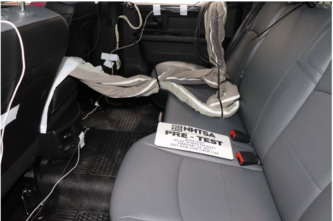
Photo No. 028 - Pre-Test Dummy Cable Routing
