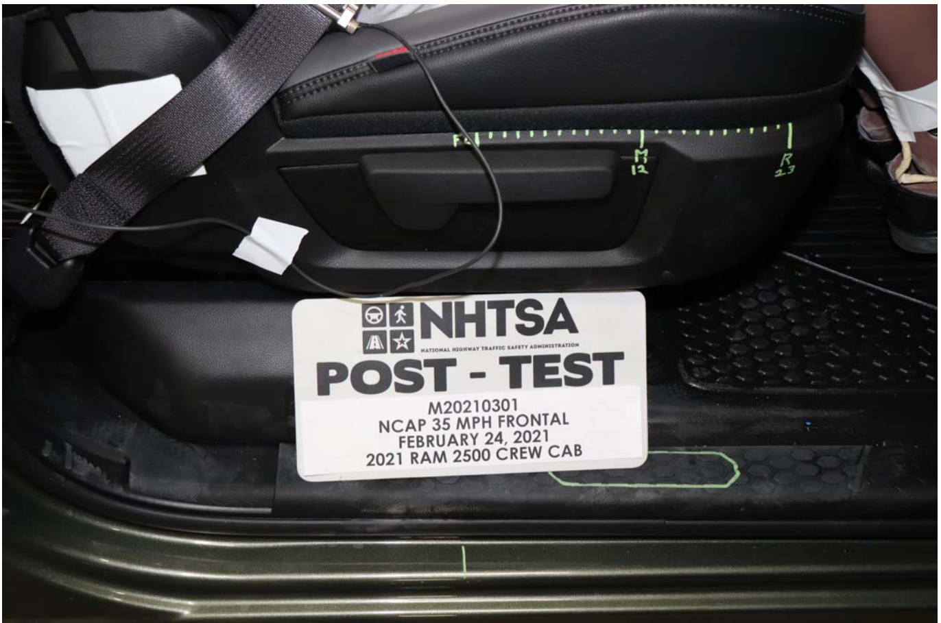
Photo No. 060 - Post-Test Passenger Seat Fore-Aft Markings
