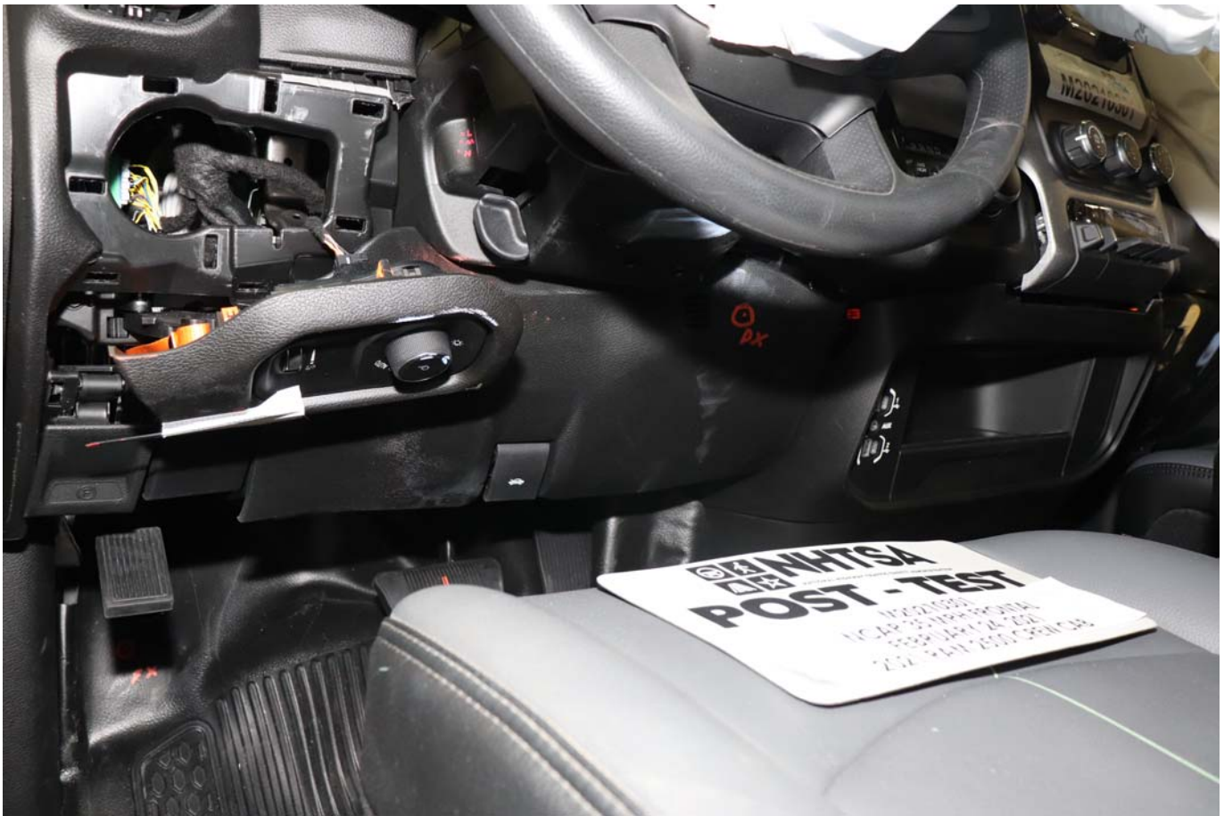
Photo No. 045 - Post-Test Driver Side Knee Bolster
