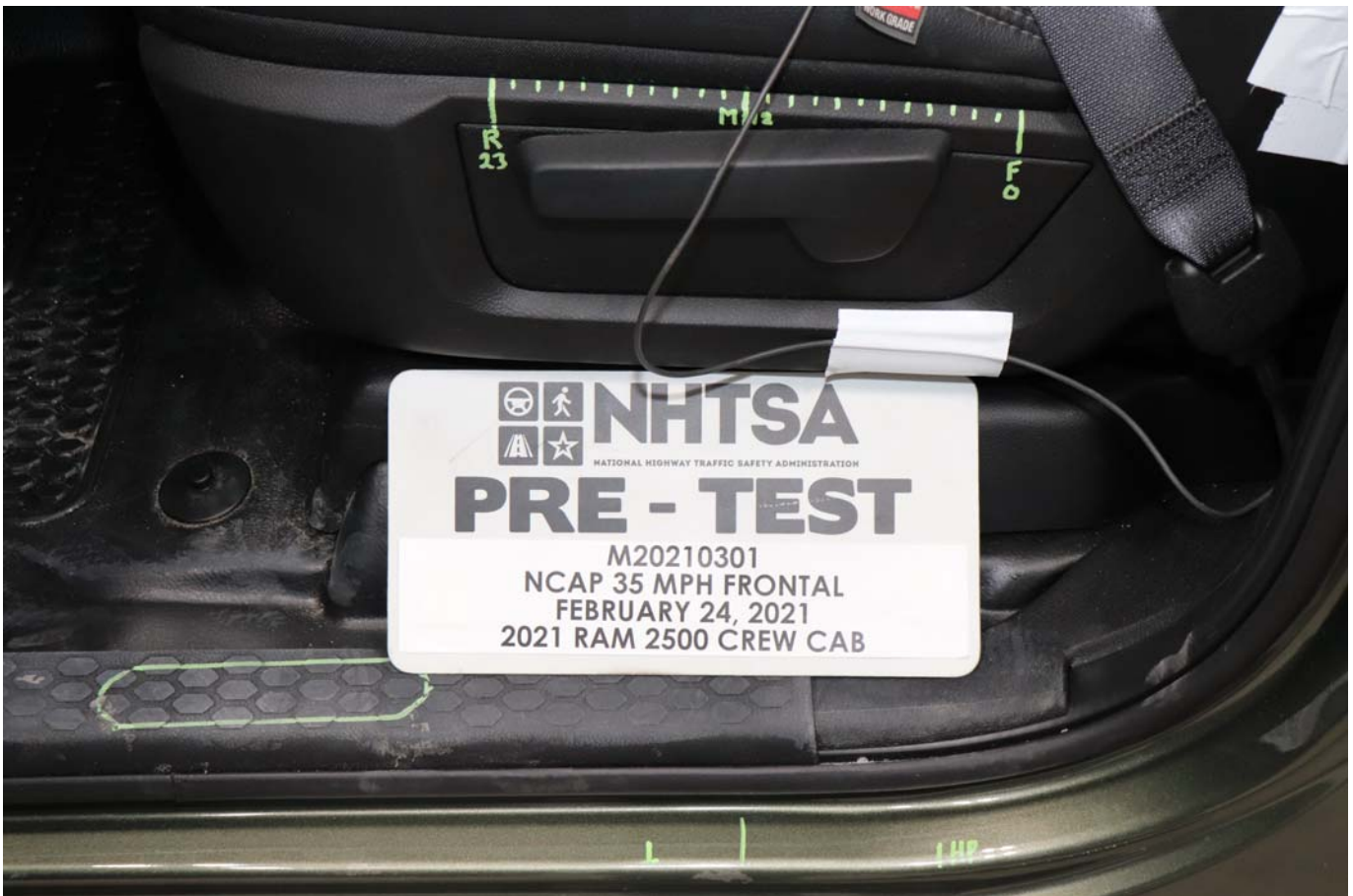
Photo No. 036 - Pre-Test Driver Seat Fore-Aft Markings
