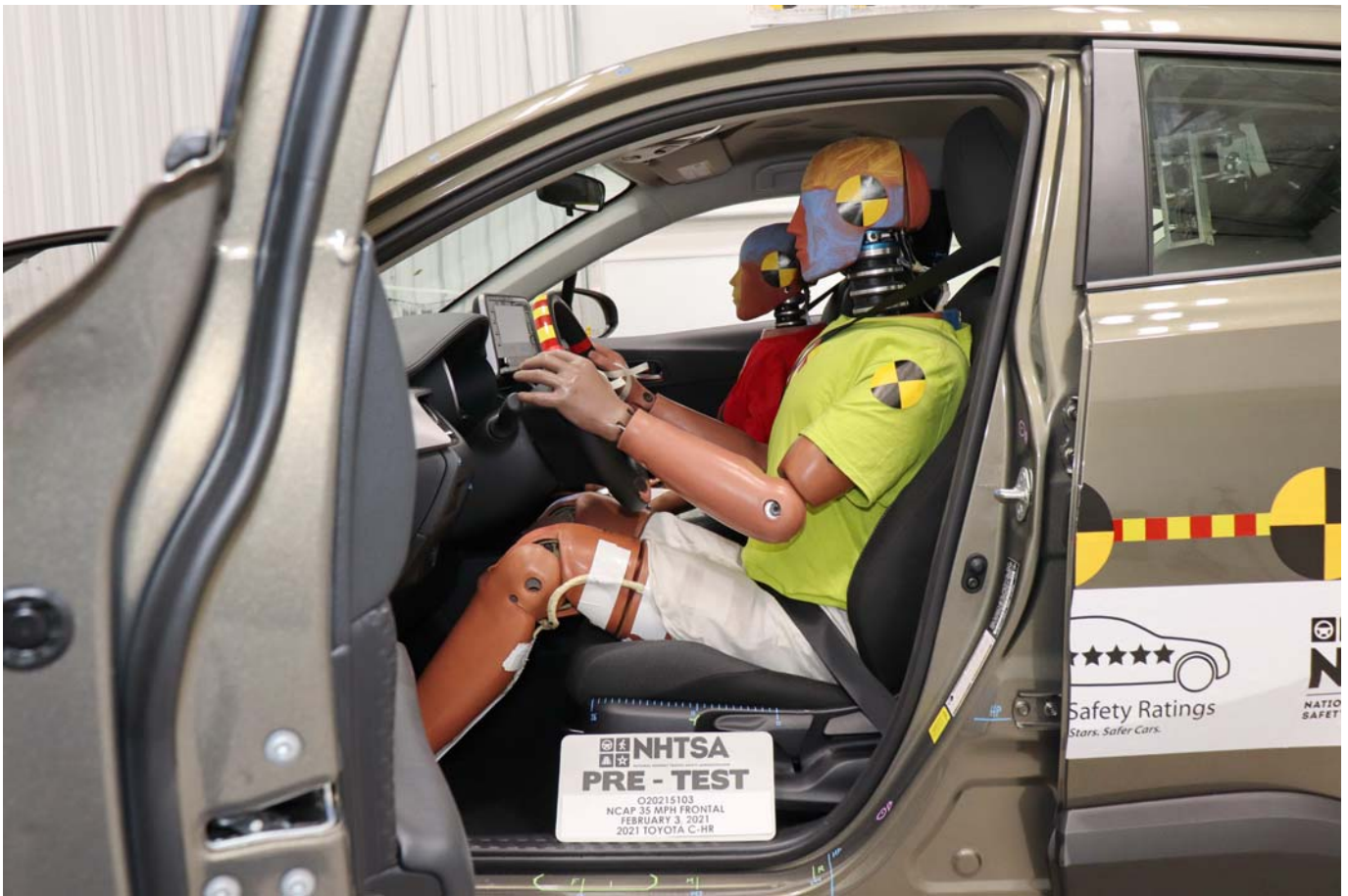
Photo No. 034 - Pre-Test Driver Dummy and Vehicle Interior
