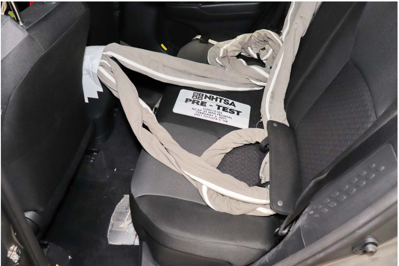
Photo No. 028 - Pre-Test Dummy Cable Routing
