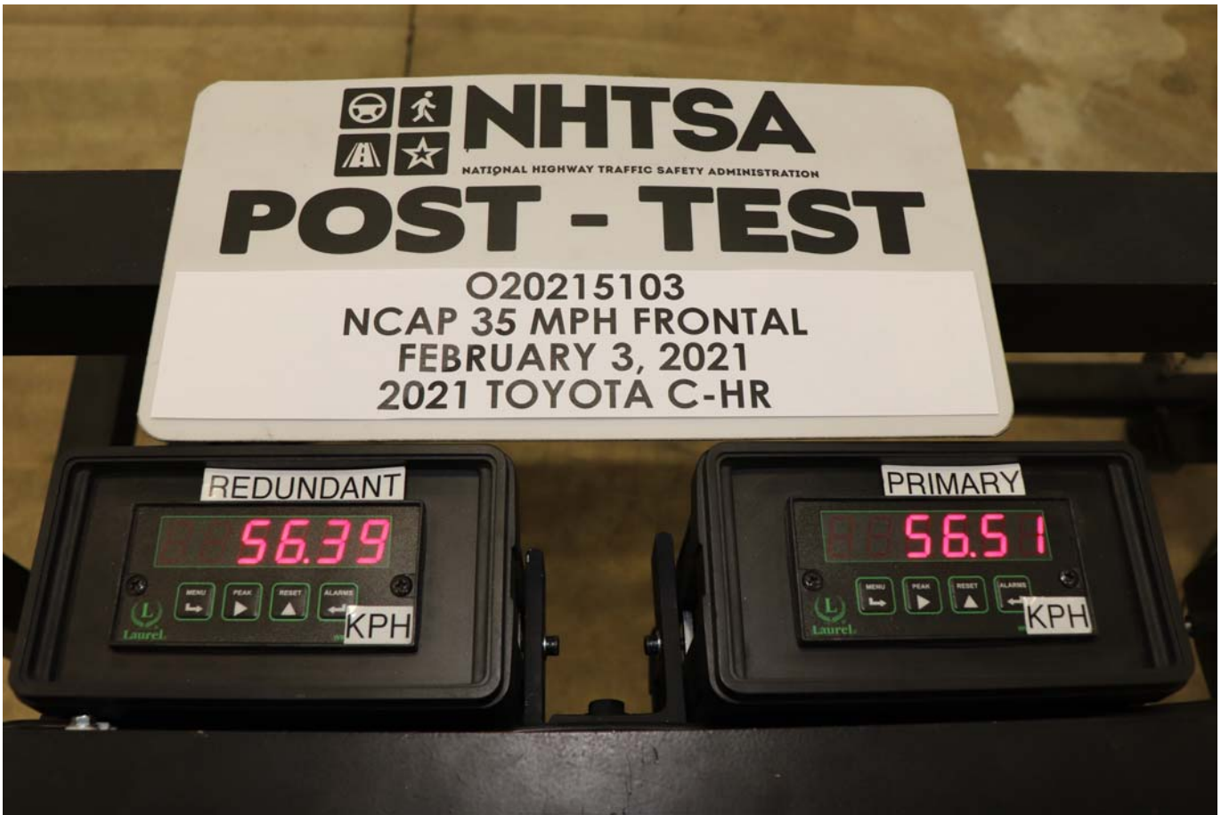
Photo No. 076 - Post-Test Speed Trap Read-Out
