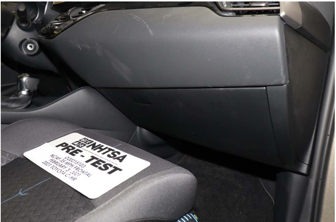
Photo No. 067 - Pre-Test Passenger Side Knee Bolster
