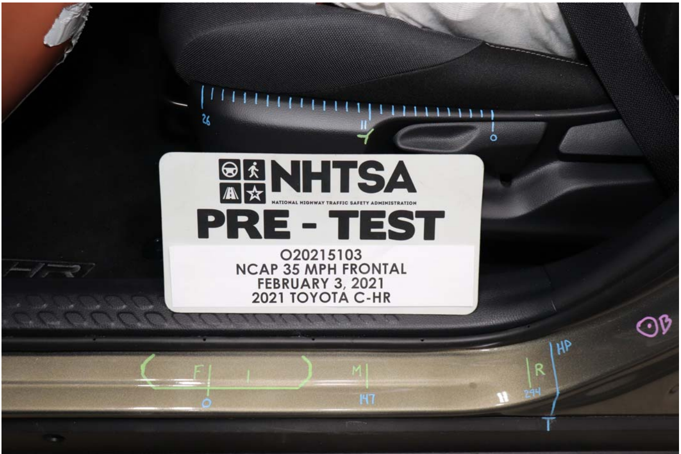
Photo No. 036 - Pre-Test Driver Seat Fore-Aft Markings
