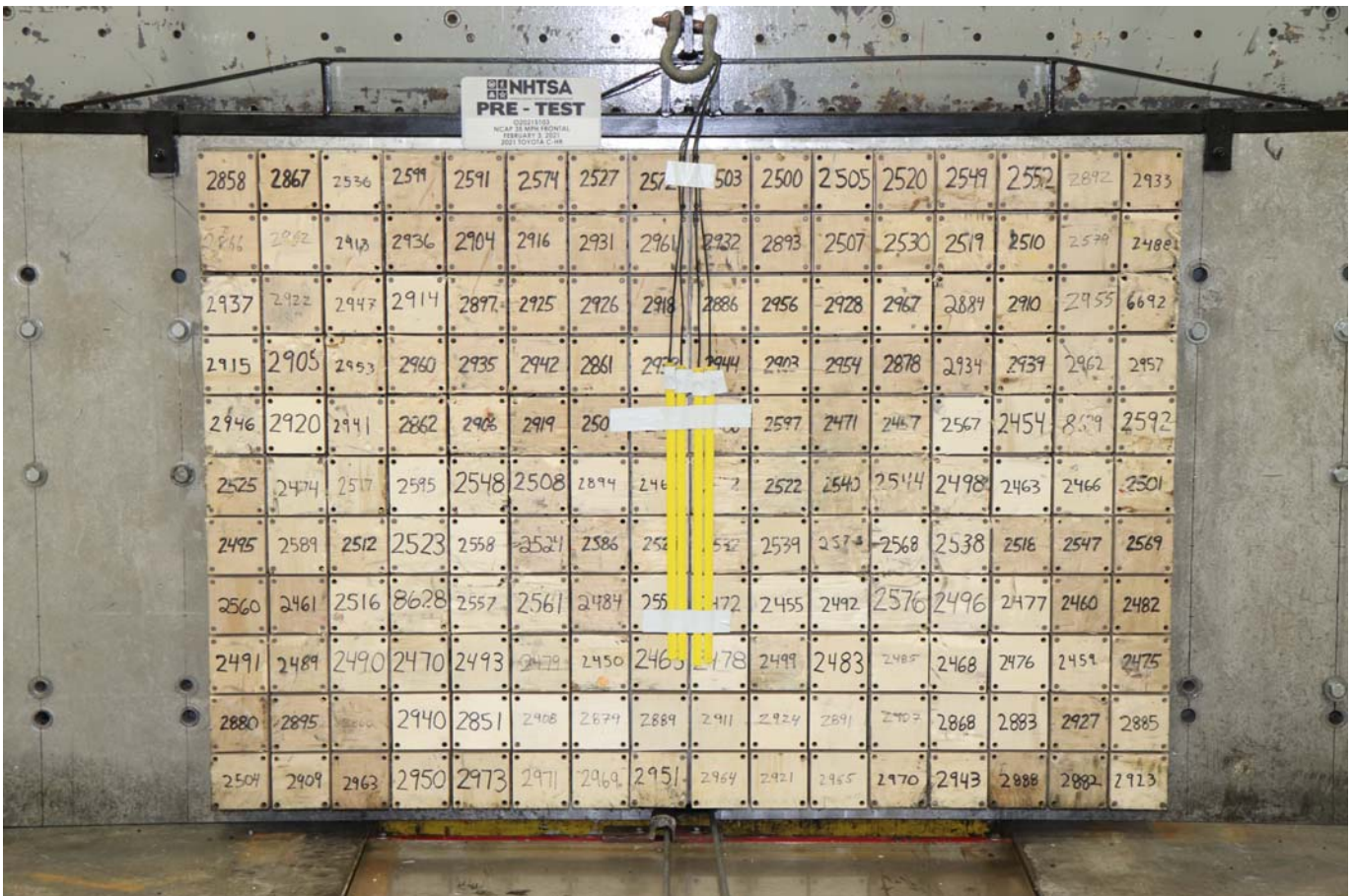
Photo No. 002 - Pre-Test Load Cell Wall
