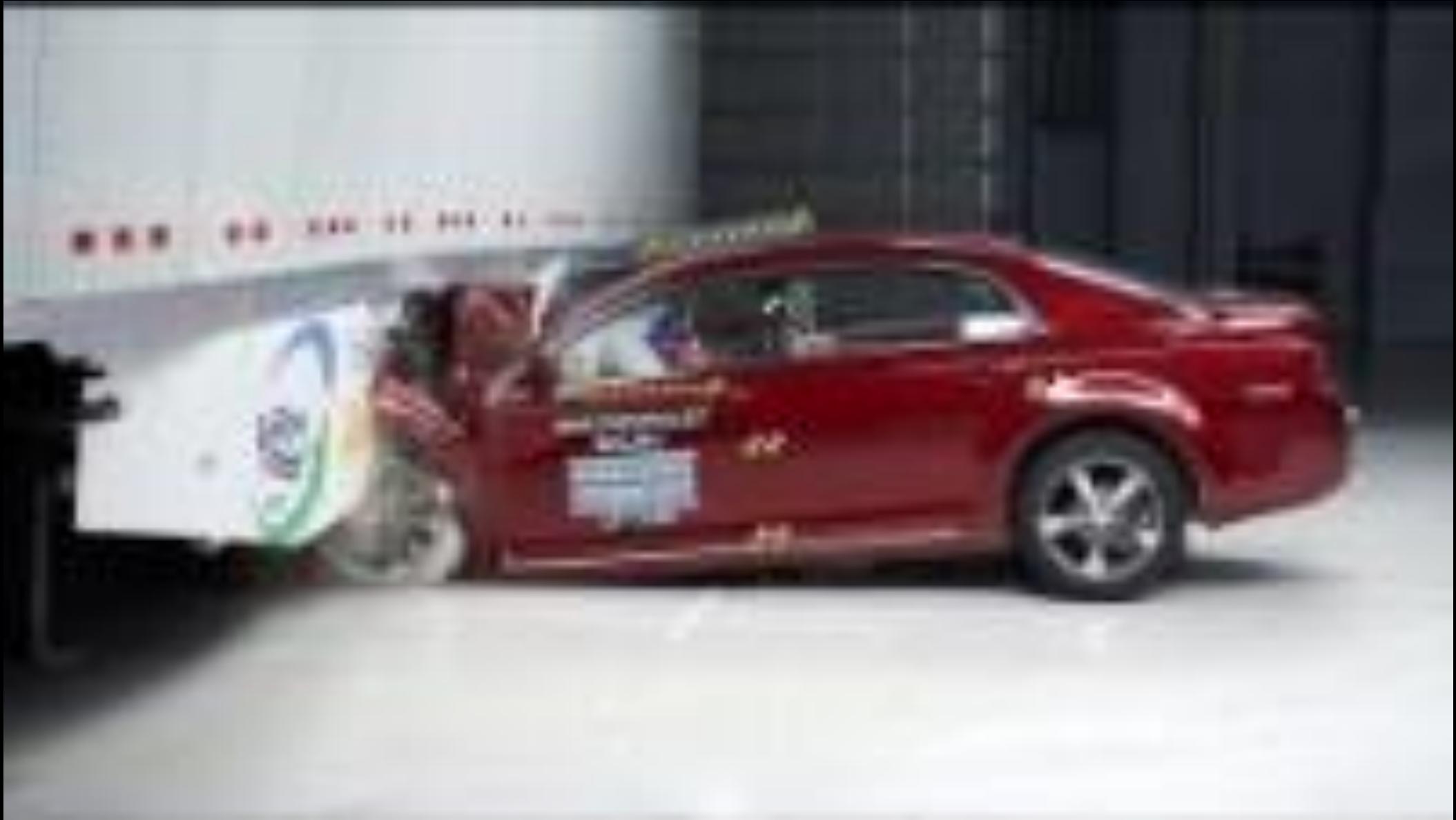
IIHS Side Guard Crash Test at 40 mph, August 29, 2017
