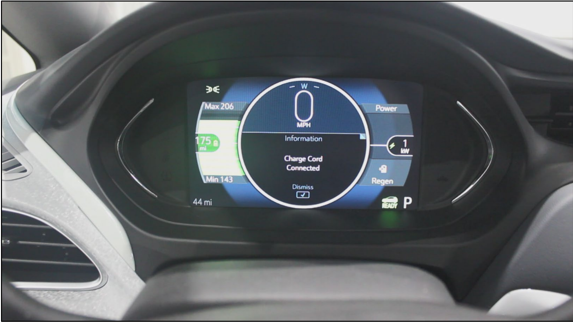
Figure 12: Signal to Driver When Selecting Active Drive Mode Possible While External Charging Is Active.
