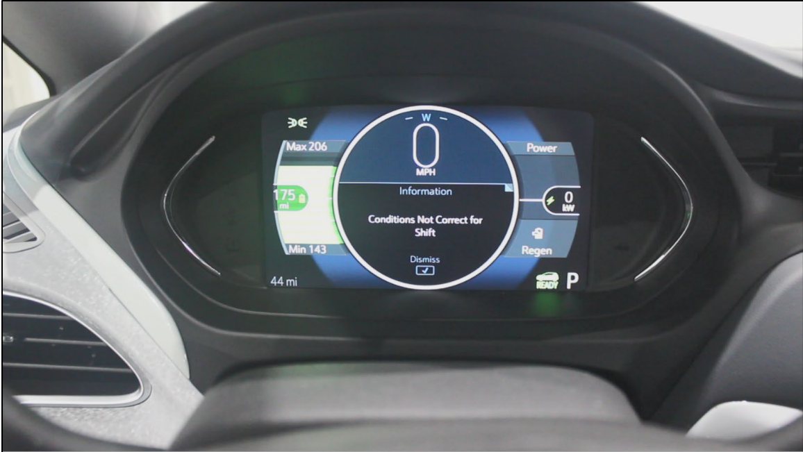
Figure 11: Momentary Signal to Driver When Selecting Active Drive Mode Possible While External Charging Is Active.
