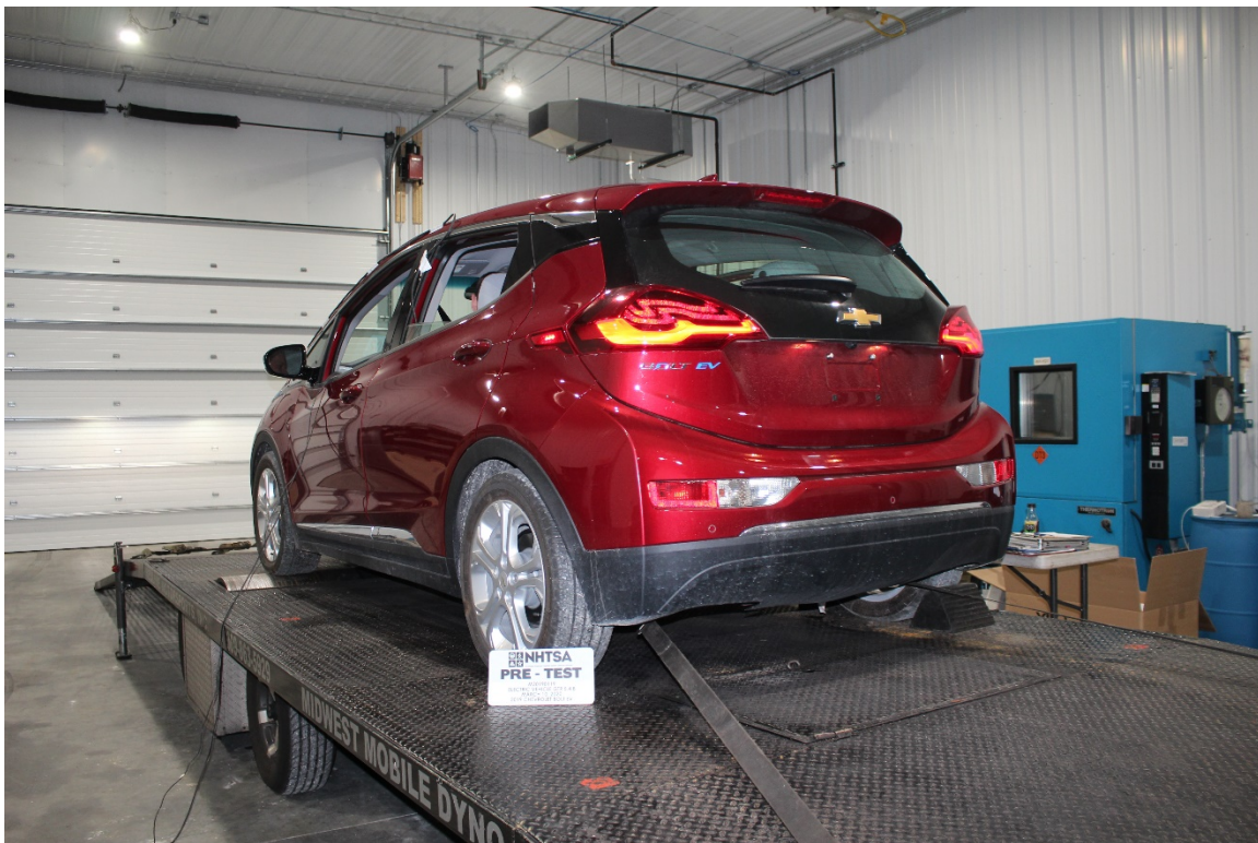
Figure 38: Vehicle Installed on Mobile Dynamometer
