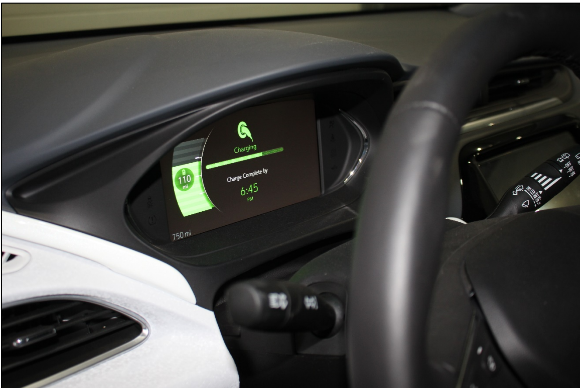
Figure 50: Over-Current Pre-Test Instrument Cluster Message
