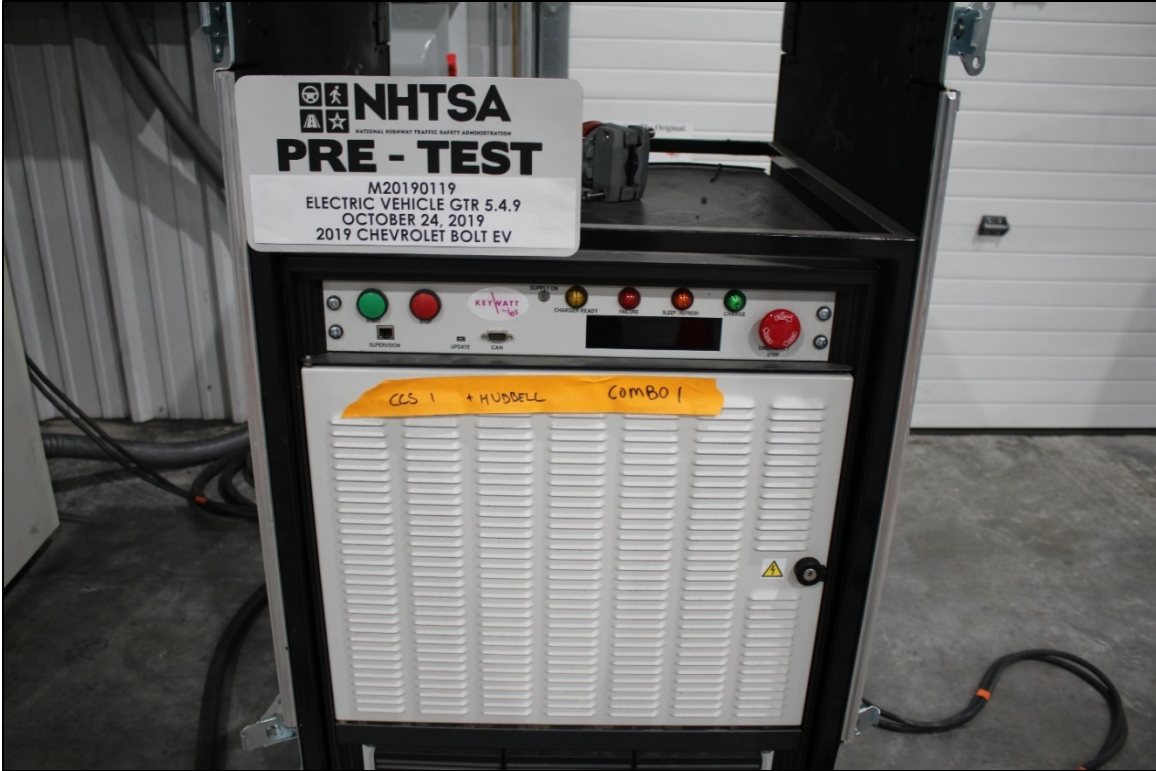
Figure 49: DC Fast Charger
