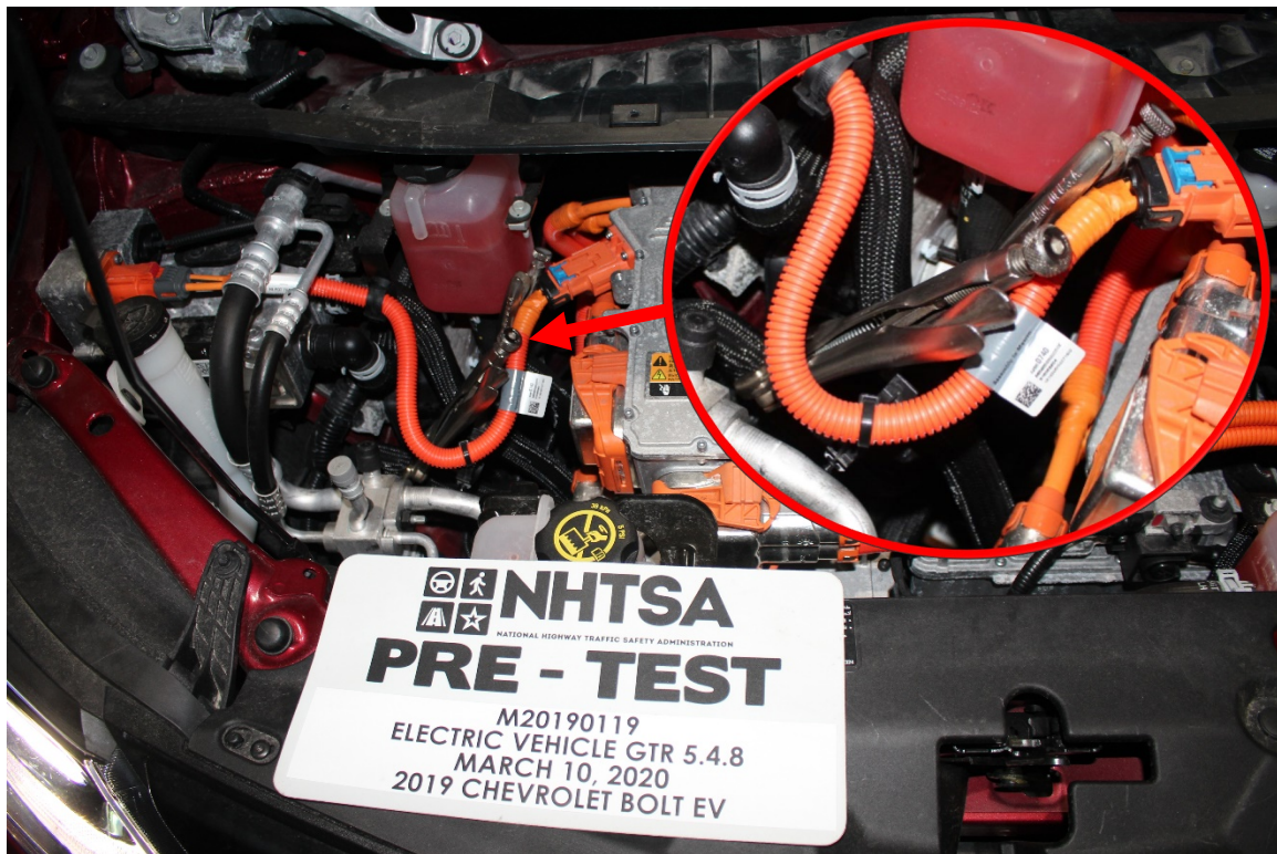
Figure 40: Over-Temperature Coolant Hose Crimps
