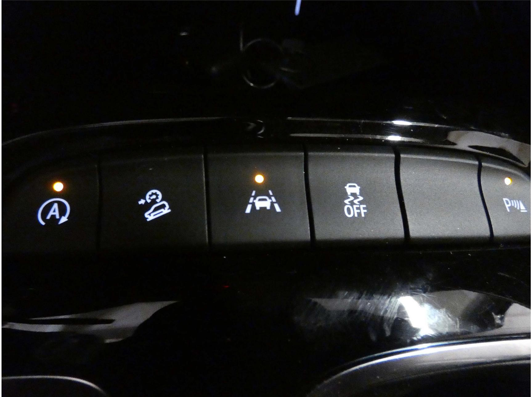
Figure A9. LDW On/Off Switch
