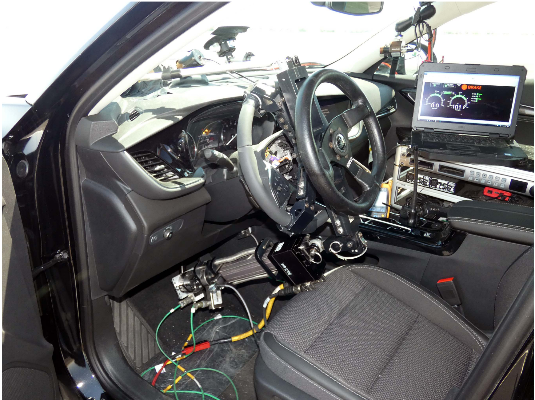
Figure A12. Computer and Brake Actuator Installed in Subject Vehicle
