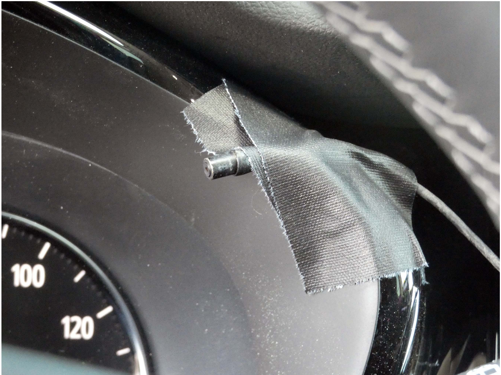
Figure A11. Sensor for Detecting Auditory Alerts A-13
