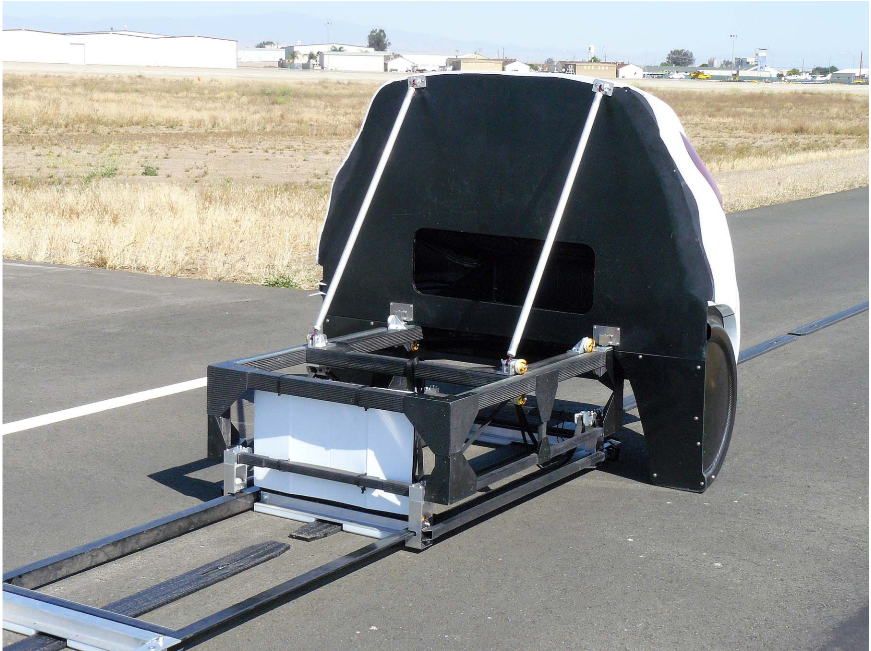
Figure A7. Load Frame/Slider of SSV
