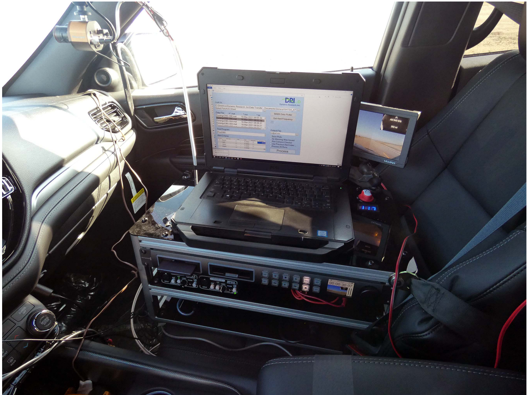
Figure A8. Computer Installed in Subject Vehicle
