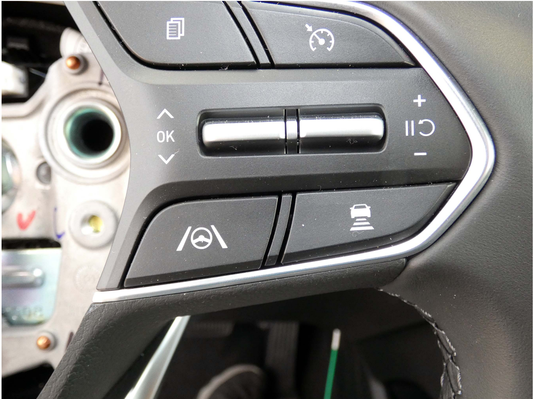
Figure A10. Buttons for Accessing System Setup Menus and Lane Driving Assist On/Off
