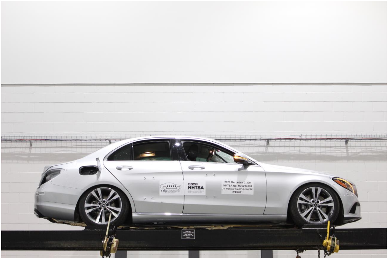
Figure A-69: FMVSS No. 301 Static Rollover 360 Degrees
