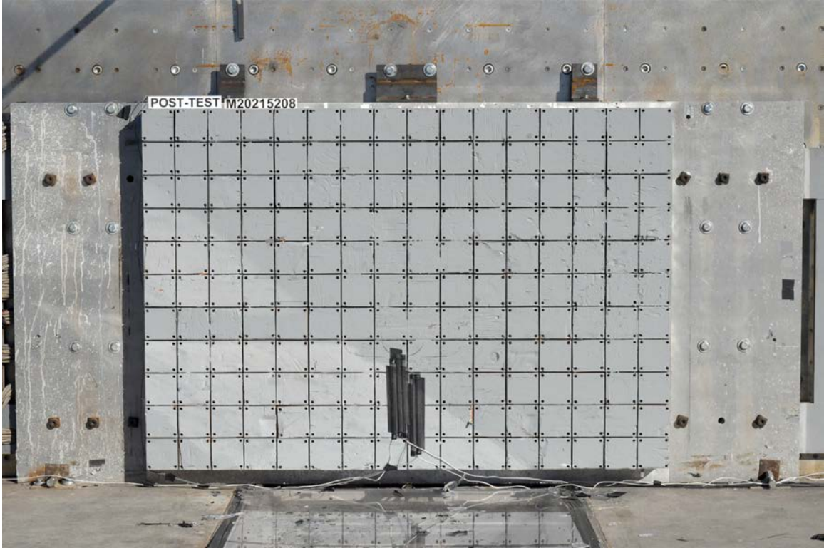
FIGURE 3. Post-Test Load Cell Wall
