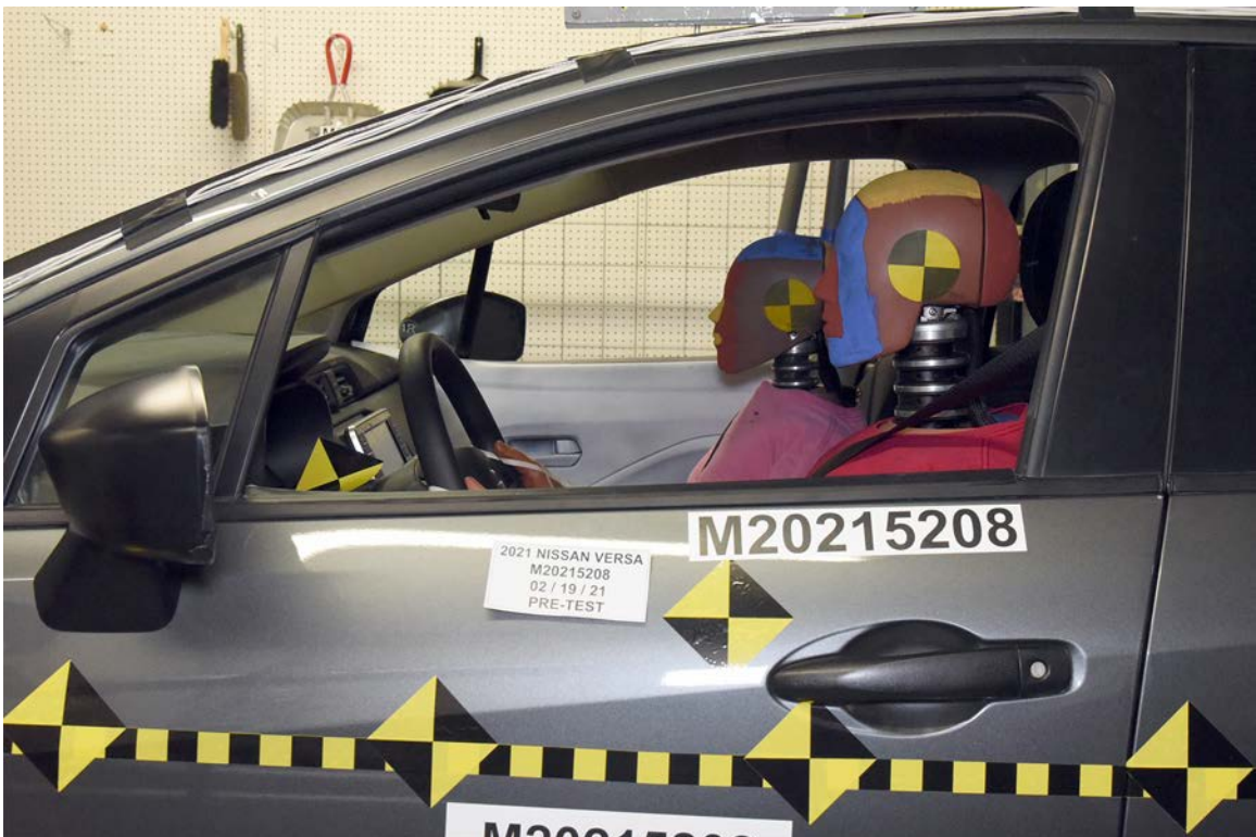
FIGURE 32. Pre-Test Driver Dummy Window View
