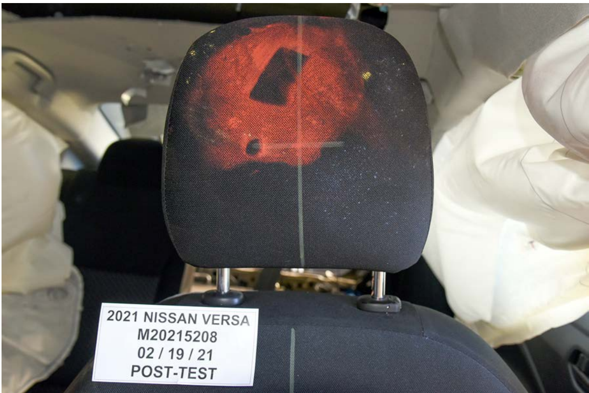
FIGURE 50. Post-Test Driver Dummy Contact with Headrest
