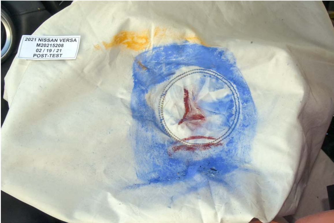
FIGURE 49. Post-Test Driver Dummy Contact with Airbag
