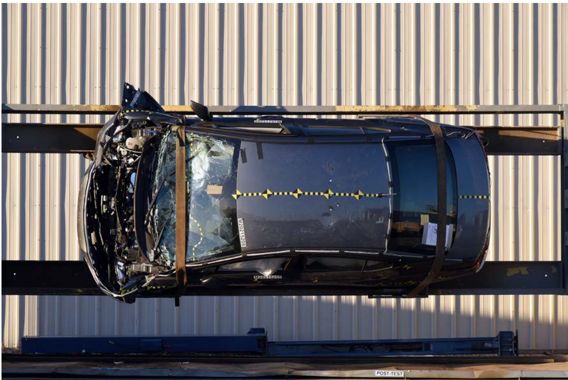
FIGURE 78. Vehicle at 90° on Static Rollover Device
