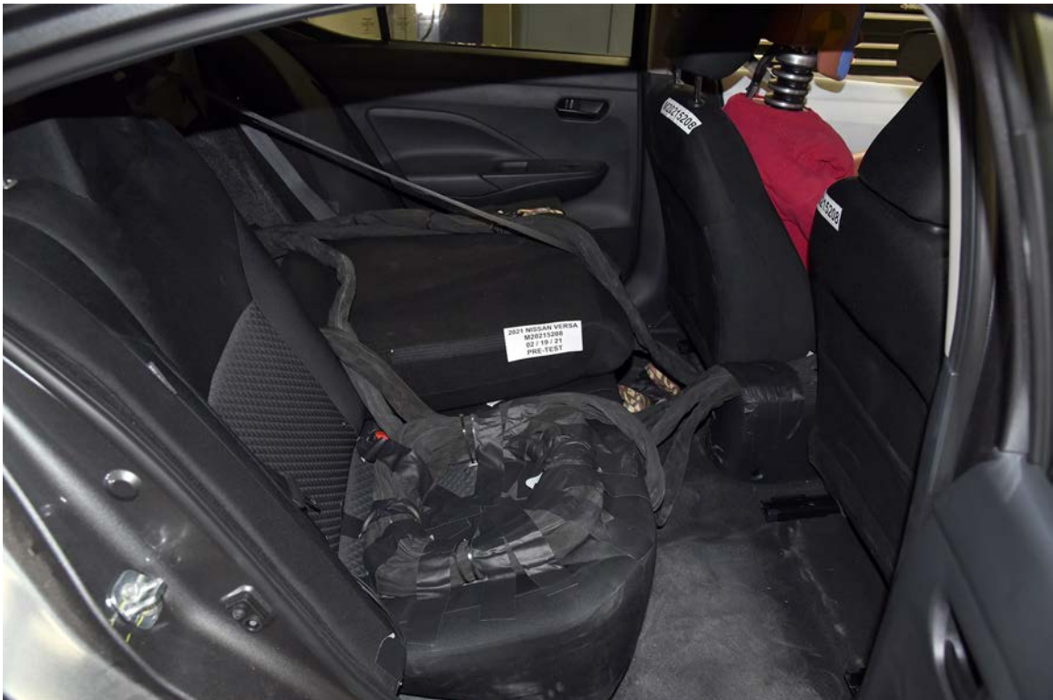
FIGURE 28. Pre-Test Dummy Cable Routing
