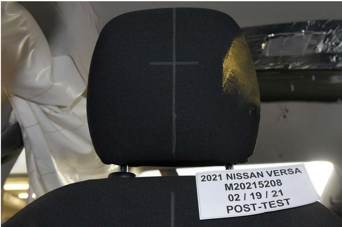
FIGURE 73. Post-Test Passenger Dummy Contact with Headrest
