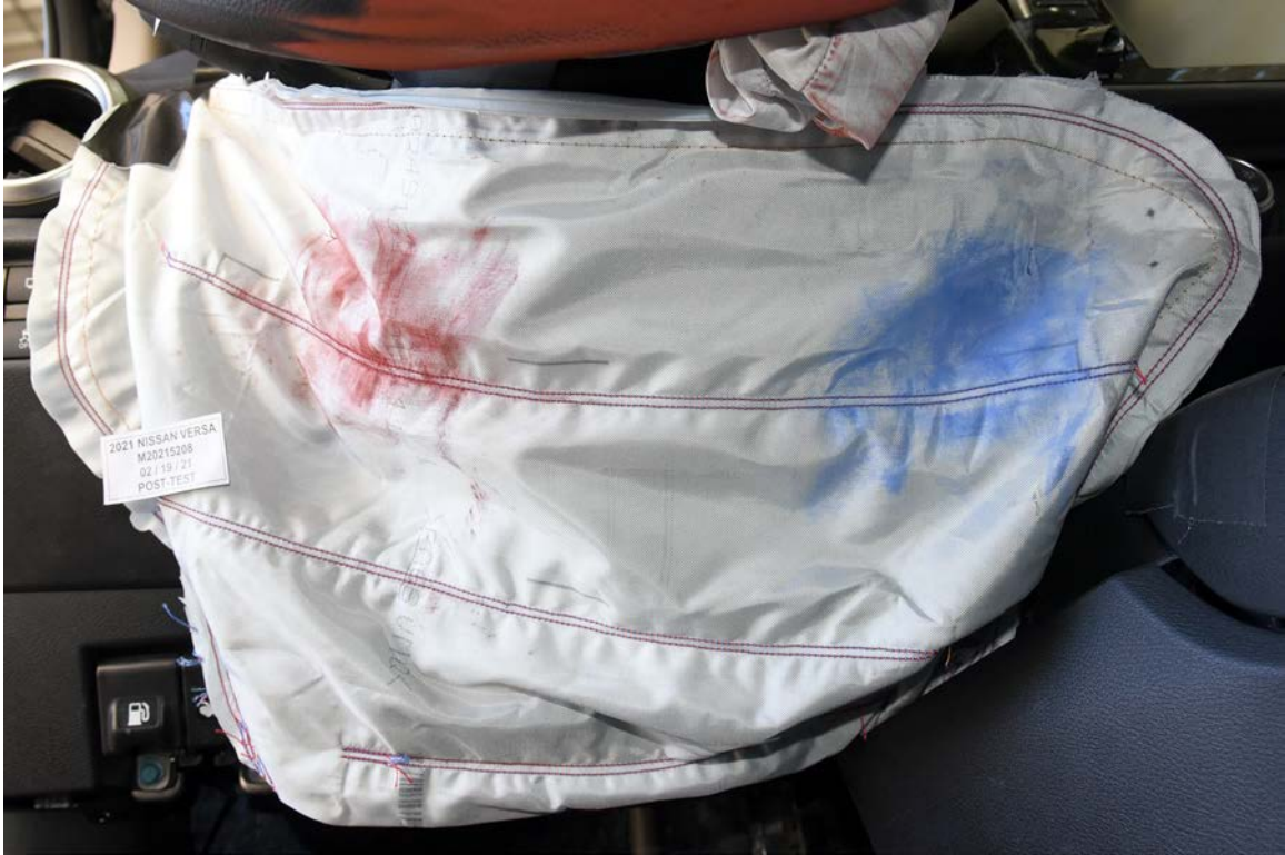
FIGURE 50a. Post-Test Driver Dummy Contact with Knee Airbag
