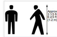
Fig 1: Pedestrians must be in the range of 1-2 m tall to be detectable
