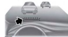
Fig.2 Head-up display warning on detection of vehicle, object or pedestrian
