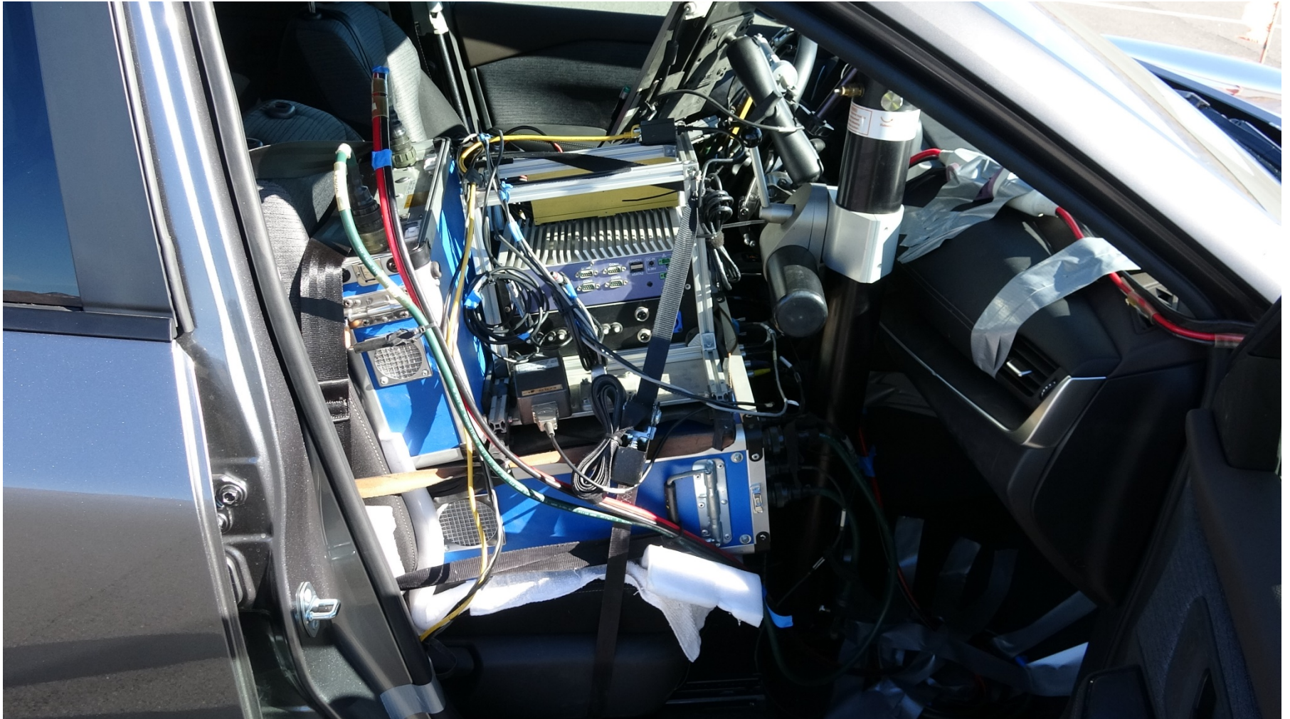
Figure A8. Instrumentation in Test Vehicle
