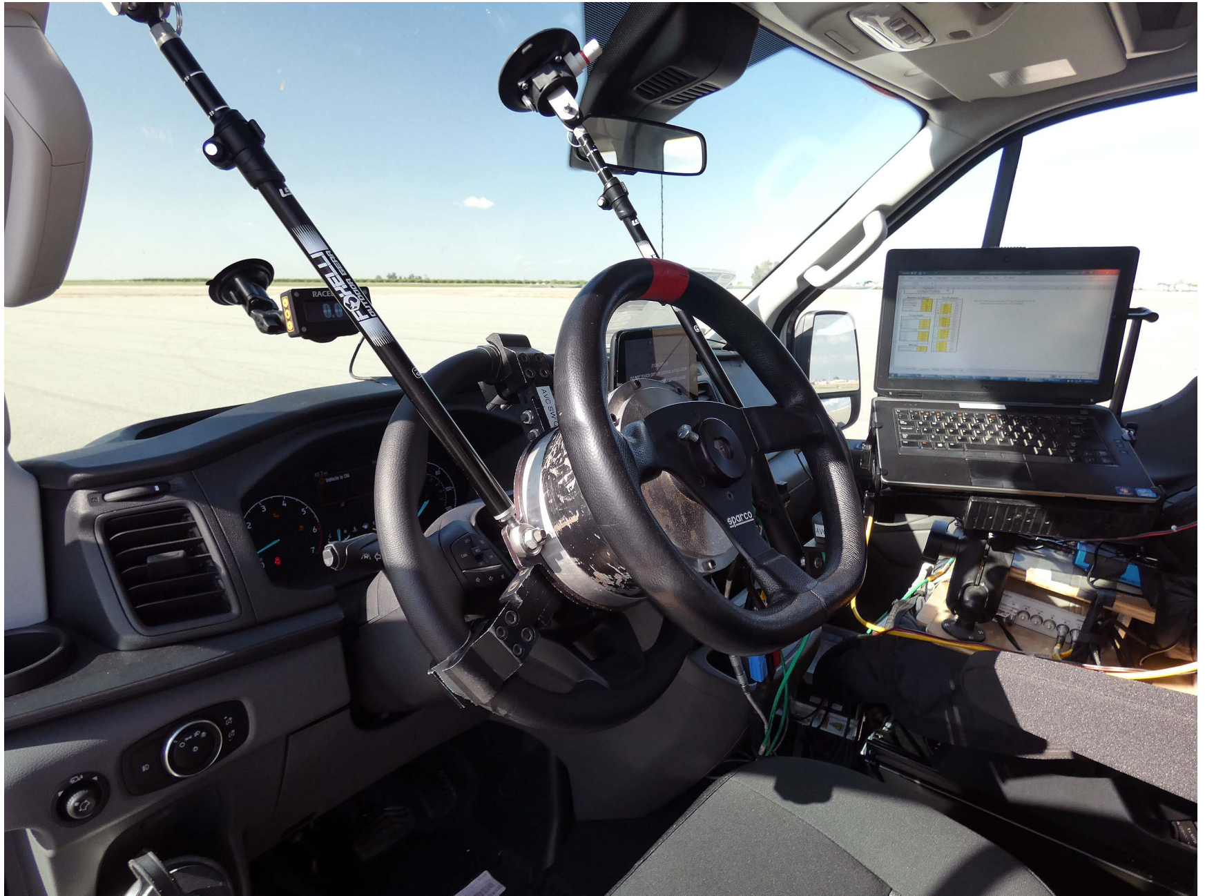
Figure A9. Steering Controller and Computer
