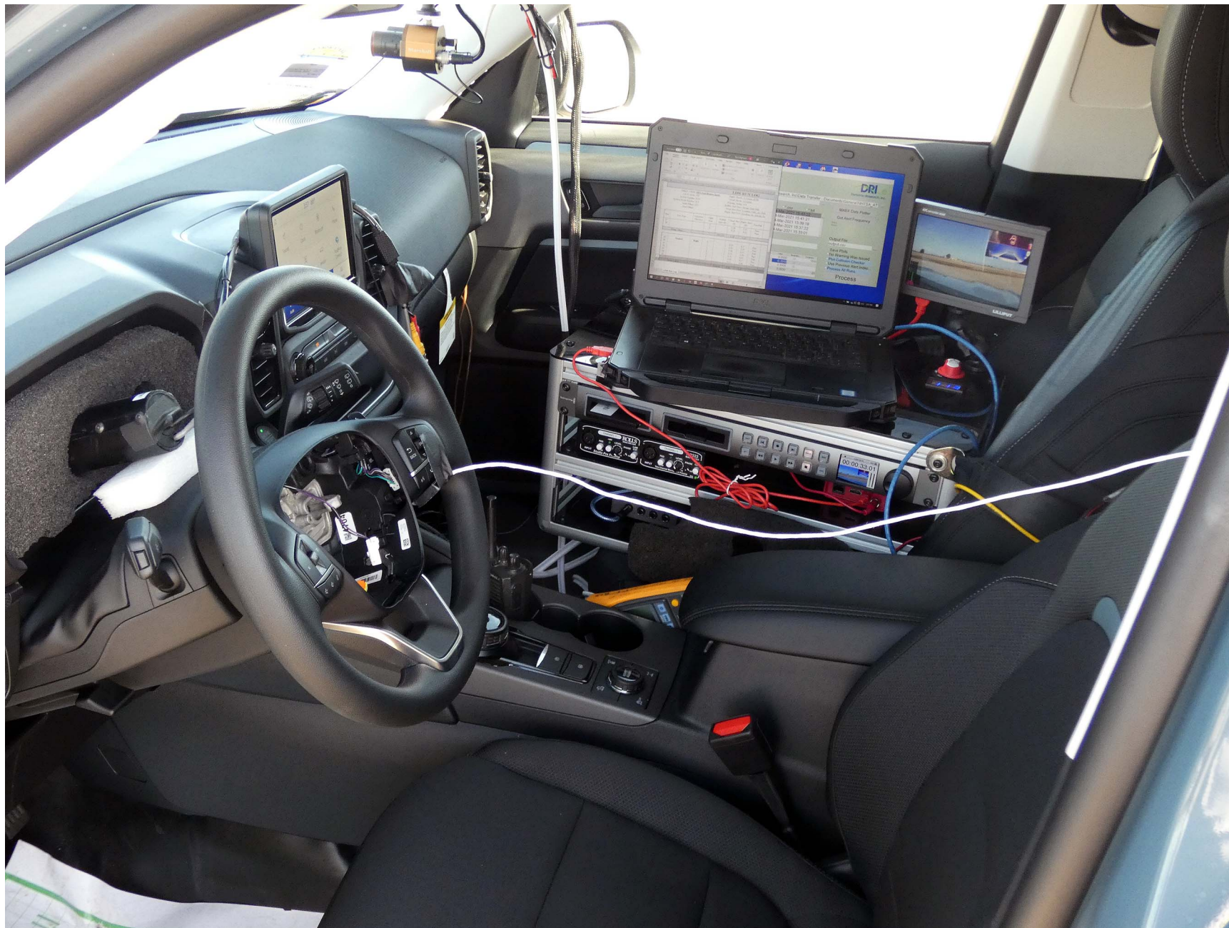
Figure A8. Computer Installed in Subject Vehicle
