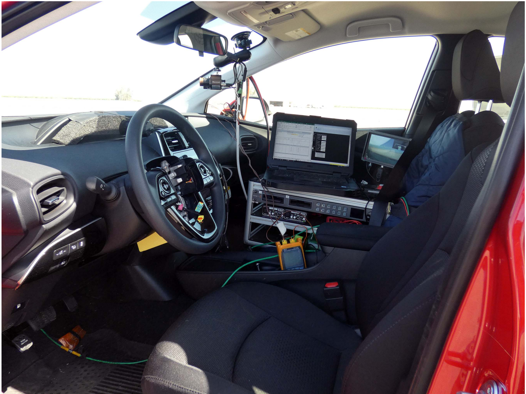
Figure A12. Computer Installed in Subject Vehicle
