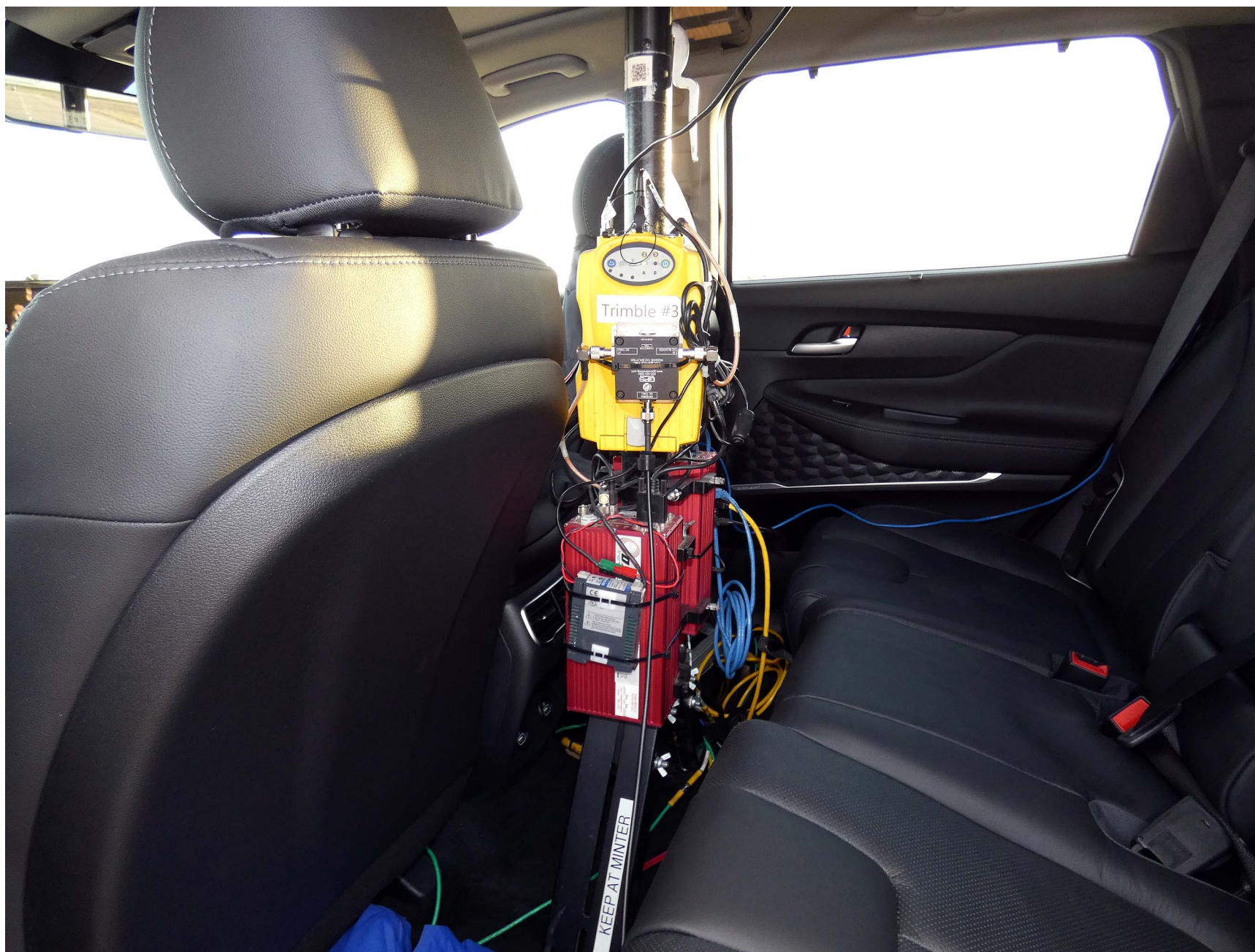
Figure A10. DGPS and Inertial Measurement Unit Installed in Subject Vehicle
