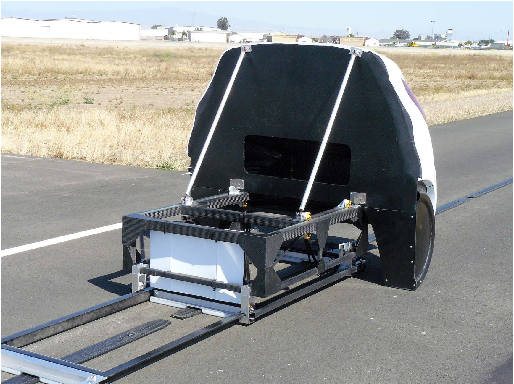
Figure A7. Load Frame/Slider of SSV
