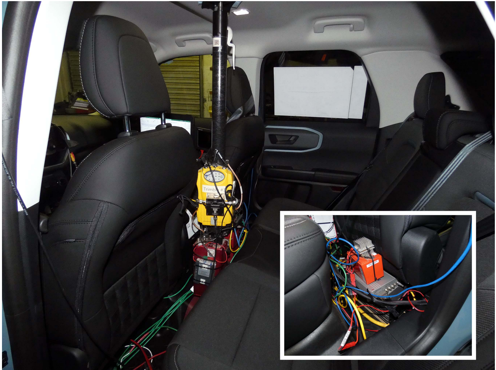
Figure A8. DGPS and Inertial Measurement Unit Installed in Subject Vehicle
