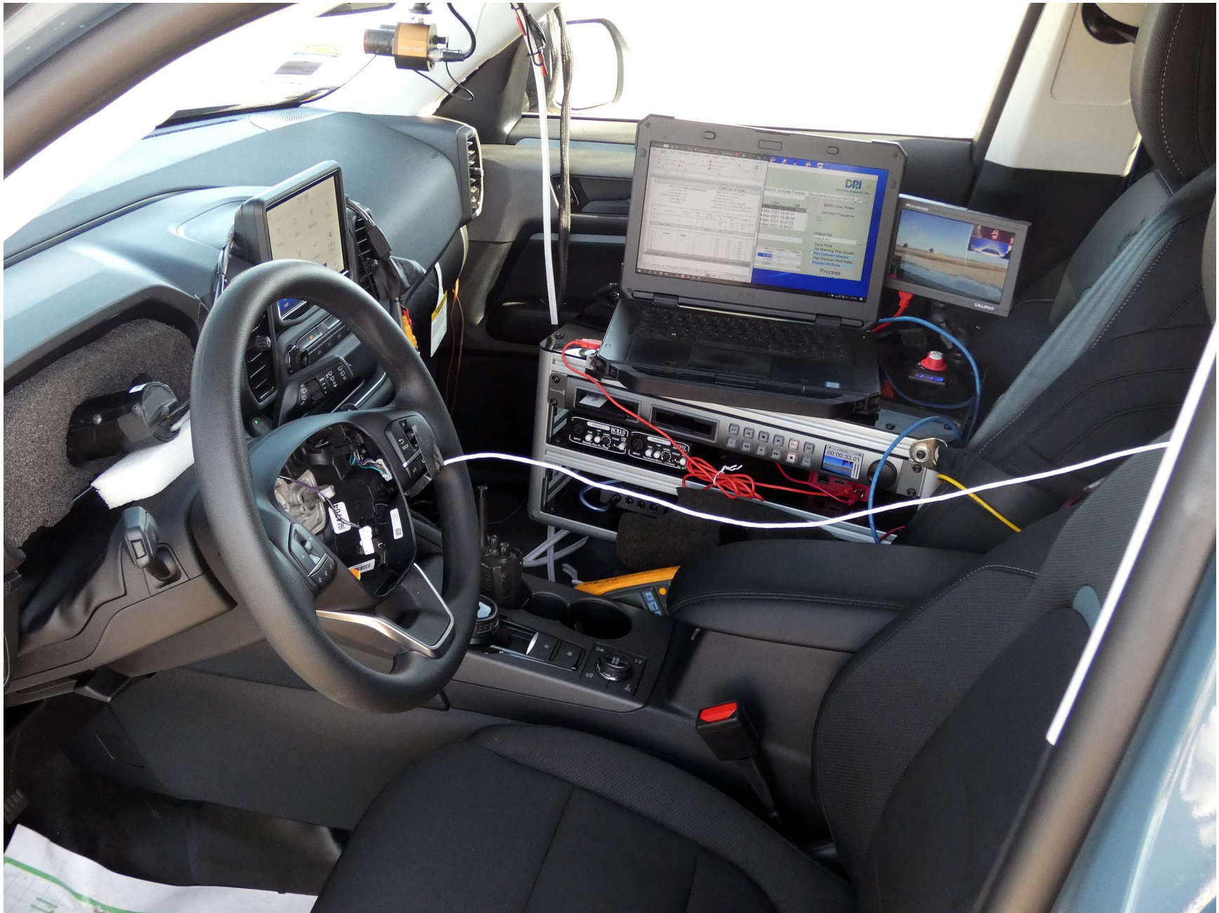
Figure A10. Computer Installed in Subject Vehicle
