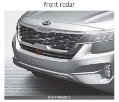
Dirt, snow, or foreign substances on the sensor cover or sensor may adversely affect the sensing performance of the sensor.
