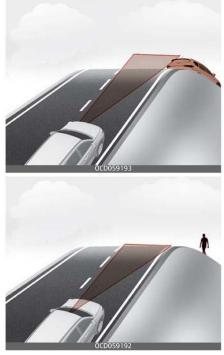
The performance of FCA decreases while driving upward or downward on a slope, not recognizing the vehicle in front in the same lane. It may unnecessarily produce the warning message and the warning alarm, or it may not produce the warning message and the warning alarm at all.
