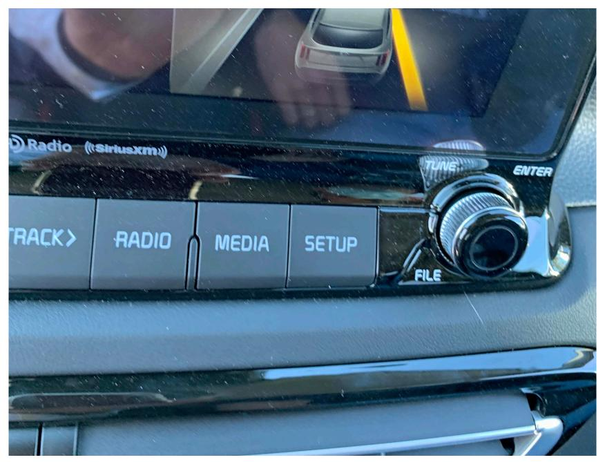
Figure A16. Button for Accessing System Setup Menus
