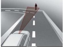
In this case, the system may unnecessarily alarm the driver and apply the brake.
