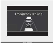
This warning message appears on the LCD display with a warning chime. Additionally, some vehicle system intervention occurs by the engine management system to help decelerate the vehicle. The brake control is maximized just before a collision, reducing impact when it strikes a forward vehicle.
