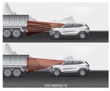
If the vehicle in front of you has cargo that extends rearward from the cab, or when the vehicle in front of you has higher ground clearance,
