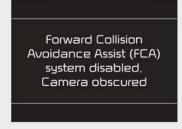
When the camera is blocked with dirt, snow, or debris, FCA system operation may not be able to detect other vehicles.
