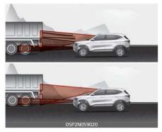
If the vehicle in front of you has cargo that extends rearward from the cab, or when the vehicle in front of you has higher ground clearance, additional special attention is required. FCA system may not be able to detect the cargo extending from the vehicle. In these instances, you must maintain a safe braking distance from the rearmost object, and if necessary, depress the brake pedal to reduce your driving speed in order to maintain distance.
