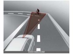
In this case, the system may unnecessarily alarm the driver and apply the brake.
