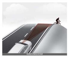
The performance of FCA decreases while driving upward or downward on a slope, as it may not recognize the vehicle in front in the same lane. It may unnecessarily produce the warning message and the warning alarm, or it may not produce the warning message and the warning alarm at all.
