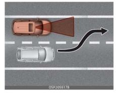
When a vehicle changes lanes in front of you, FCA system may not immediately detect the vehicle, especially if the vehicle changes lanes abruptly. In this case, you must maintain a safe braking distance, and if necessary, depress the brake pedal to reduce your driving speed in order to maintain a safe distance.
