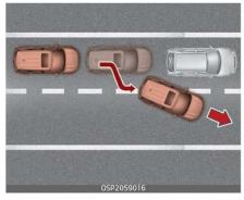
When driving in stop-and-go traffic, and a stopped vehicle in front of you merges out of the lane, FCA system may not immediately detect the new vehicle that is now in front of
