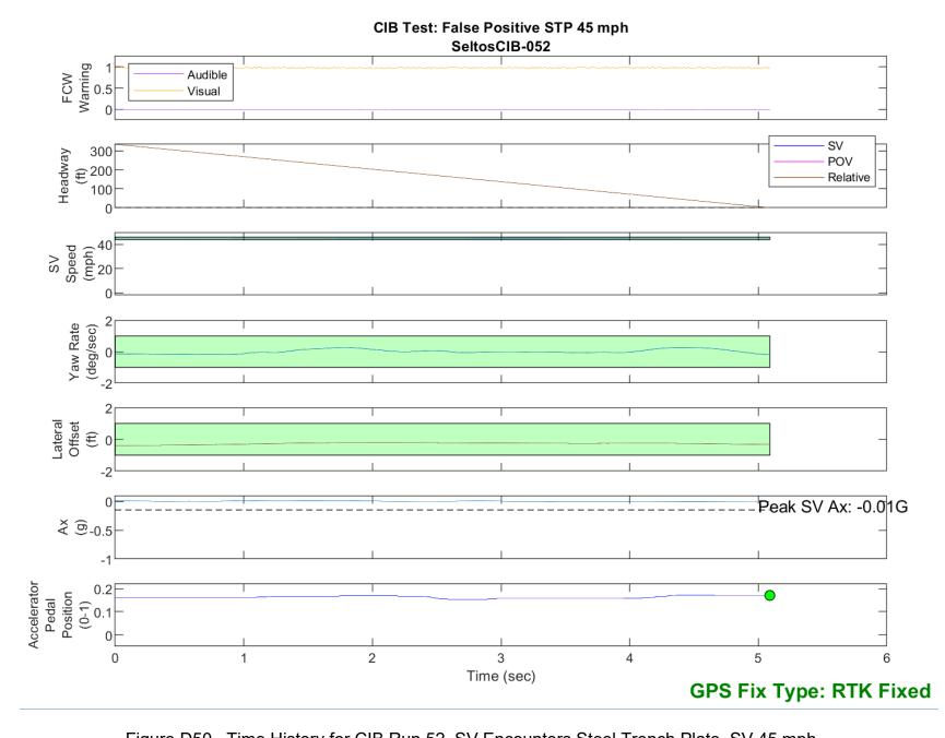
Figure D50. Time History for CIB Run 52, SV Encounters Steel Trench Plate, SV 45 mph
