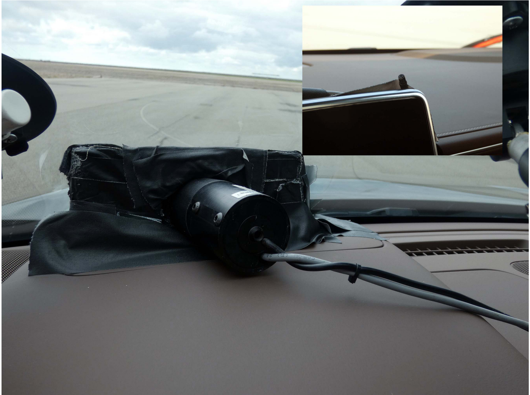
Figure A7. Sensors for Detecting Visual and Auditory Alerts
