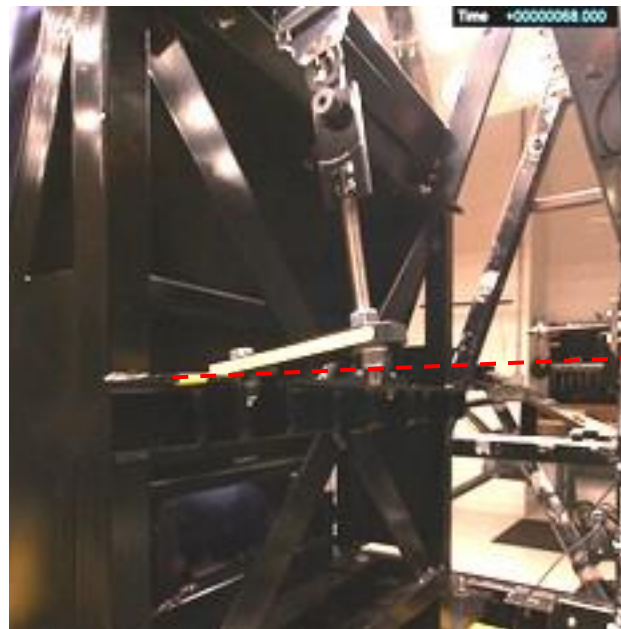
Figure 4. Still Image from High Speed Video Showing Upward Flexion of the Rear Shelf Mount (Original Plane of the Rear Locking Belt Mounting Bar Assembly Shown as a Dashed Red Line).
