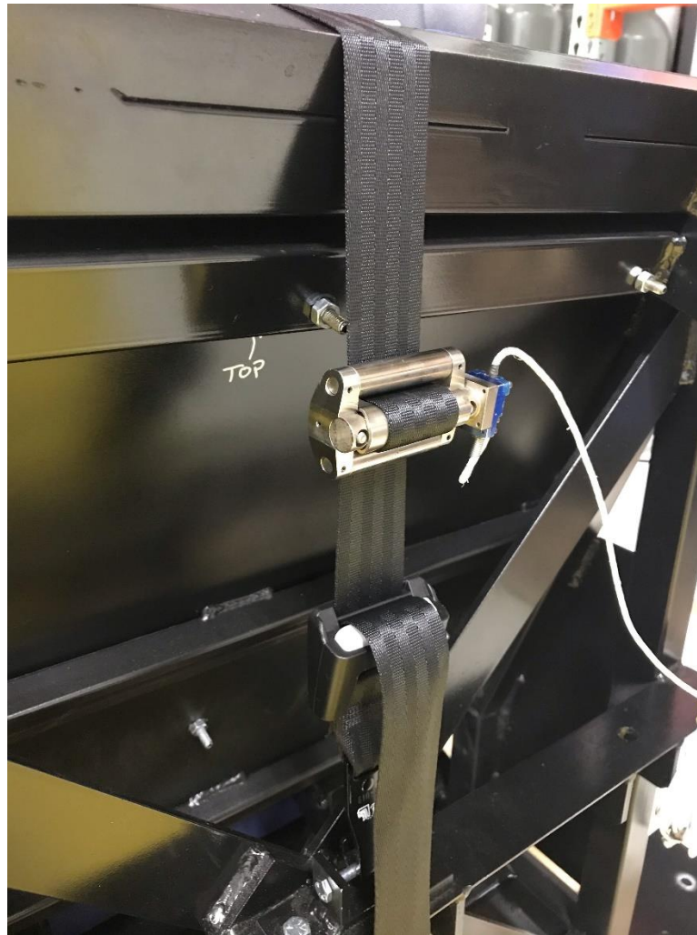
Figure 14. Recommended Load Cell Location on Tether for Pre-Test Tension Measurement.
