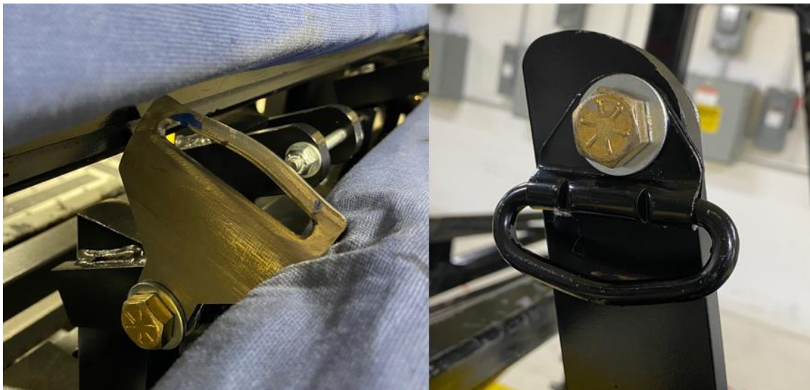
Figure 7. Deformation of the Inboard Lap Belt Anchor (left) and the D-Ring (right).
