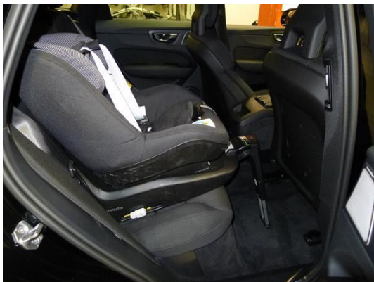
Figure 3a. A convertible CRS with support leg in forward-facing mode; a Maxi Cosi 2way Pearl with 2wayFix base in a Volvo car.
