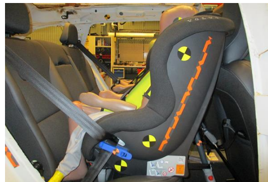
Figure 3b. Rearward facing child seat with support leg, Q6 dummy in a Volvo rearward facing child seat in a Volvo car.
