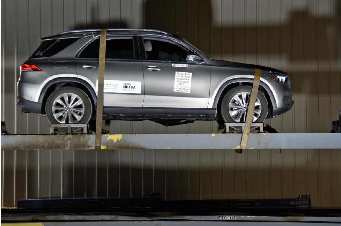
FIGURE 65. FMVSS No. 301 Static Rollover 0 Degrees
