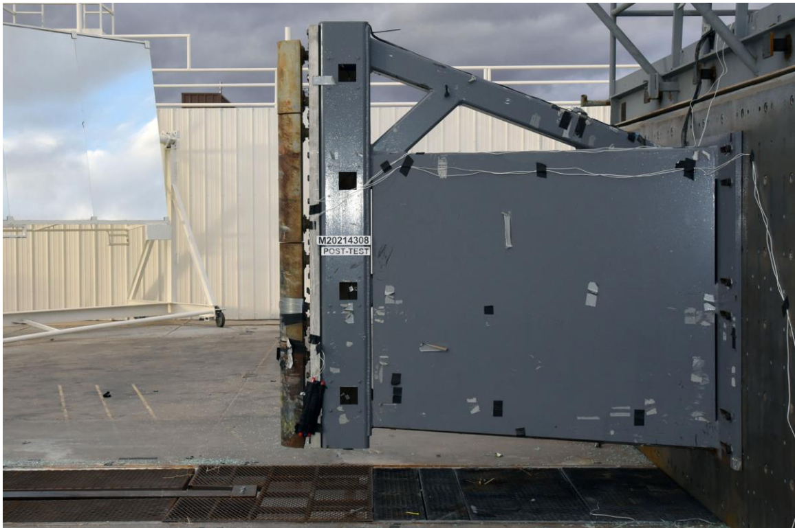
FIGURE 62. Post-Test Pole Barrier Side View
