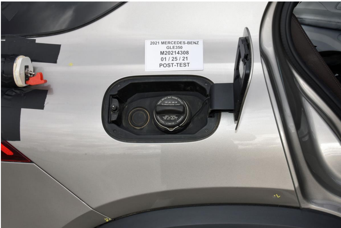
FIGURE 56. Post-Test View of Fuel Filler Cap or Fuel Filler Neck
