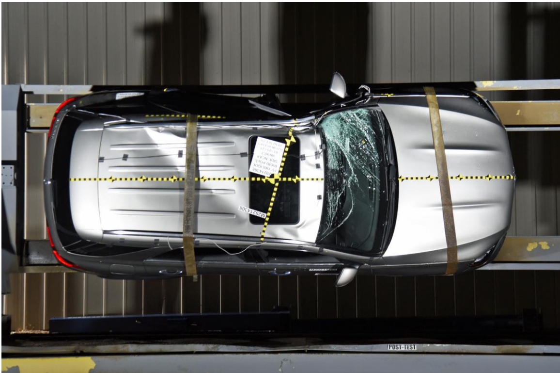
FIGURE 66. FMVSS No. 301 Static Rollover 90 Degrees
