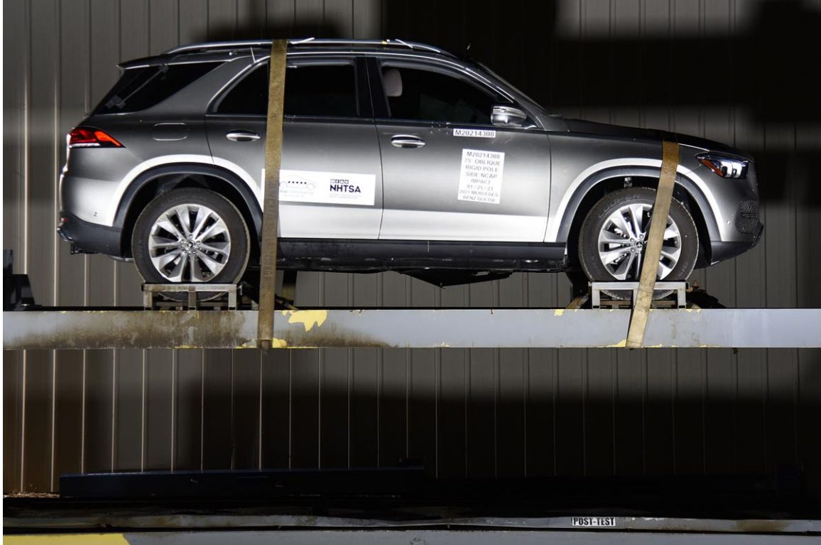
FIGURE 69. FMVSS No. 301 Static Rollover 360 Degrees
