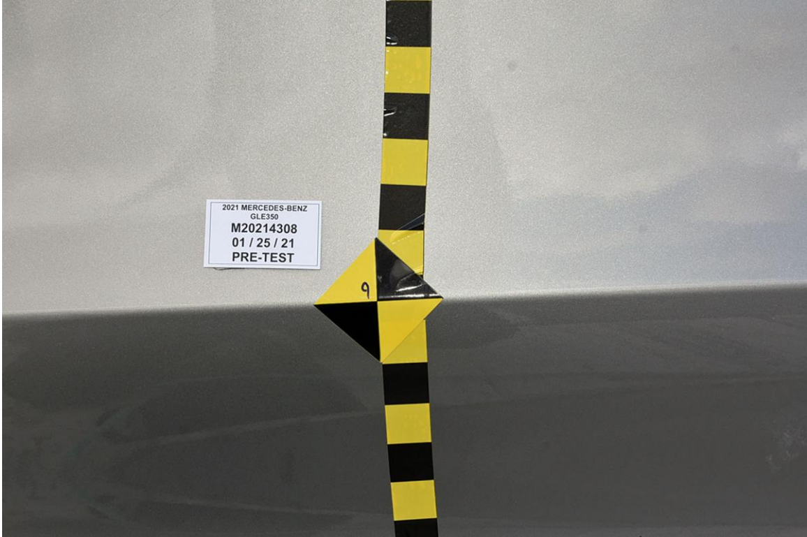
FIGURE 19. Pre-Test Close-Up View of Impact Point Target
