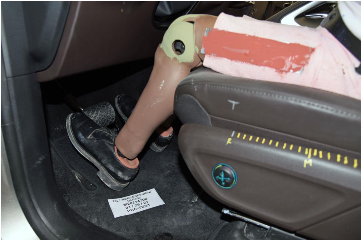
FIGURE 32. Pre-Test Placement of Dummy's Feet
