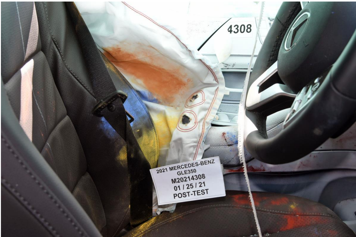
FIGURE 48. Post-Test Dummy Close-Up Torso Contact With Vehicle Interior View
