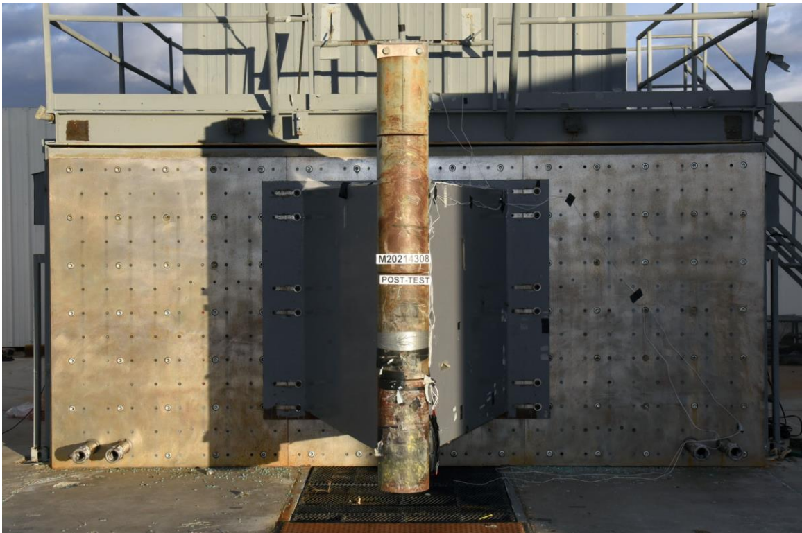
FIGURE 60. Post-Test Pole Barrier Front View
