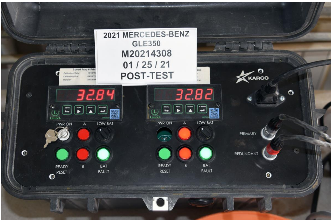
FIGURE 64. Post-Test Primary and Redundant Speed Trap Read-Out
