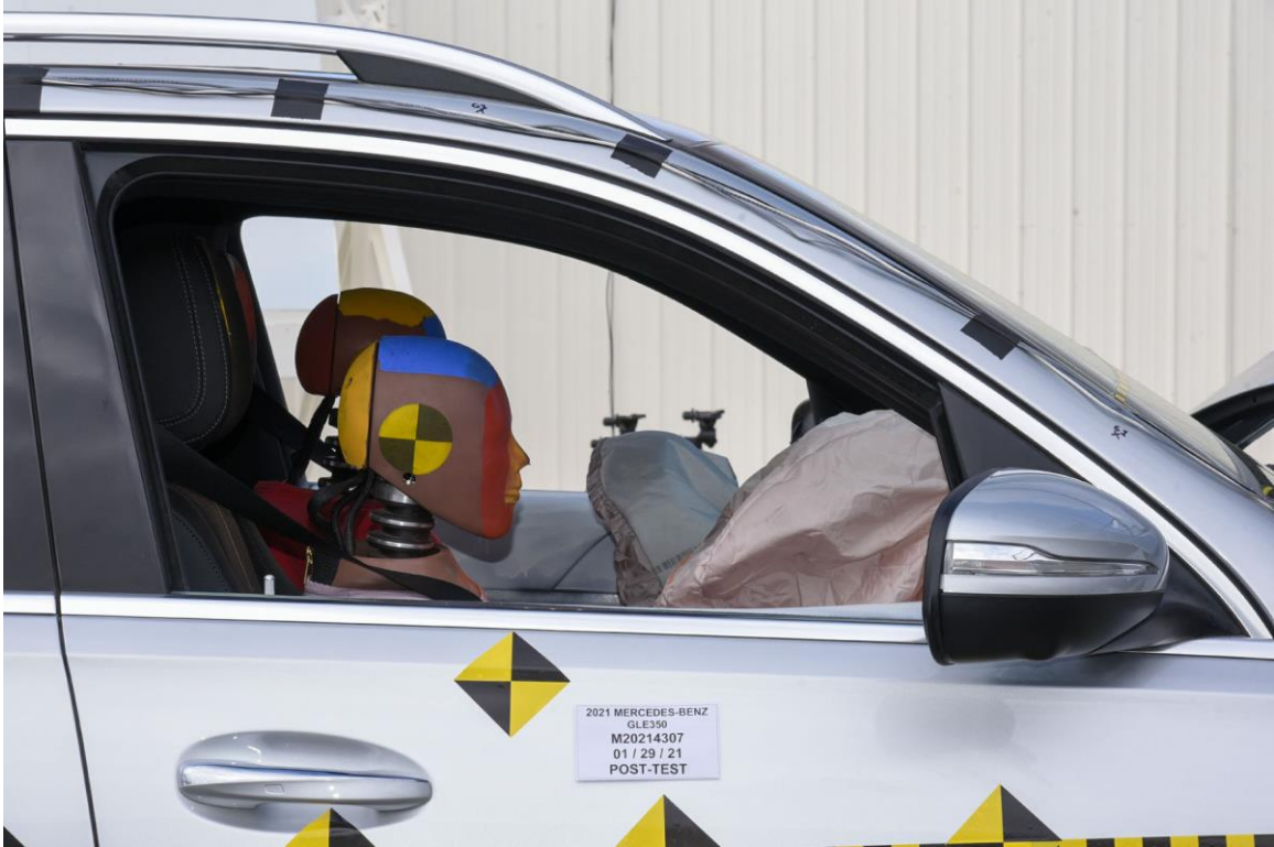
FIGURE 56. Post-Test Passenger Dummy Window View
