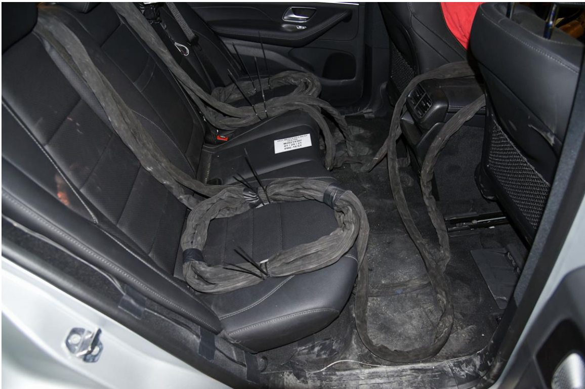
FIGURE 28. Pre-Test Dummy Cable Routing
