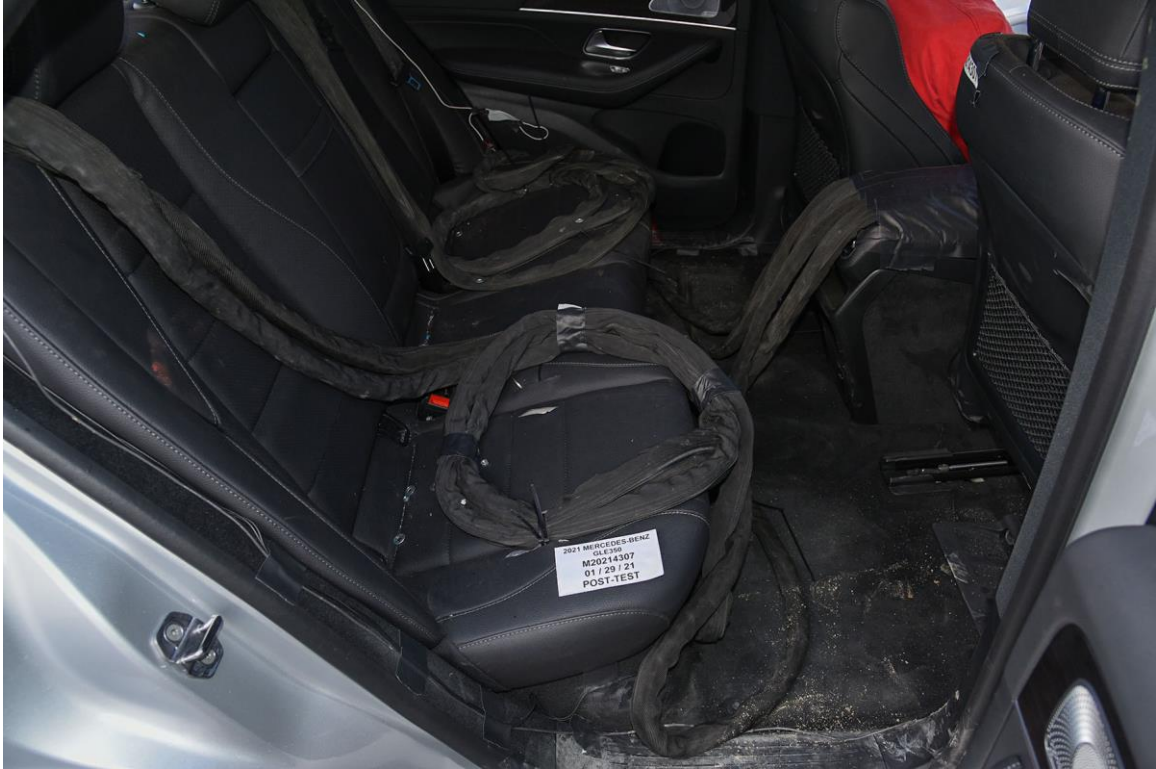
FIGURE 29. Post-Test Dummy Cable Routing
