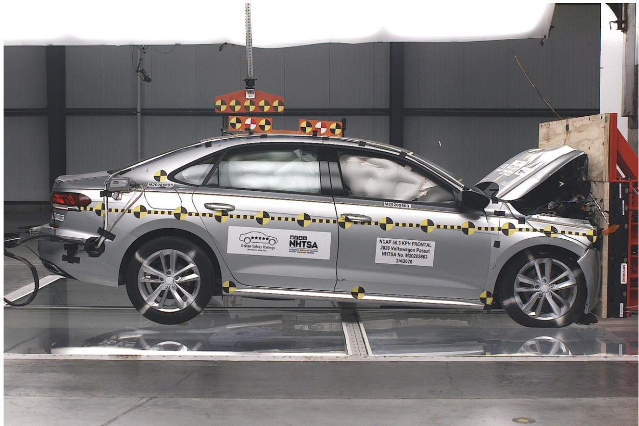
Figure A-82: 2020 Volkswagen Passat Frontal Impact Event
