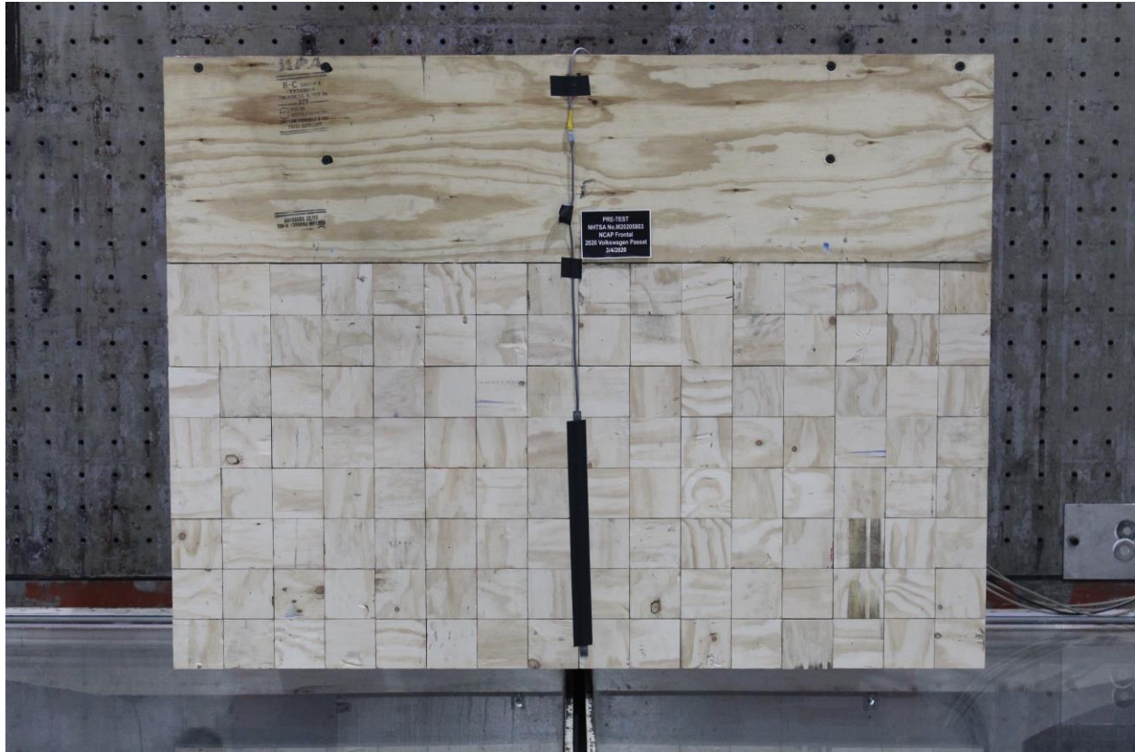
Figure A-2: Pre-Test Load Cell Wall
