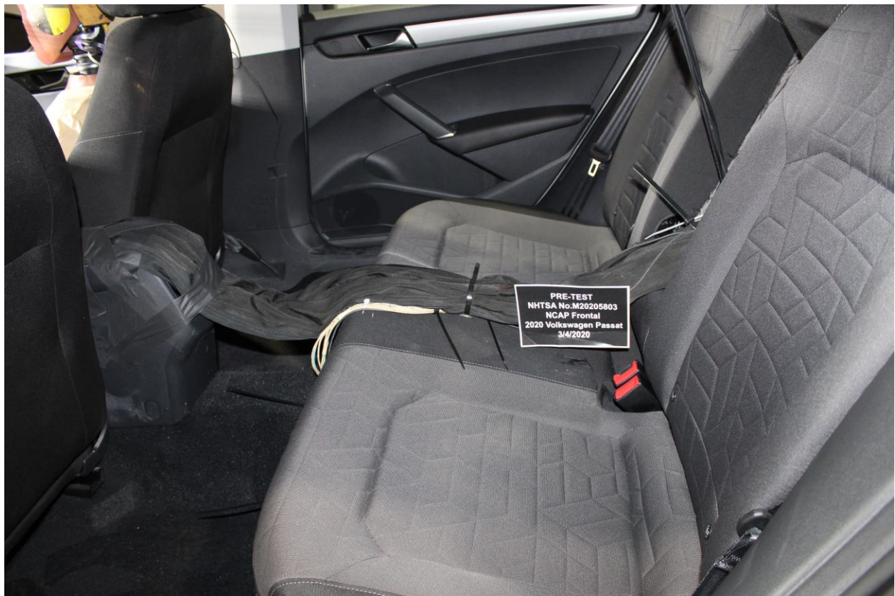
Figure A-28: Pre-Test Dummy Cable Routing
