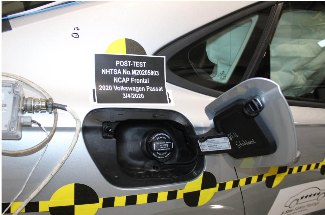
Figure A-23: Post-Test Fuel Filler Cap View
