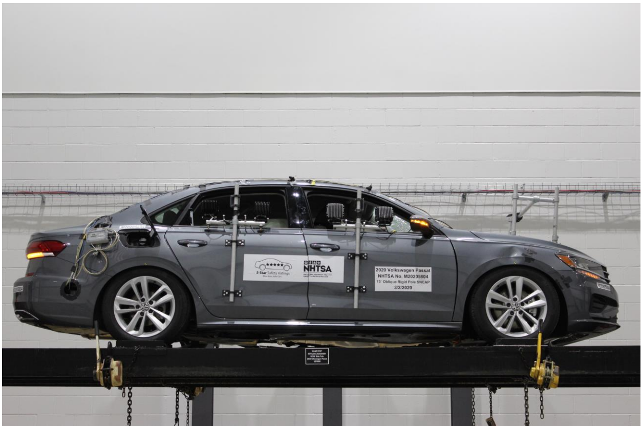
Figure A-67: FMVSS No. 301 Static Rollover 360 Degrees
