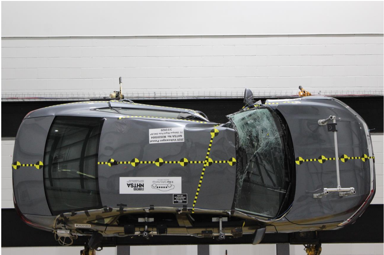
Figure A-64: FMVSS No. 301 Static Rollover 90 Degrees
