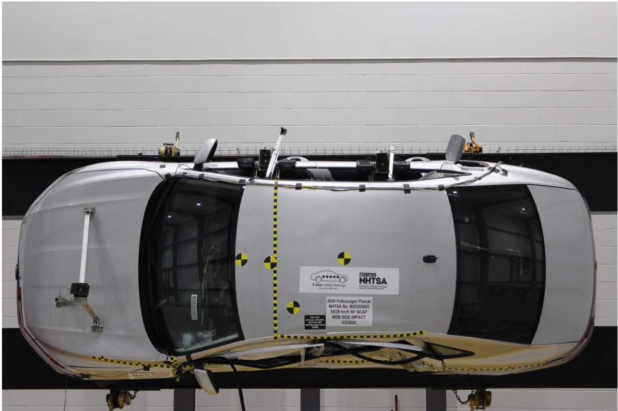
Figure A-97: FMVSS No. 301 Static Rollover 90 Degrees
