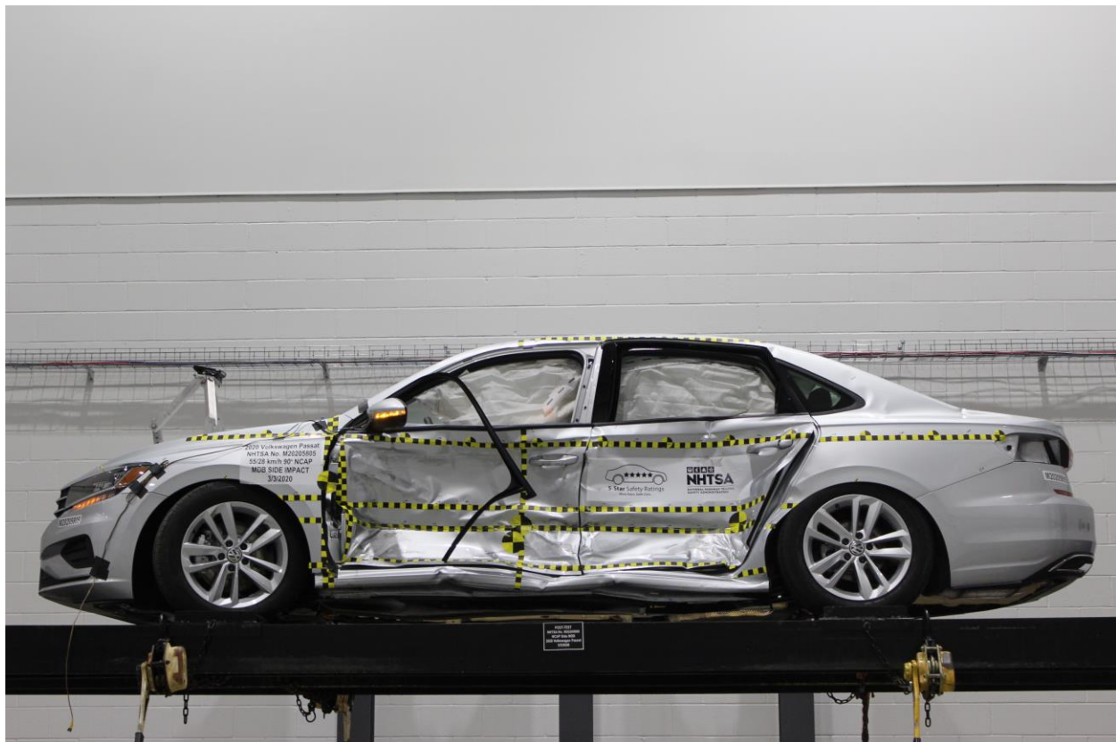
Figure A-96: FMVSS No. 301 Static Rollover 0 Degrees
