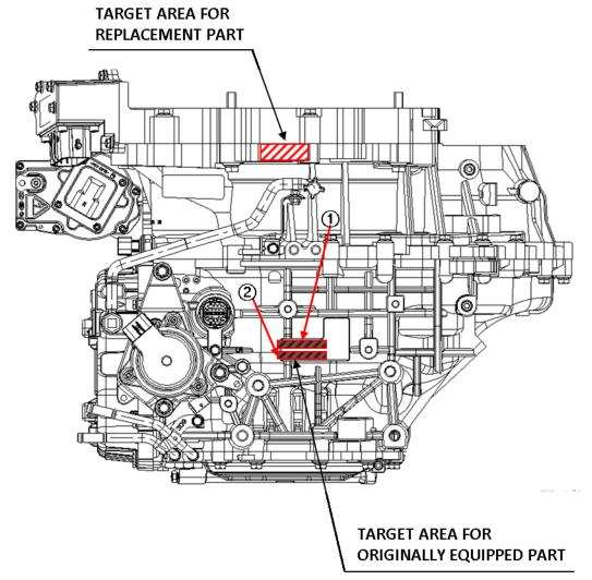
XVIN plate for originally equipped part will be attached to either ① or ②.
