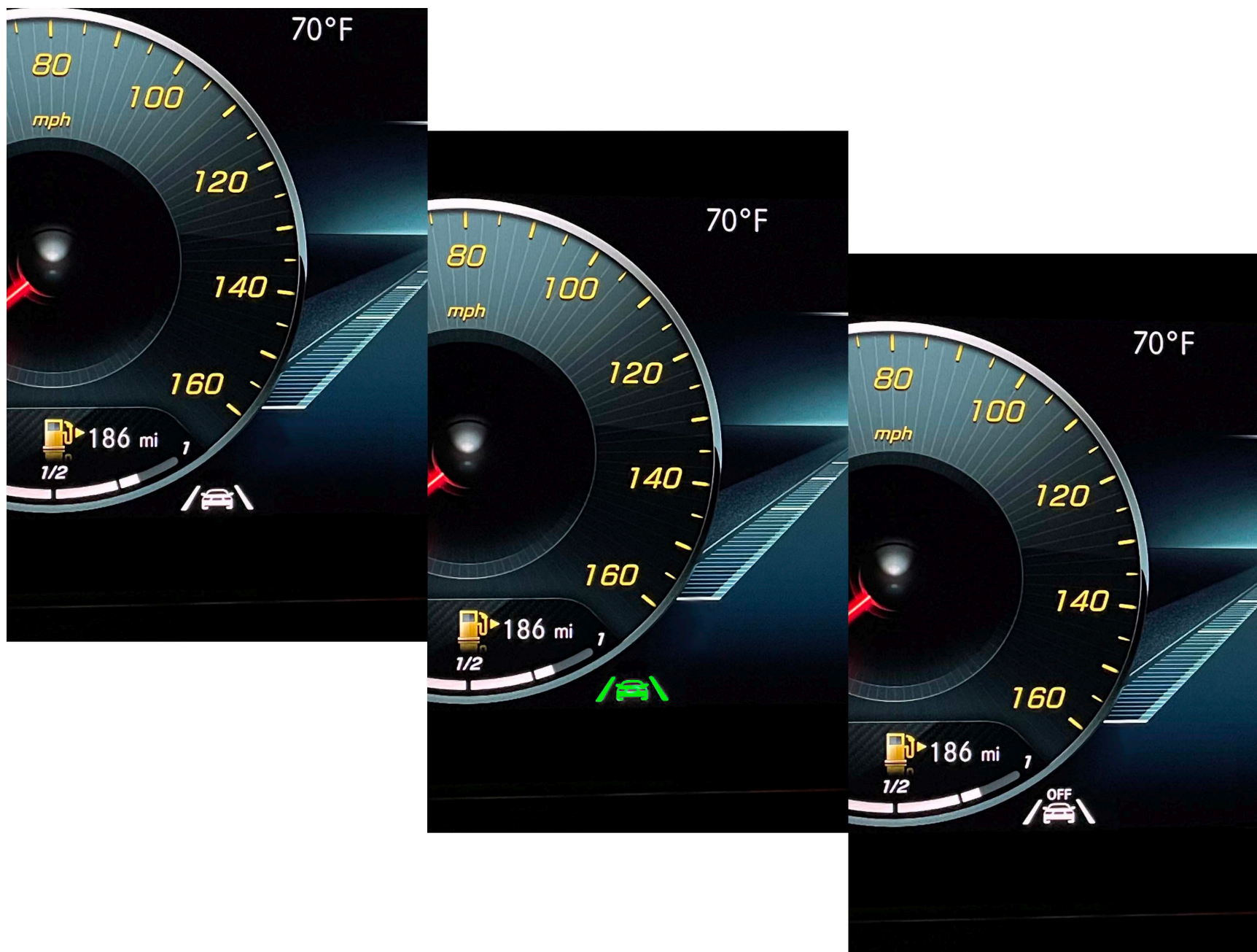
Figure A12. Visual Alert Showing (L-R): "Active, Not Operating", "Active, Operating", and "Deactivated or Malfunction"
