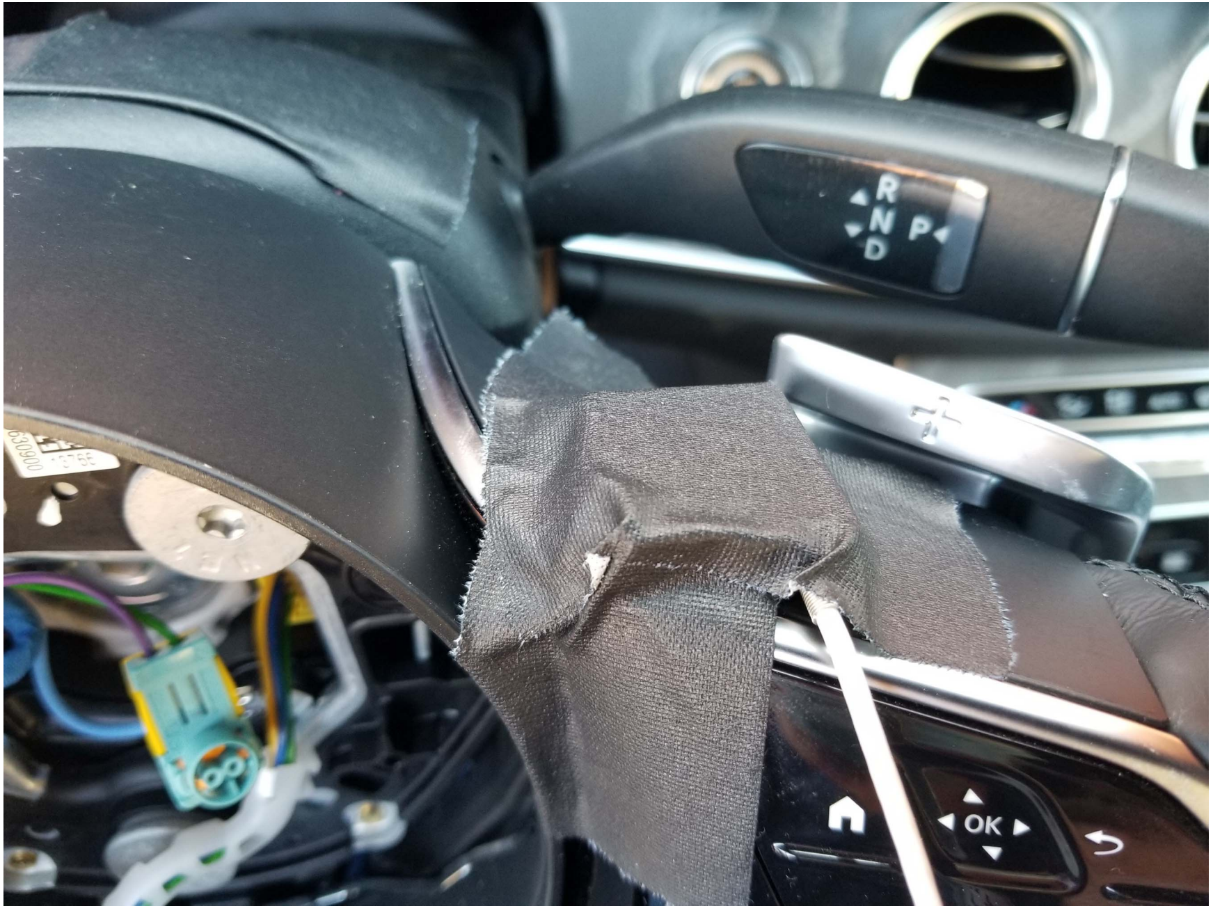
Figure A7. Sensor for Detecting Haptic Alerts
