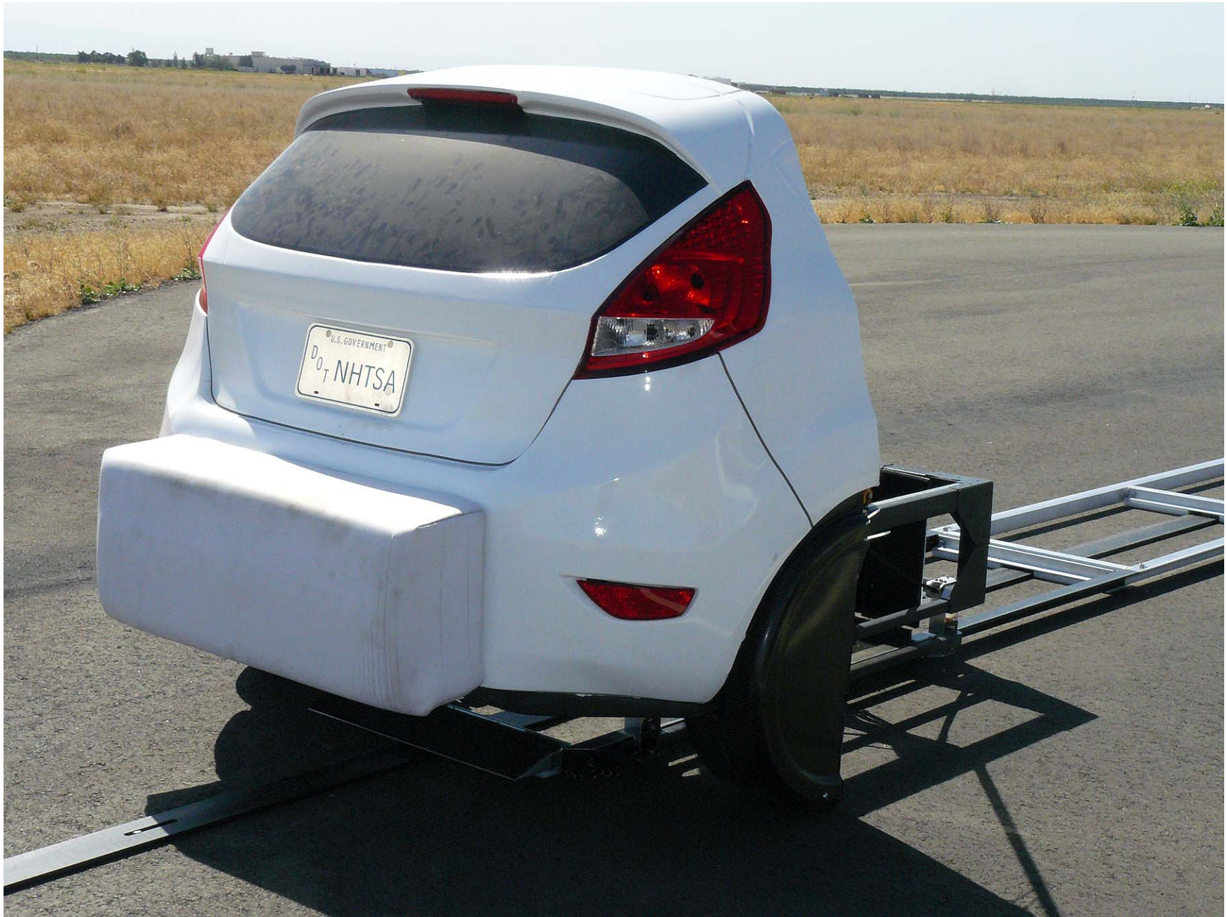
Figure A6. Rear View of Principal Other Vehicle (SSV)
