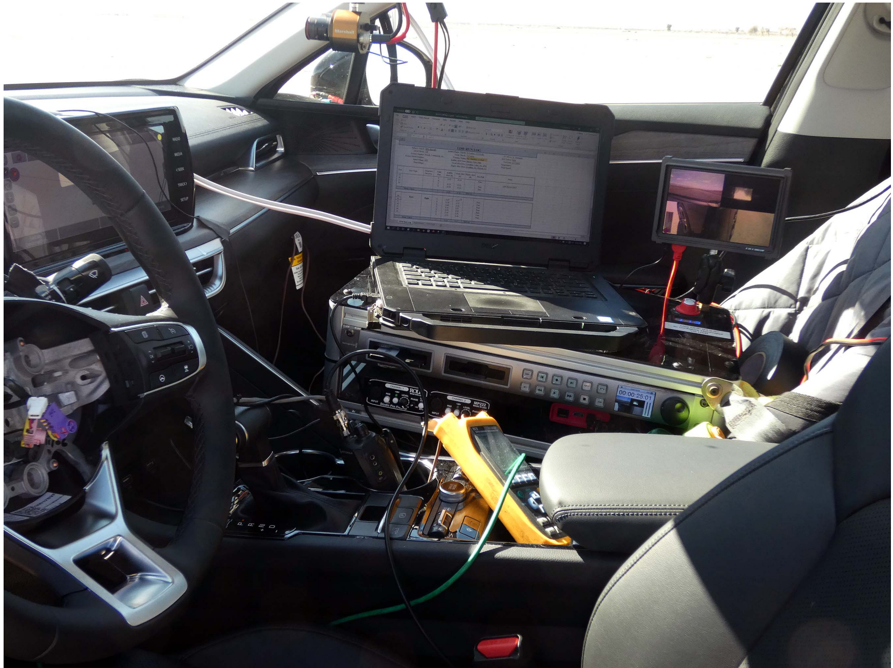
Figure A8. Computer Installed in Subject Vehicle
