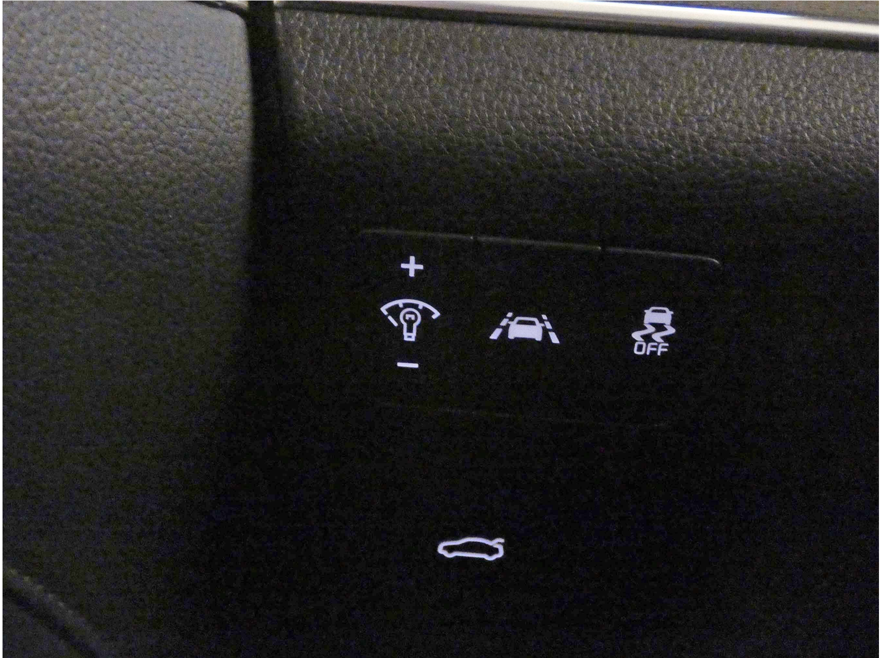
Figure A12. LDW On/Off Switch
