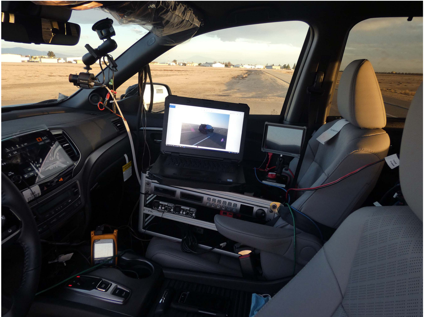
Figure A10. Computer Installed in Subject Vehicle
