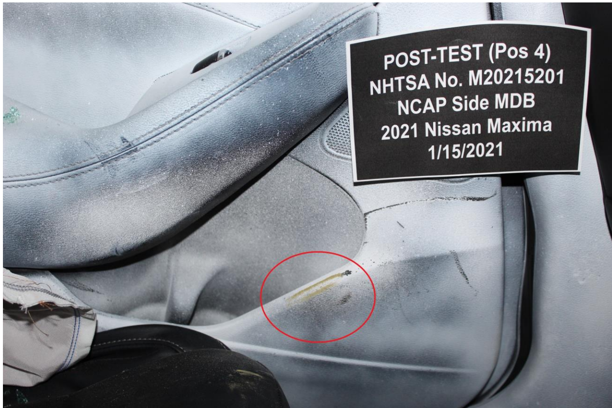
Figure A-81: Post-Test Rear Passenger Dummy Close-Up Knee Contact View
