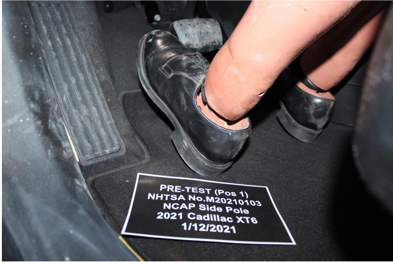
Figure A-32: Pre-Test Placement of Dummy's Feet
