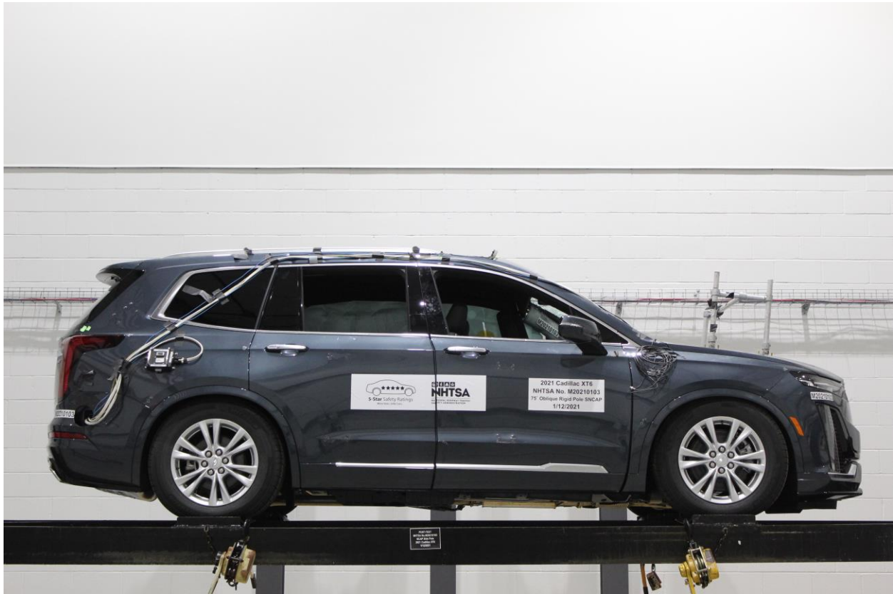
Figure A-63: FMVSS No. 301 Static Rollover 0 Degrees
