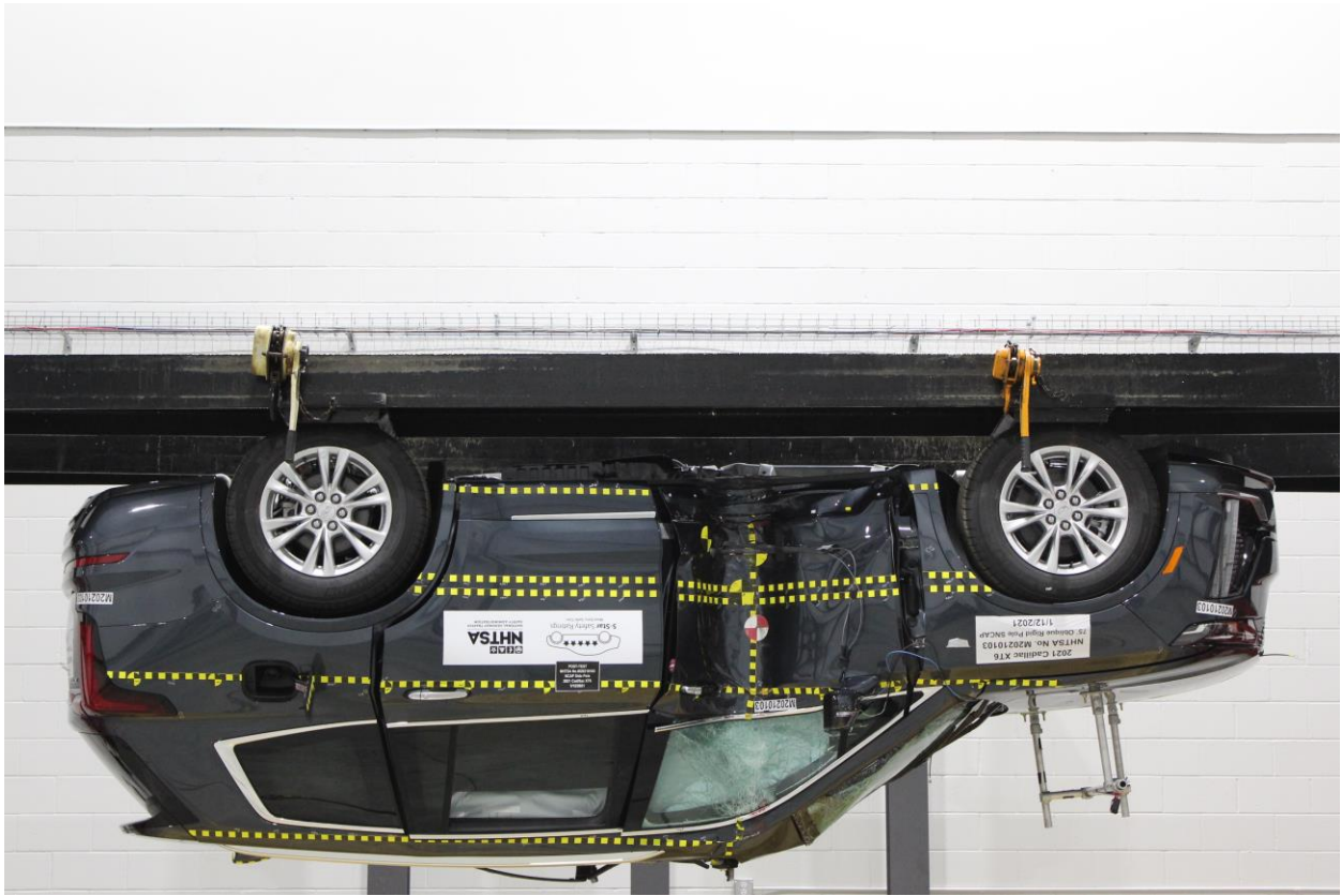
Figure A-65: FMVSS No. 301 Static Rollover 180 Degrees
