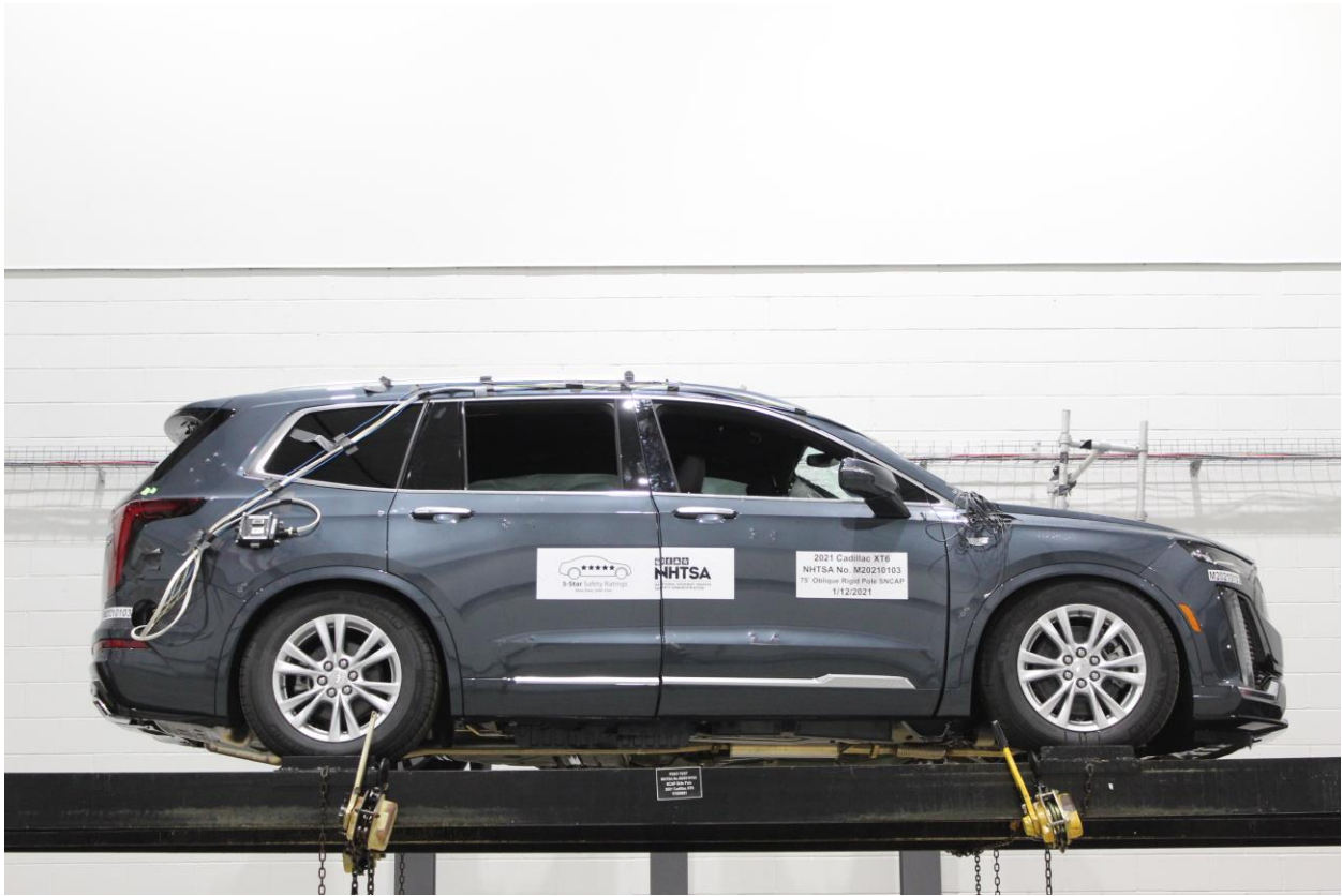
Figure A-67: FMVSS No. 301 Static Rollover 360 Degrees
