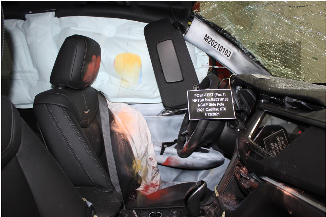
Figure A-71: Post-Test View of Shattered Vehicle Inner Door Panel
