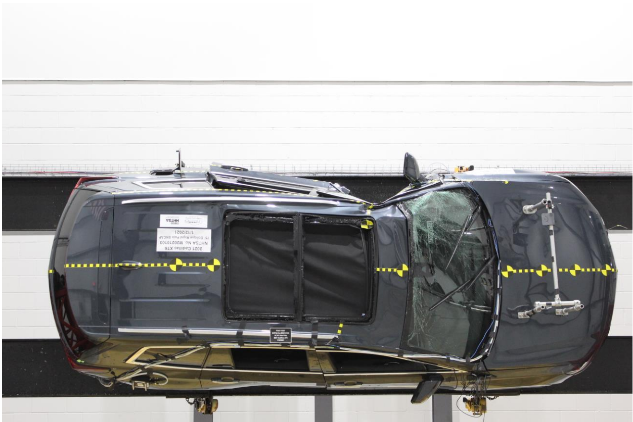
Figure A-66: FMVSS No. 301 Static Rollover 270 Degrees
