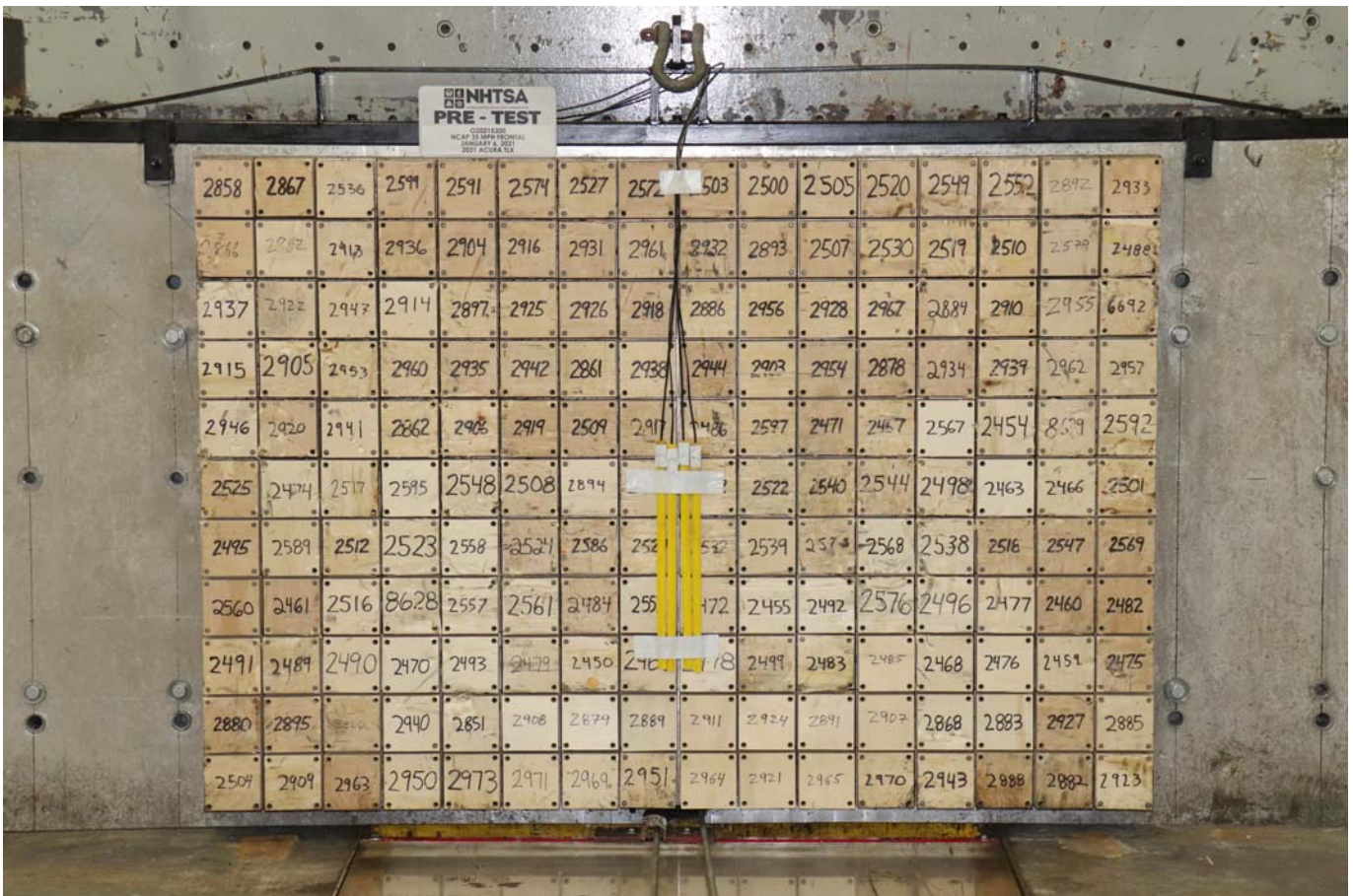
Photo No. 002 - Pre-Test Load Cell Wall
