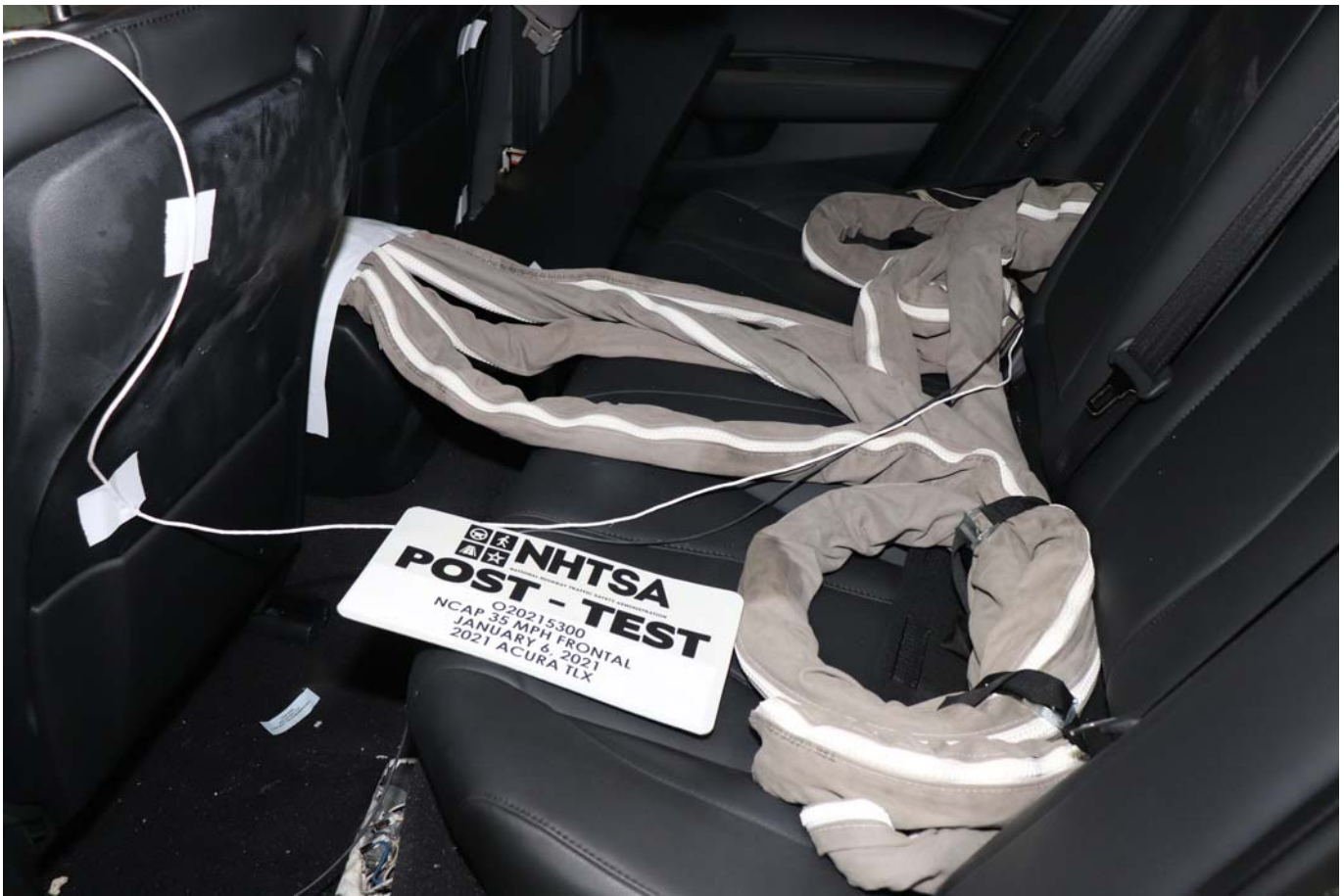
Photo No. 029 - Post-Test Dummy Cable Routing
