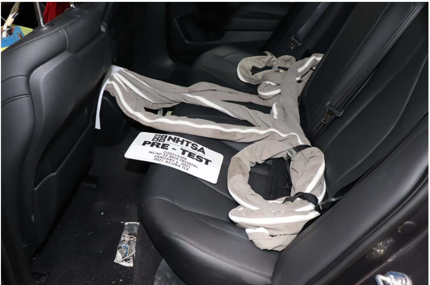
Photo No. 028 - Pre-Test Dummy Cable Routing
