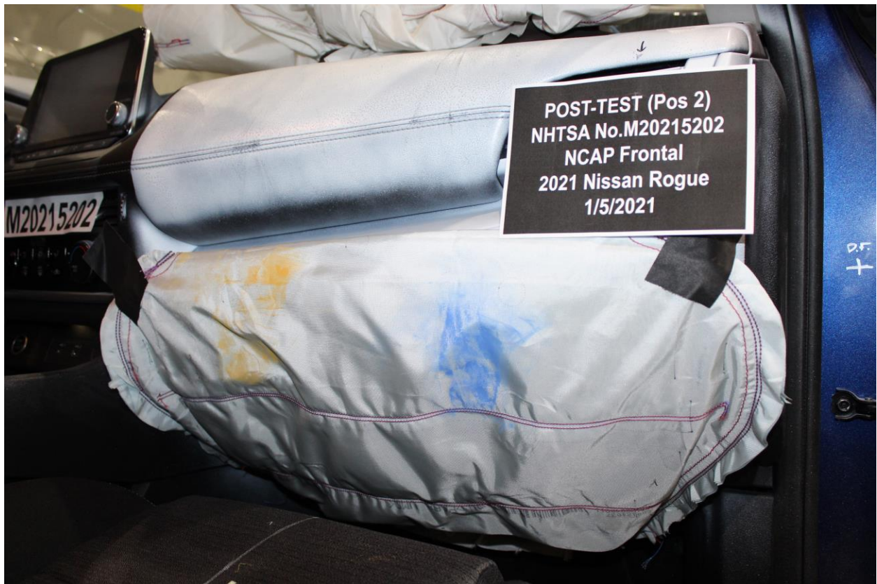
Figure A-68: Post-Test Passenger's Side Knee Bolster
