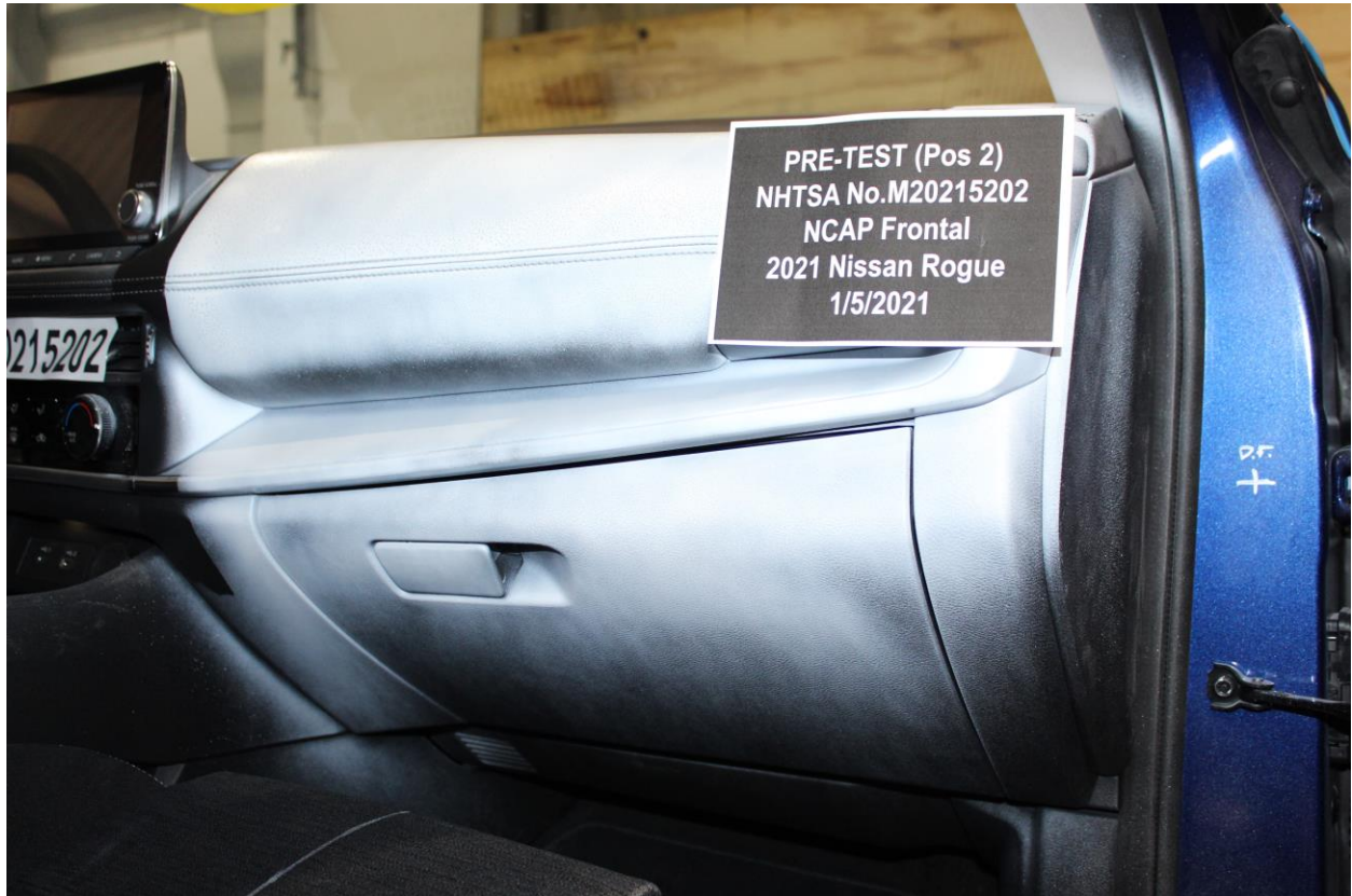
Figure A-67: Pre-Test Passenger's Side Knee Bolster
