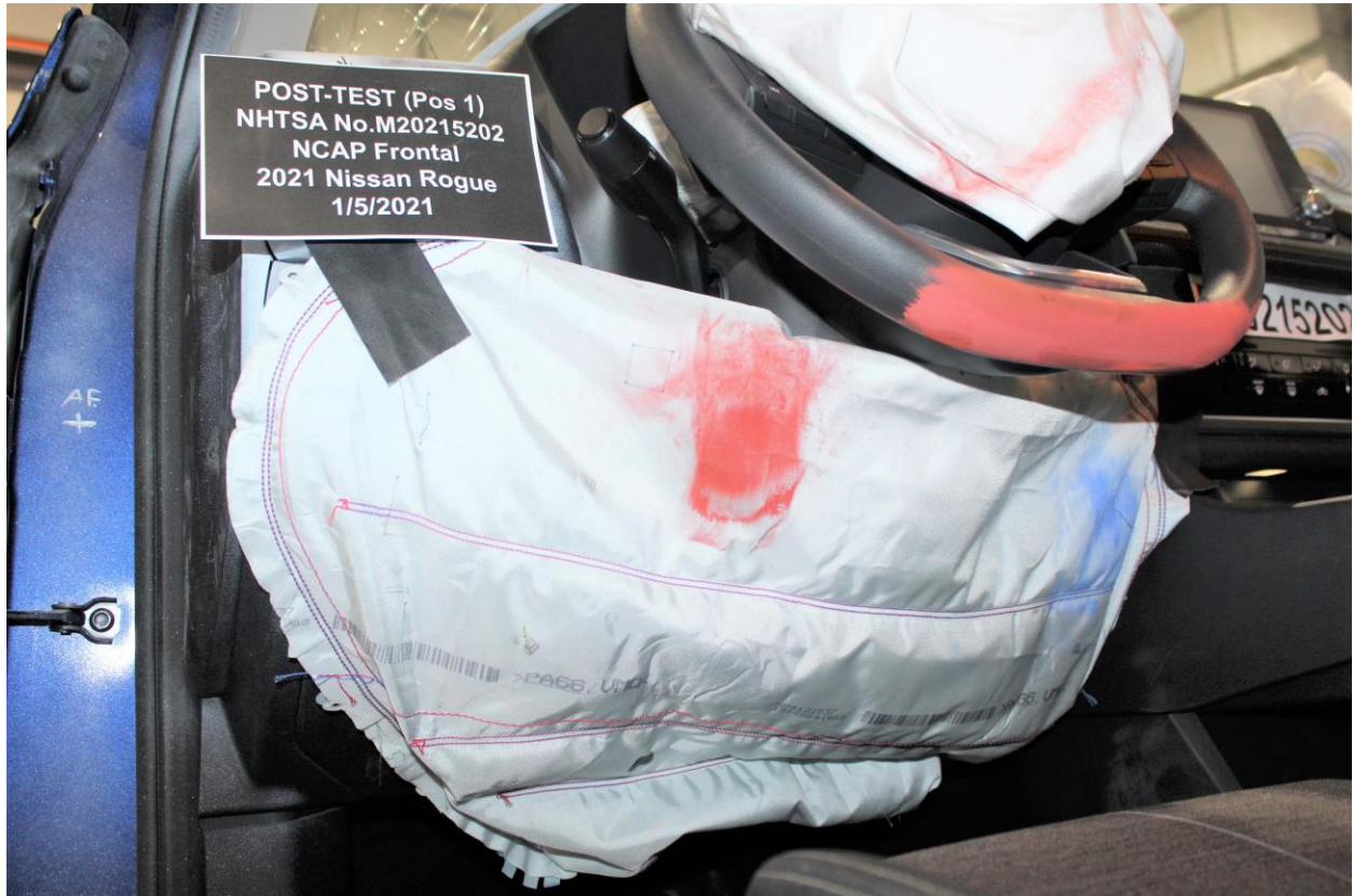
Figure A-45: Post-Test Driver's Side Knee Bolster
