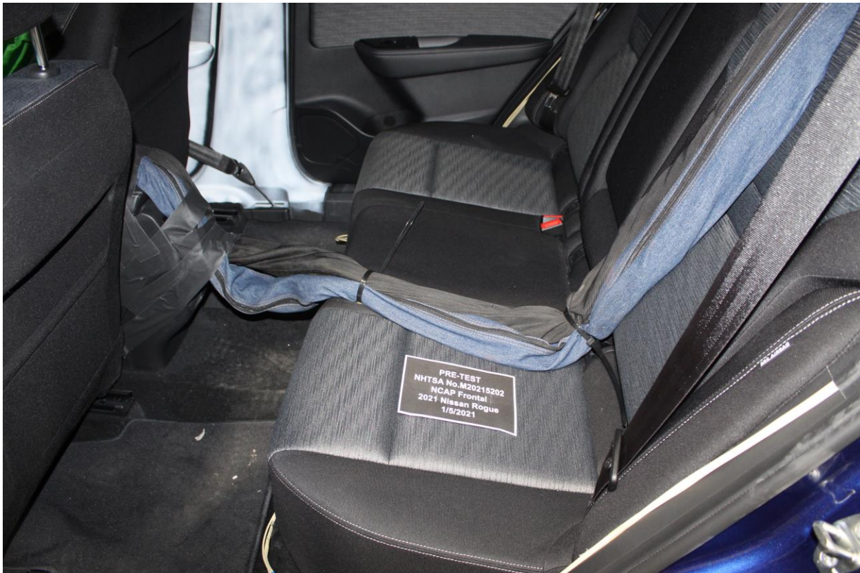
Figure A-28: Pre-Test Dummy Cable Routing
