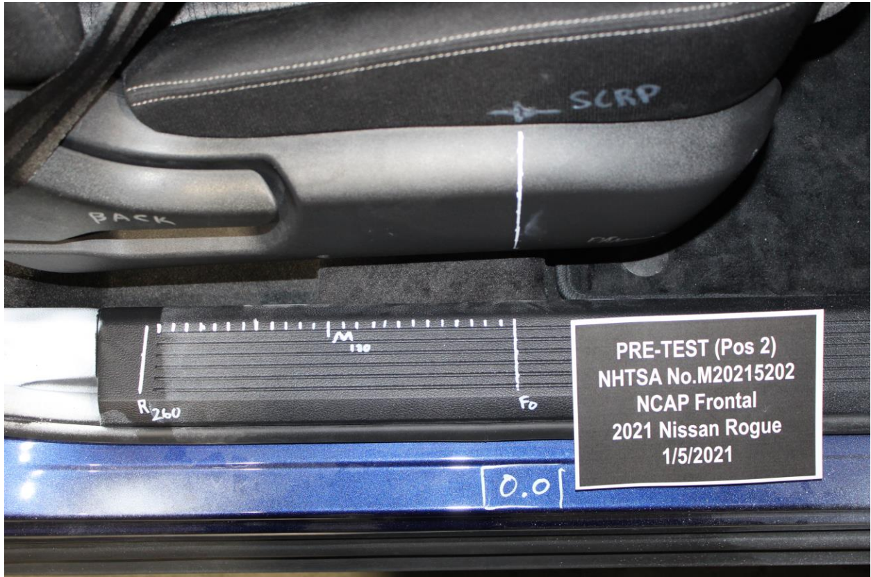
Figure A-59: Pre-Test Passenger's Seat Fore-Aft Markings
