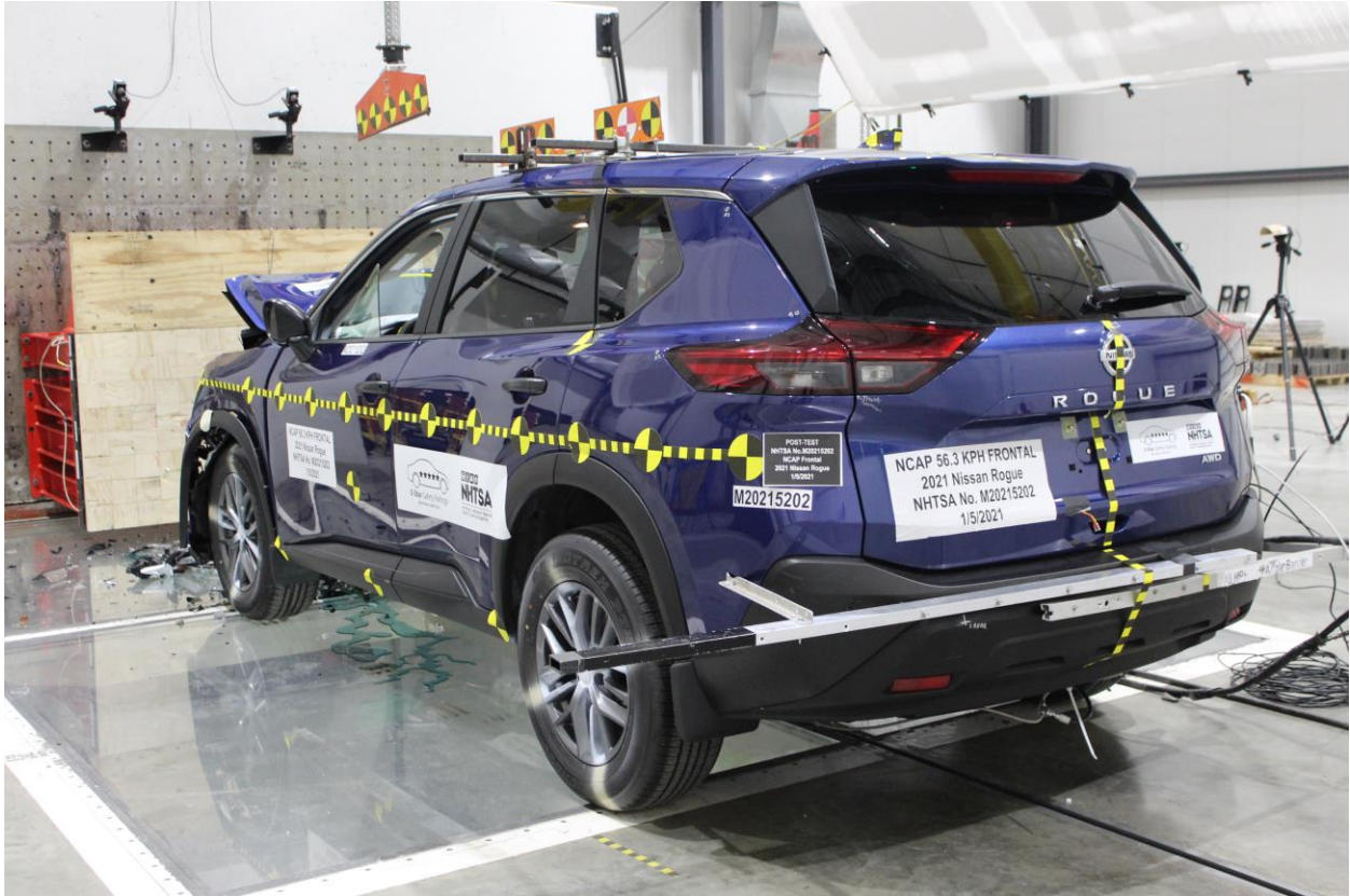
Figure A-17: Post-Test Left Rear 3-4 View
