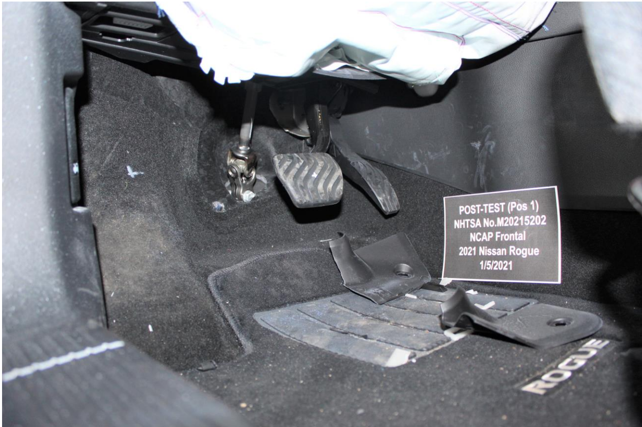
Figure A-47: Post-Test Driver's Side Floorpan
