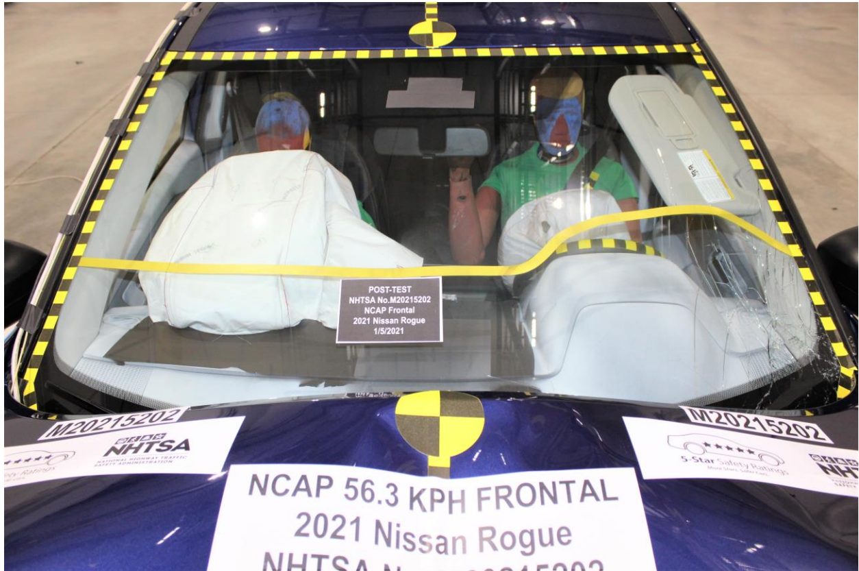
Figure A-19: Post-Test Windshield View
