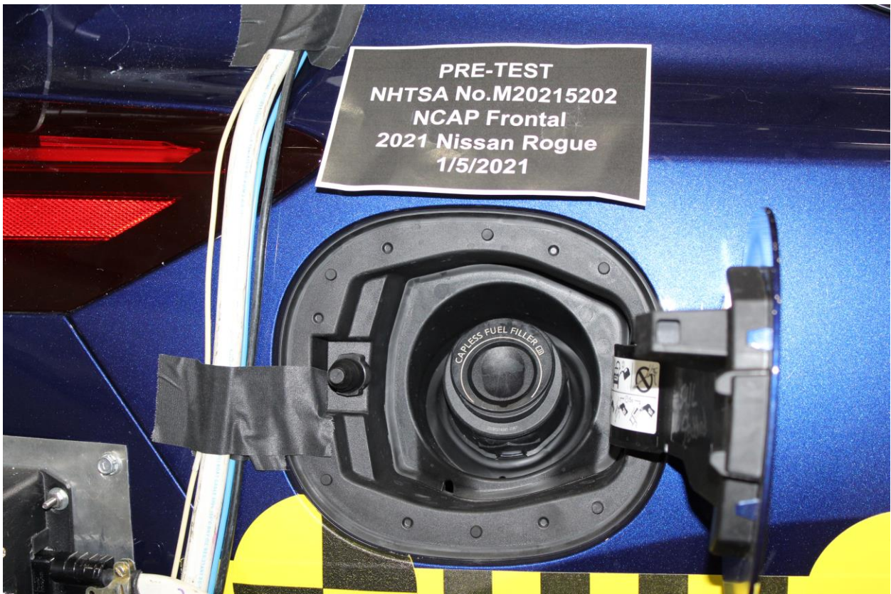
Figure A-22: Pre-Test Fuel Filler Cap View
