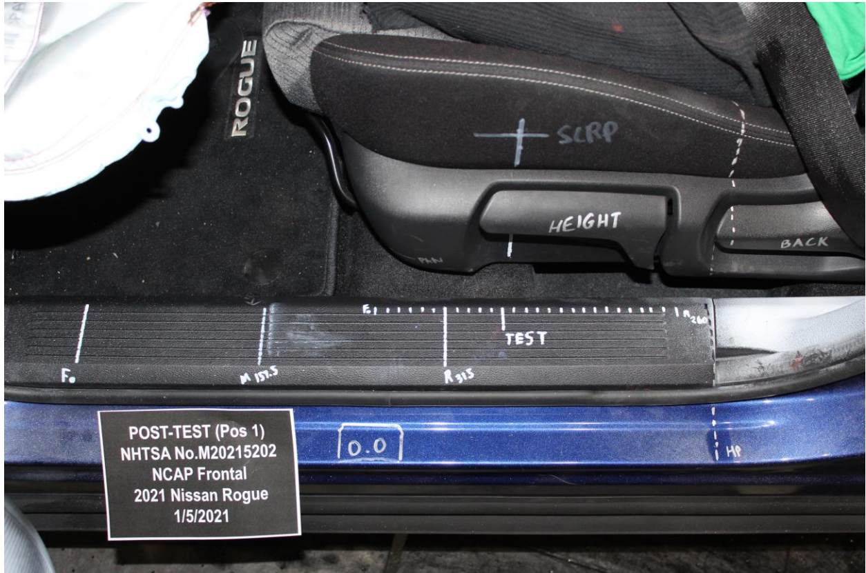
Figure A-37: Post-Test Driver's Seat Fore-Aft Markings
