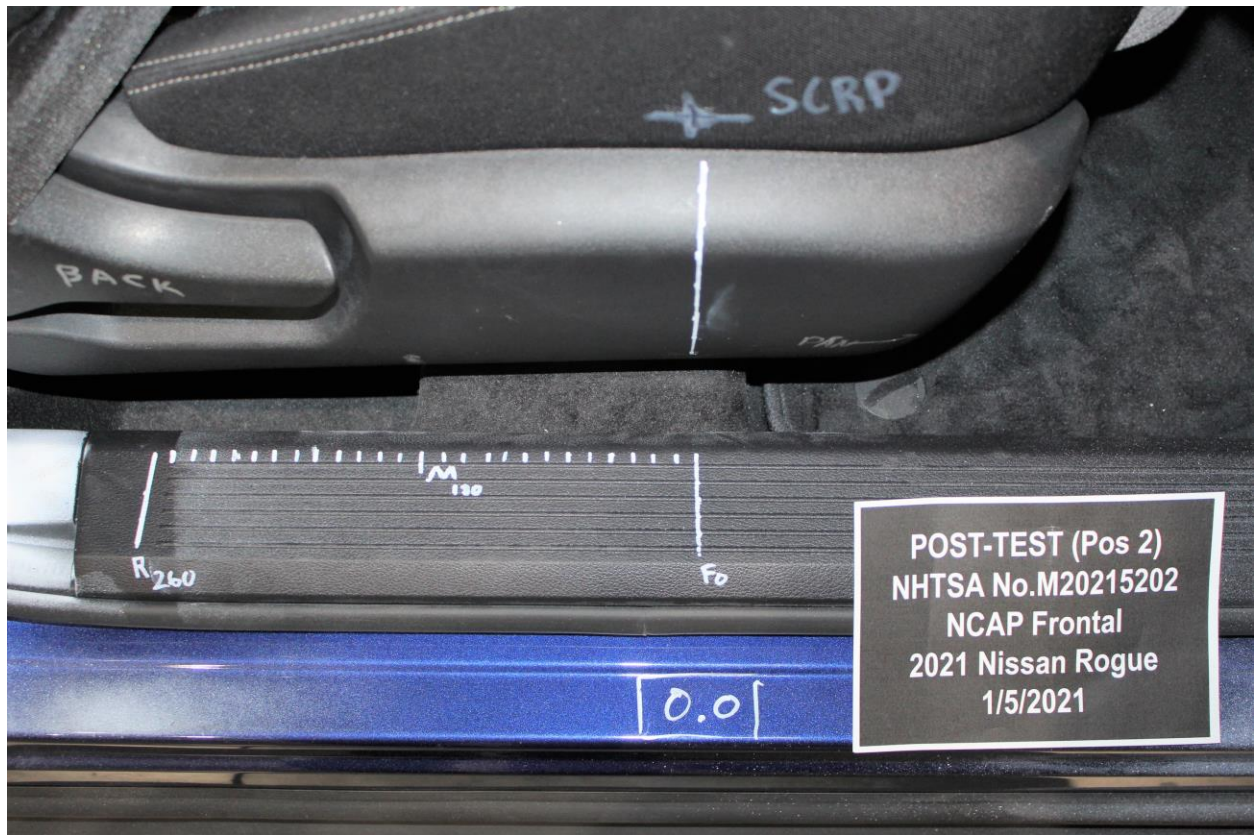
Figure A-60: Post-Test Passenger's Seat Fore-Aft Markings
