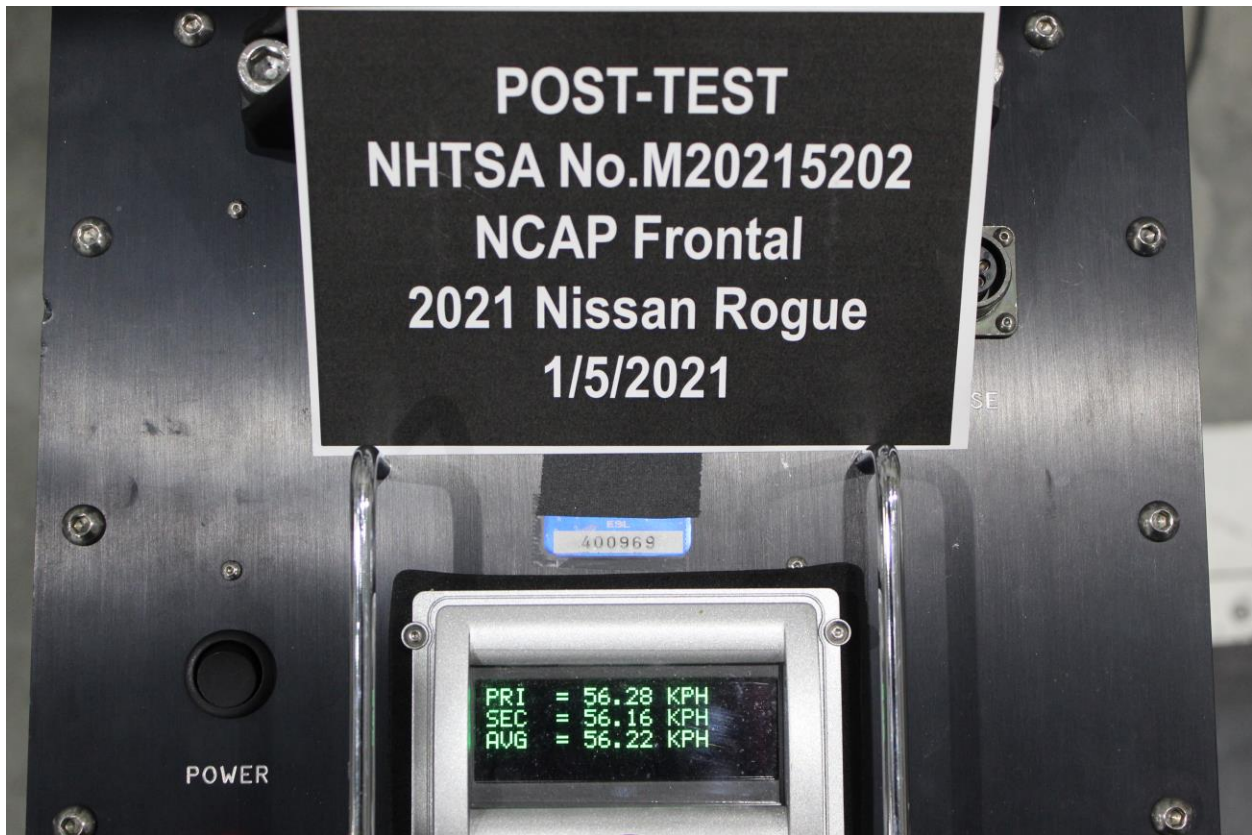
Figure A-76: Post-Test Speed Trap Read-Out
