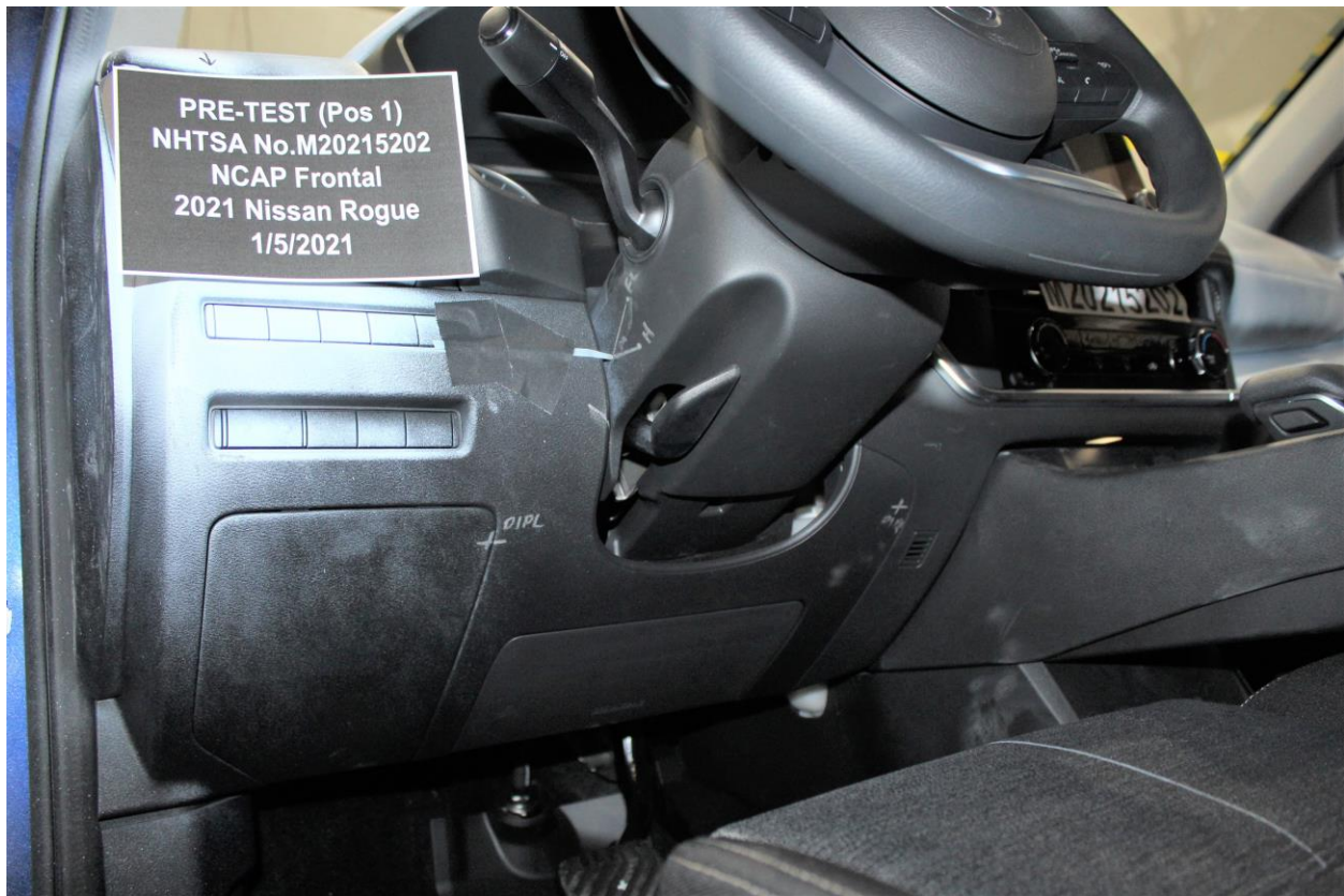
Figure A-44: Pre-Test Driver's Side Knee Bolster
