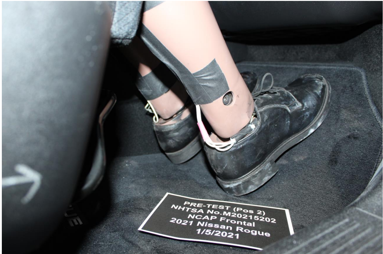
Figure A-65: Pre-Test Passenger Dummy Feet
