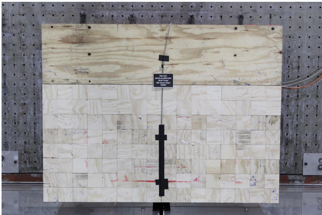
Figure A-2: Pre-Test Load Cell Wall
