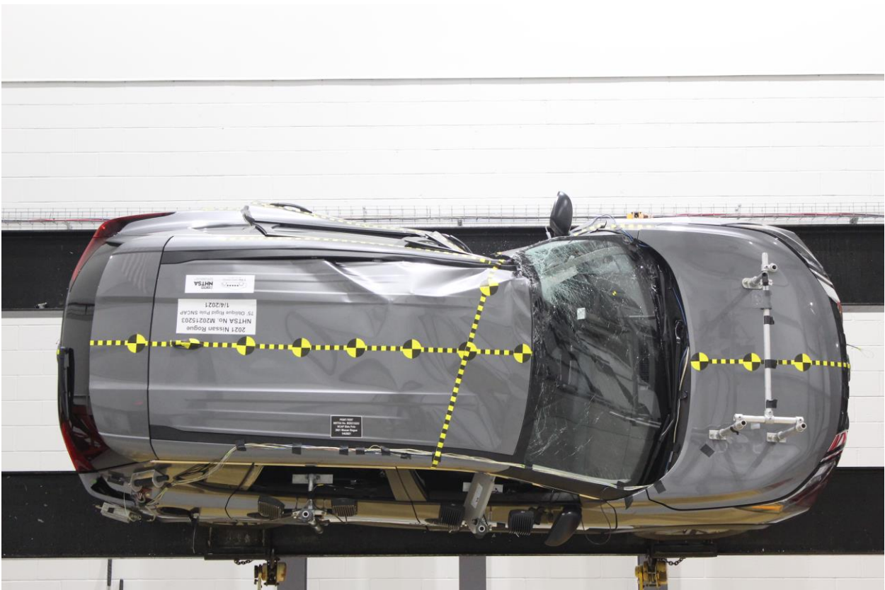
Figure A-64: FMVSS No. 301 Static Rollover 90 Degrees
