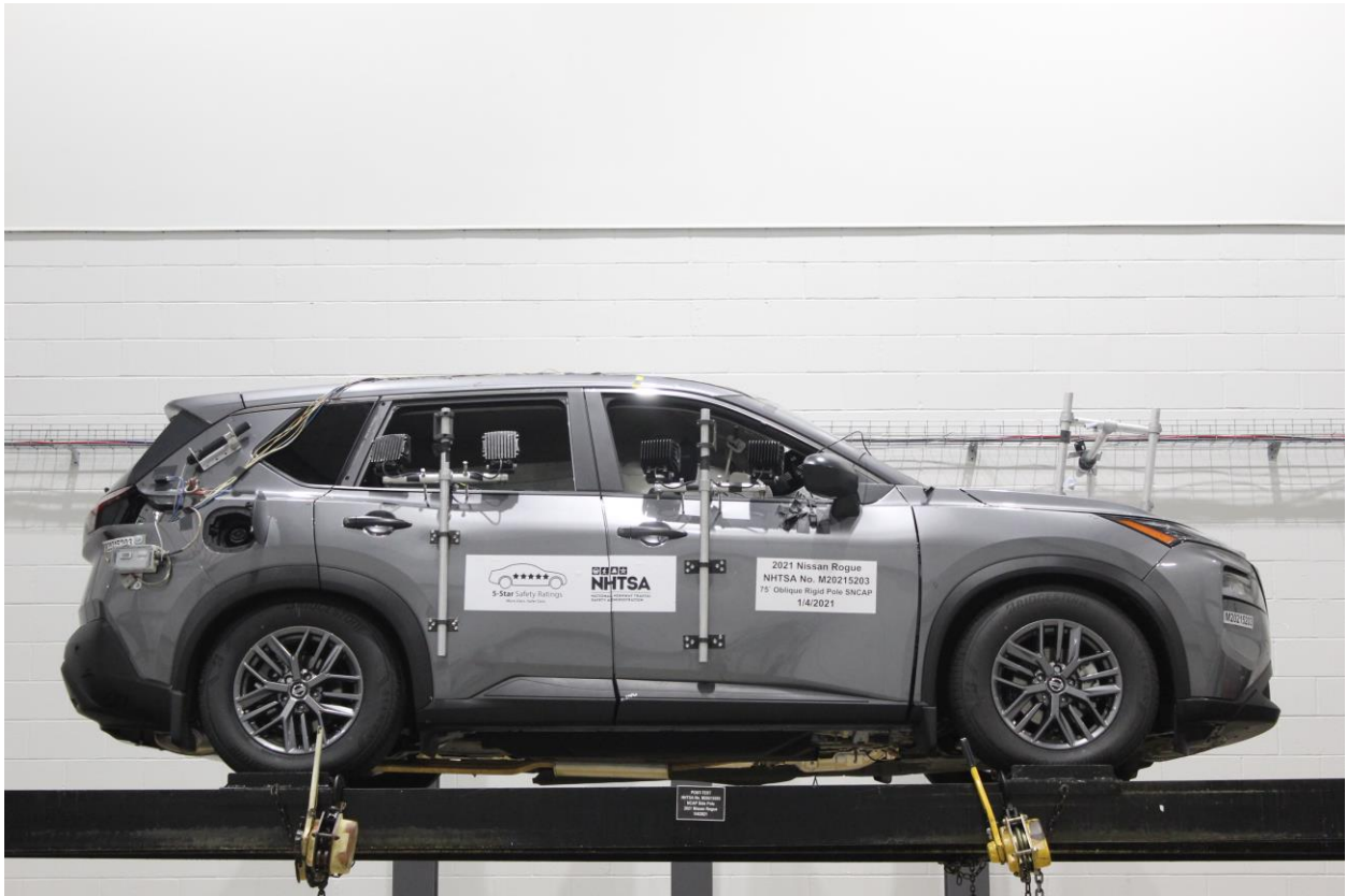
Figure A-67: FMVSS No. 301 Static Rollover 360 Degrees
