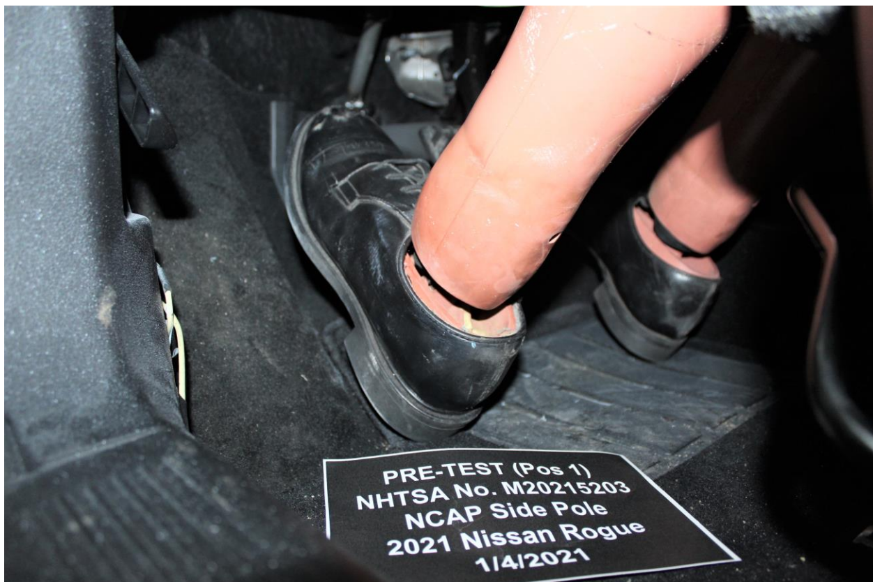
Figure A-32: Pre-Test Placement of Dummy's Feet
