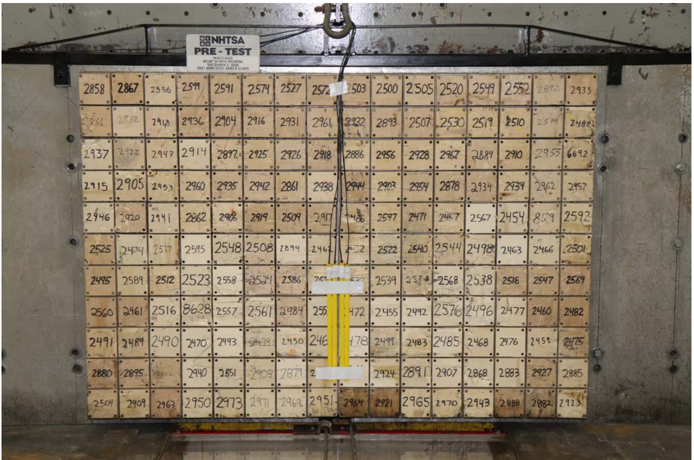
Photo No. 002 - Pre-Test Load Cell Wall
