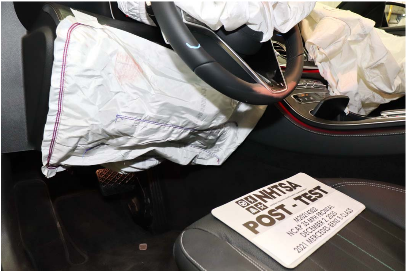
Photo No. 045 - Post-Test Driver Side Knee Bolster
