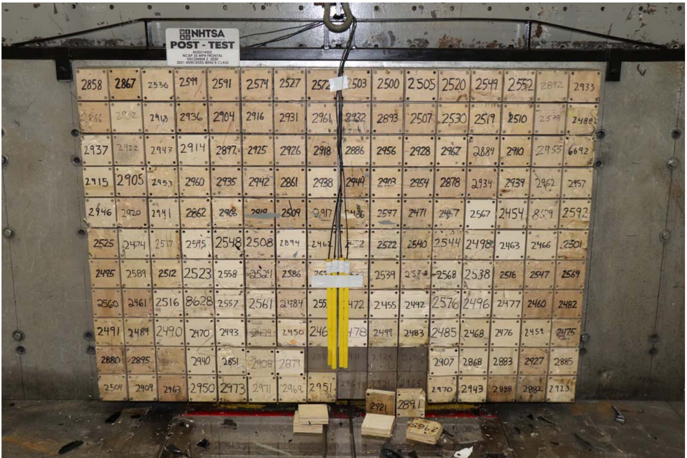
Photo No. 003 - Post-Test Load Cell Wall
