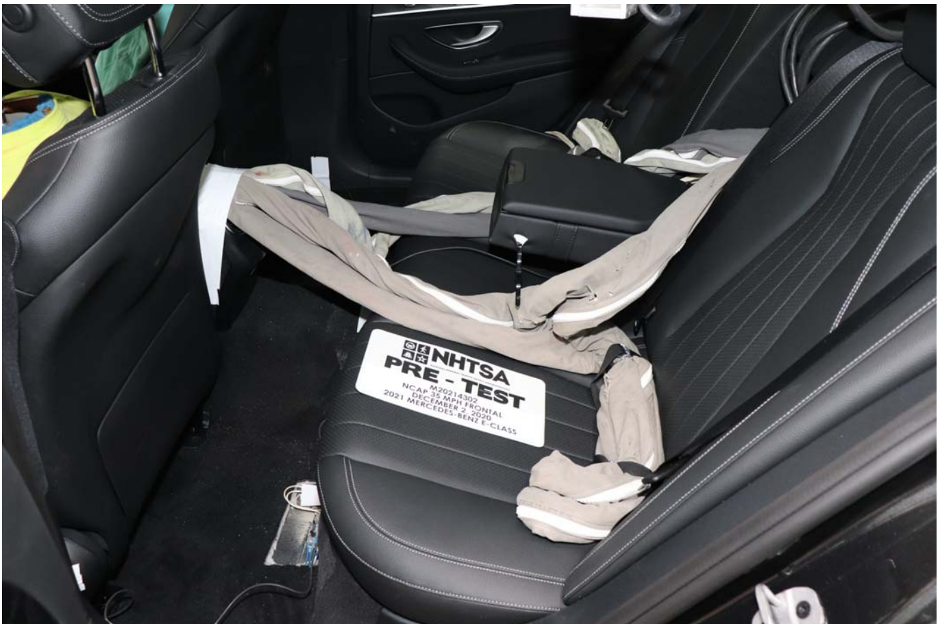
Photo No. 028 - Pre-Test Dummy Cable Routing
