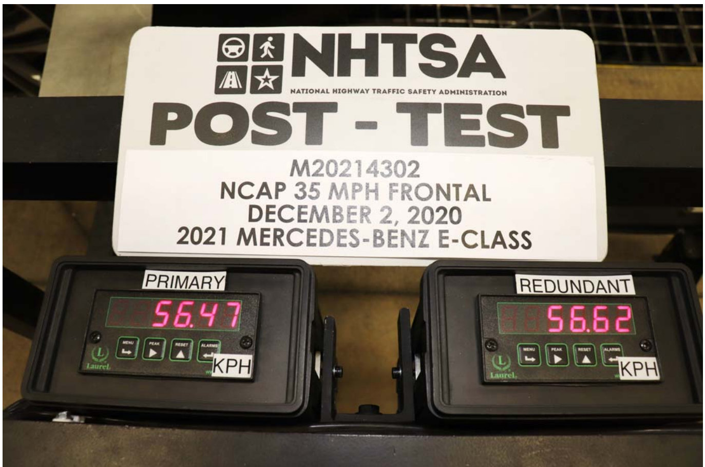
Photo No. 076 - Post-Test Speed Trap Read-Out
