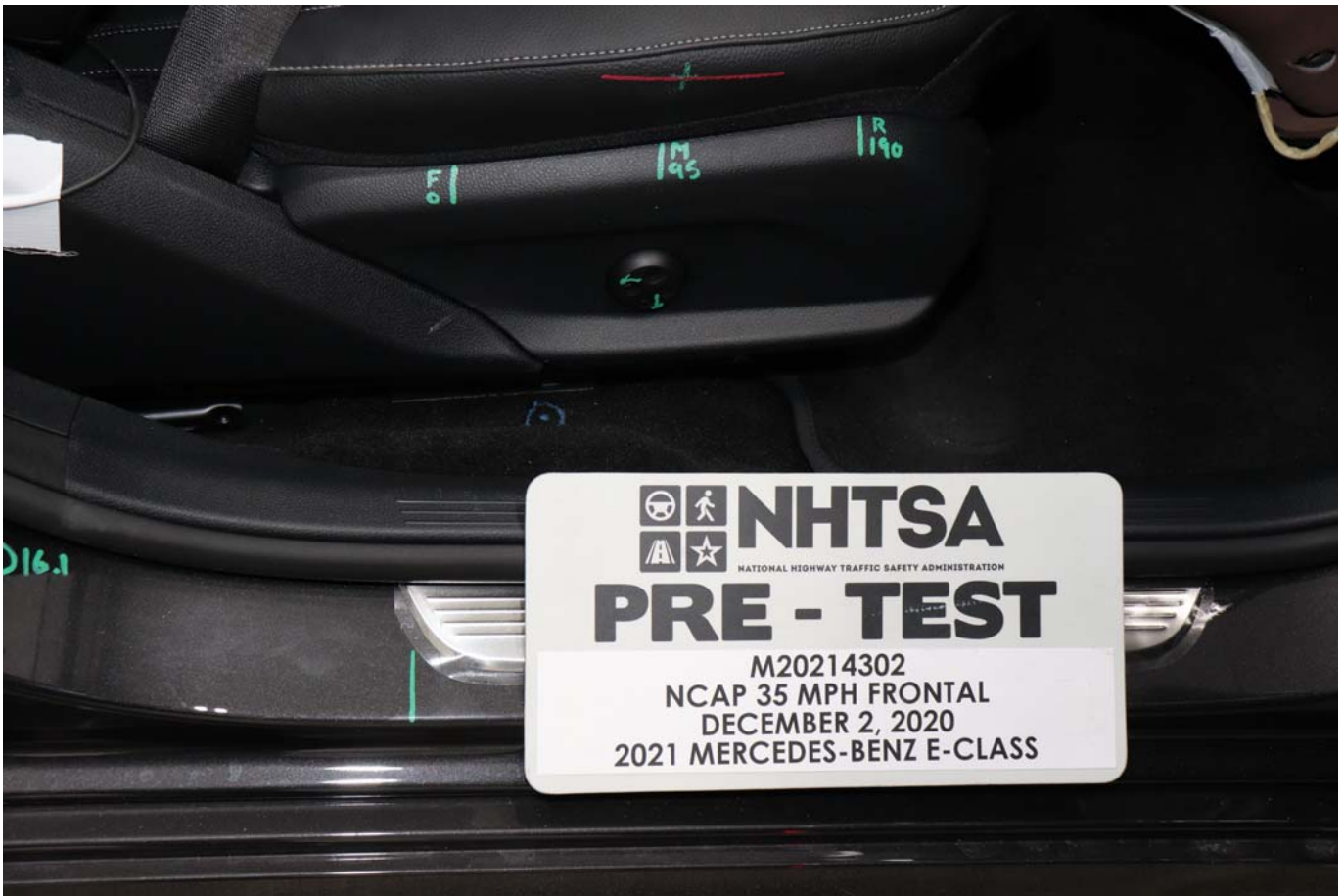
Photo No. 059 - Pre-Test Passenger Seat Fore-Aft Markings
