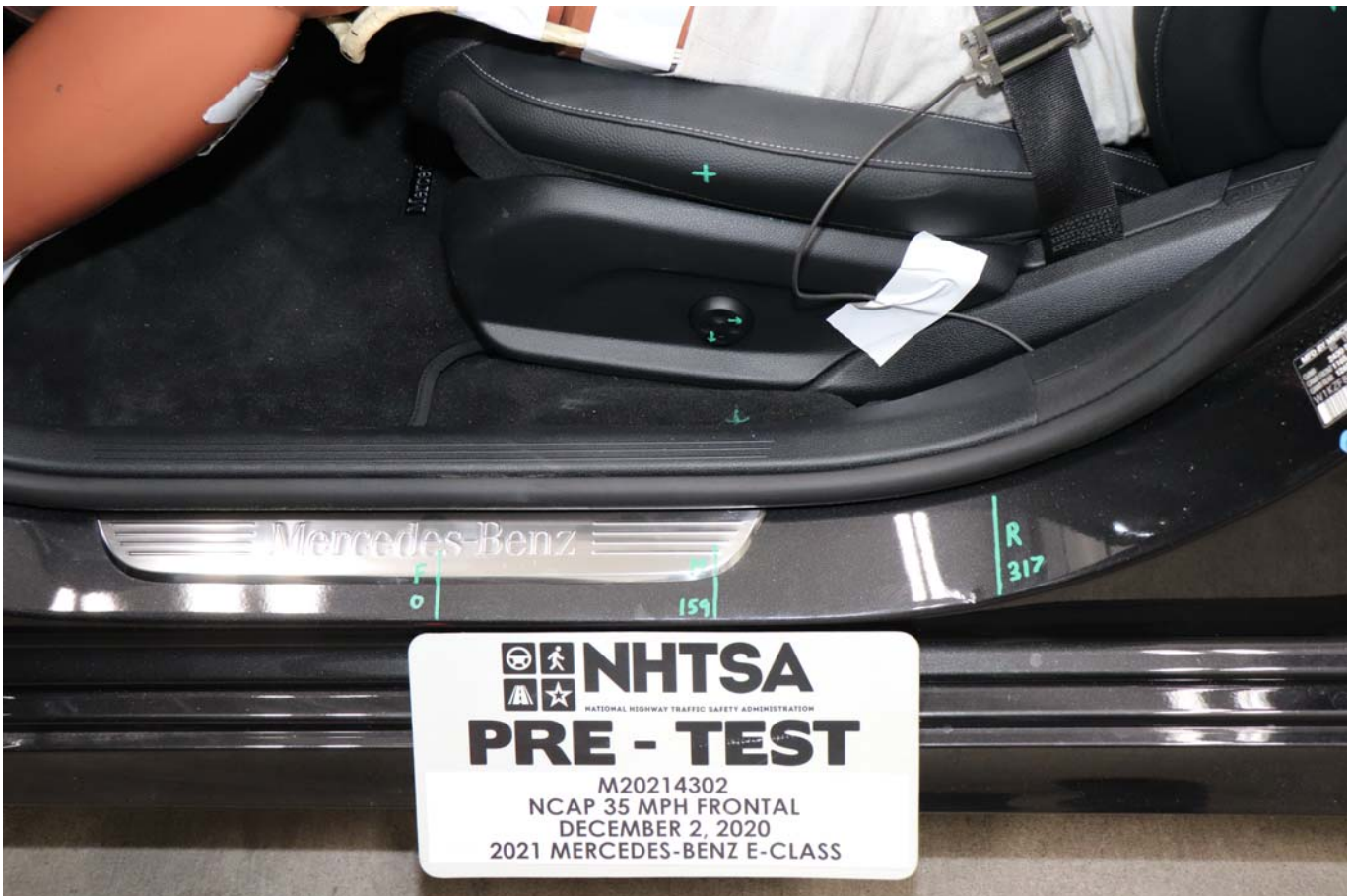
Photo No. 036 - Pre-Test Driver Seat Fore-Aft Markings
