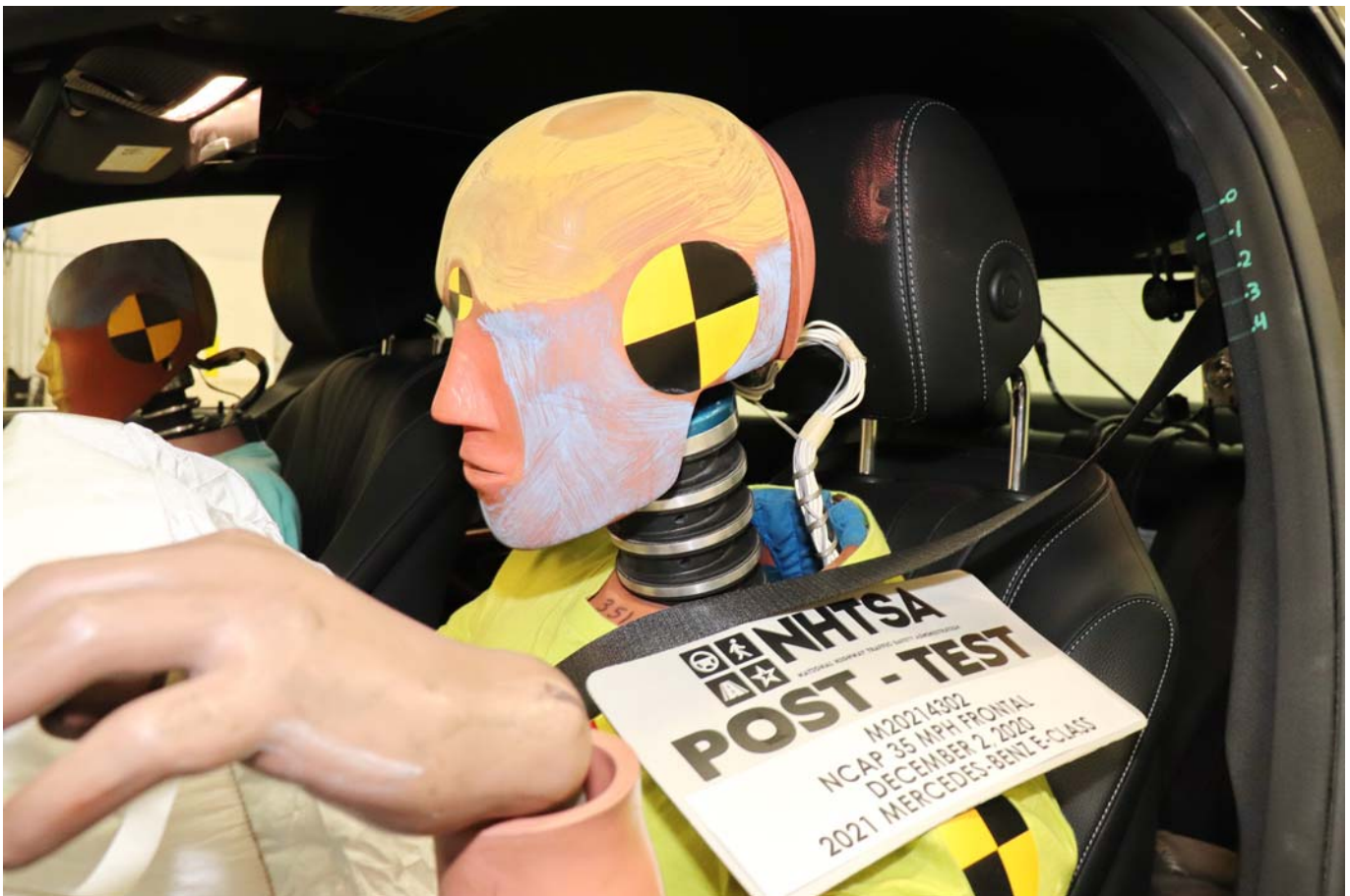
Photo No. 048 - Post-Test Driver Dummy Face
