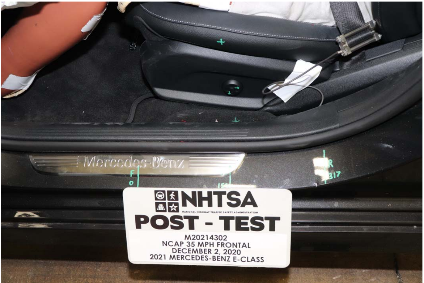
Photo No. 037 - Post-Test Driver Seat Fore-Aft Markings
