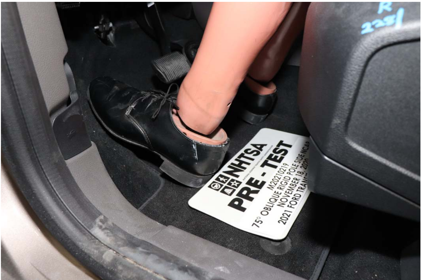
Photo No. 032 - Pre-Test Placement of Dummy Feet
