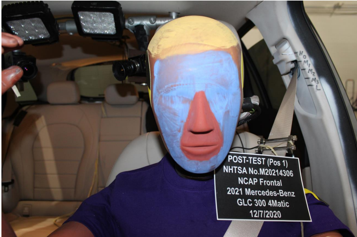
Figure A-48: Post-Test Driver Dummy Face
