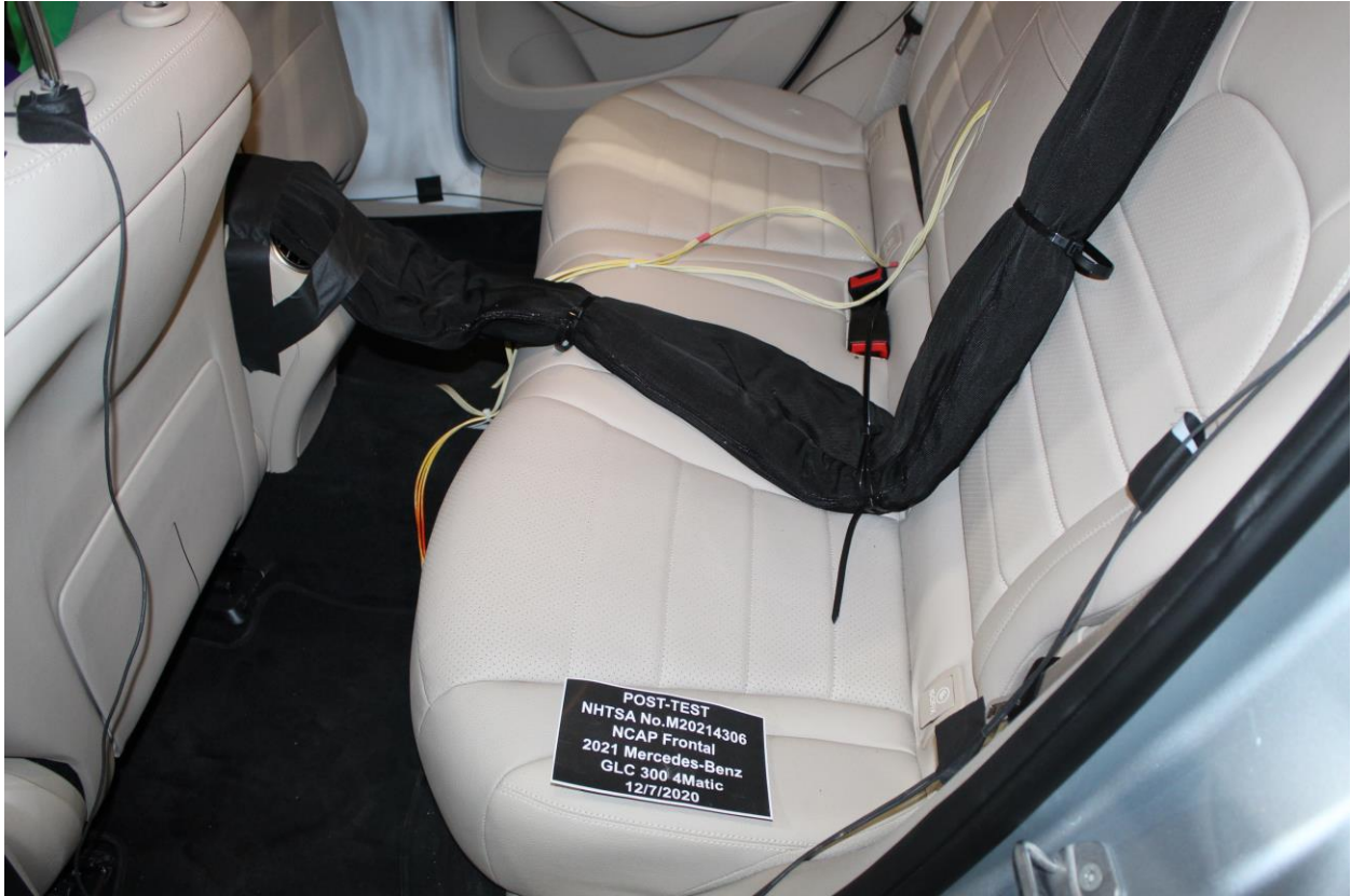
Figure A-29: Post-Test Dummy Cable Routing
