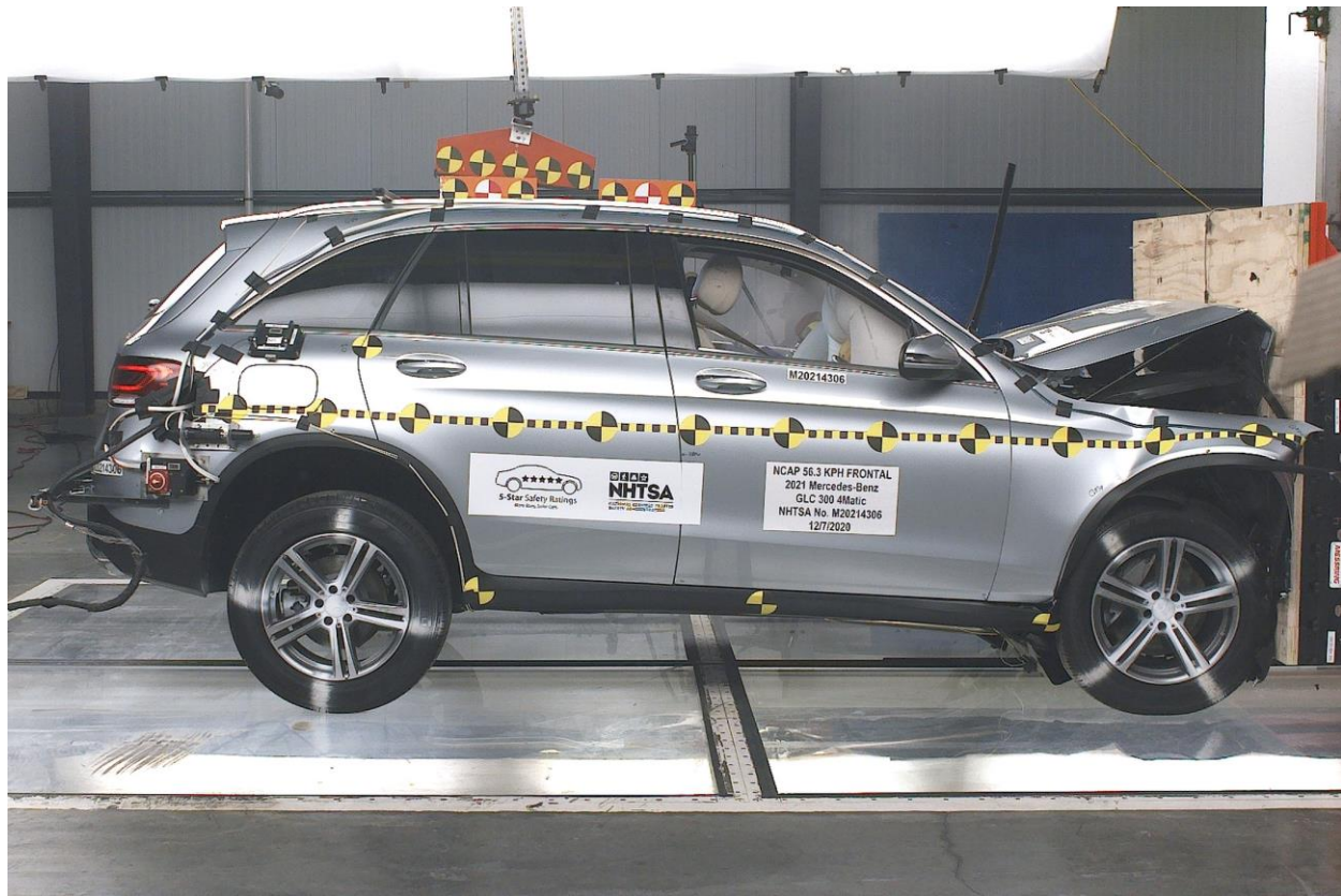
Figure A-82: 2021 Mercedes-Benz GLC 300 4Matic Frontal Impact Event
