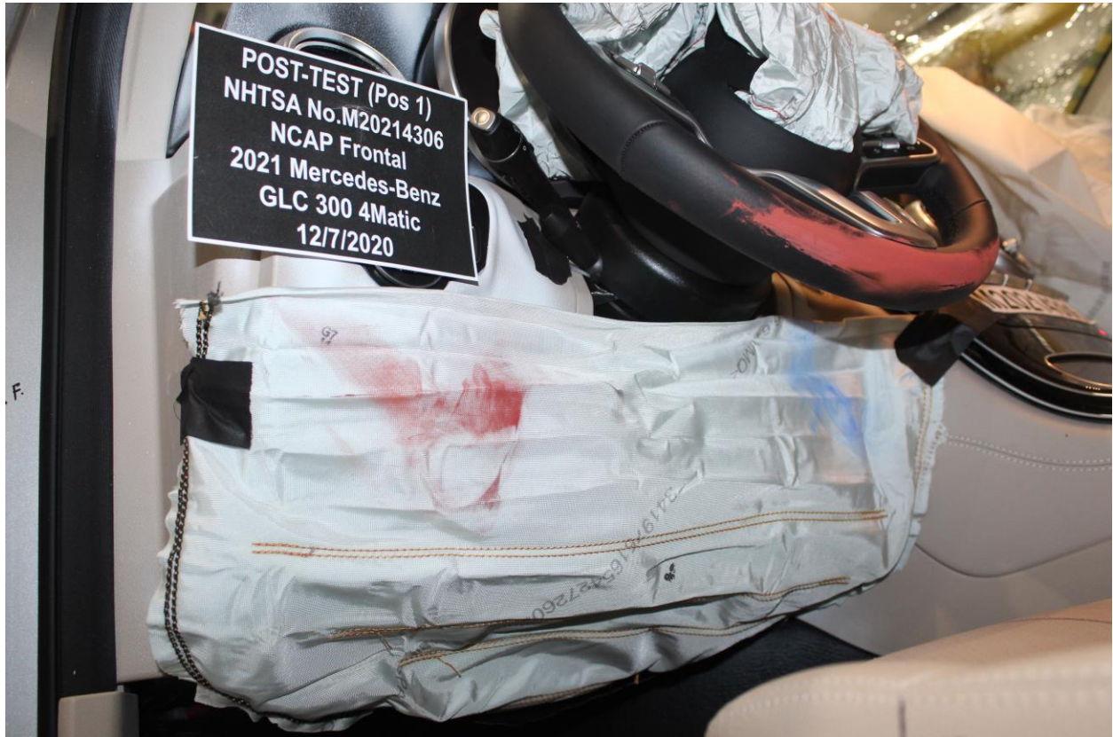
Figure A-45: Post-Test Driver's Side Knee Bolster
