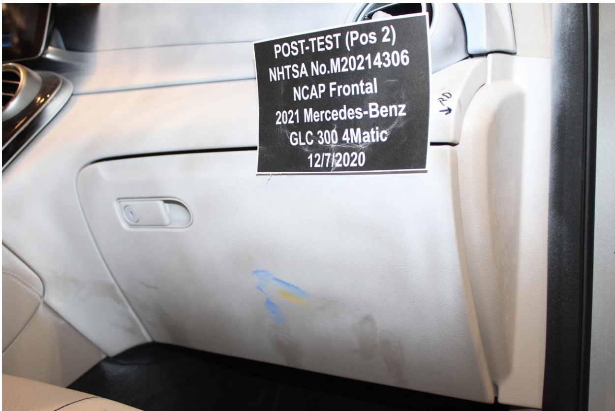
Figure A-68: Post-Test Passenger's Side Knee Bolster
