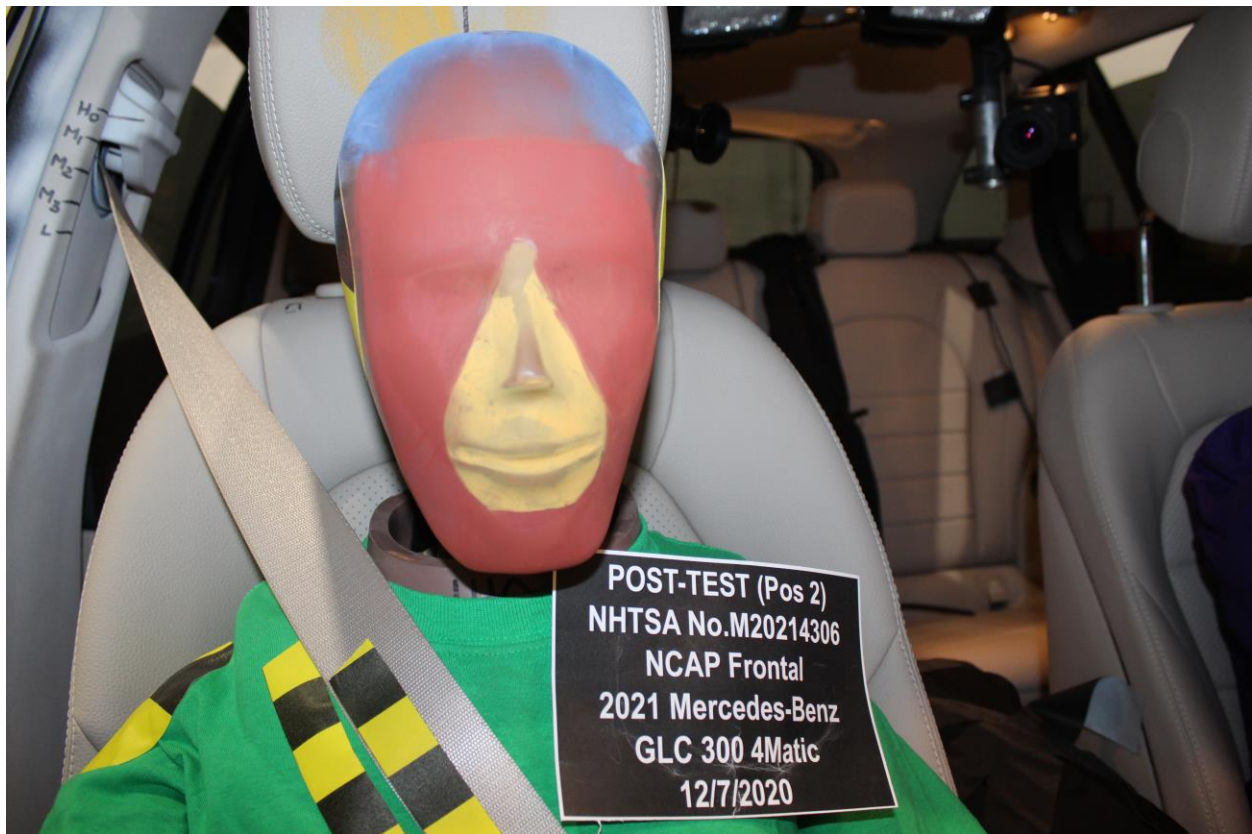
Figure A-71: Post-Test Passenger Dummy Face
