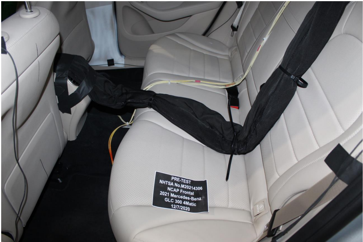
Figure A-28: Pre-Test Dummy Cable Routing
