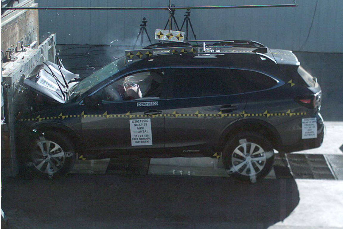
FIGURE 82. 2021 Subaru Outback Frontal Impact Event
