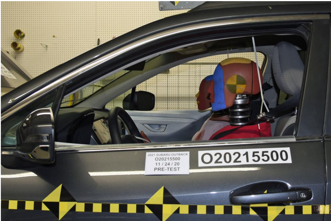
FIGURE 32. Pre-Test Driver Dummy Window View
