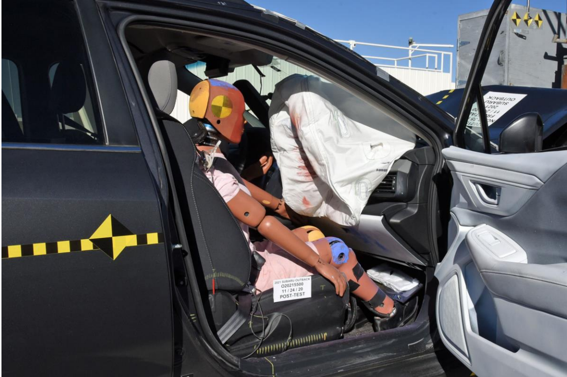
FIGURE 58. Post-Test Passenger Dummy and Vehicle Interior View
