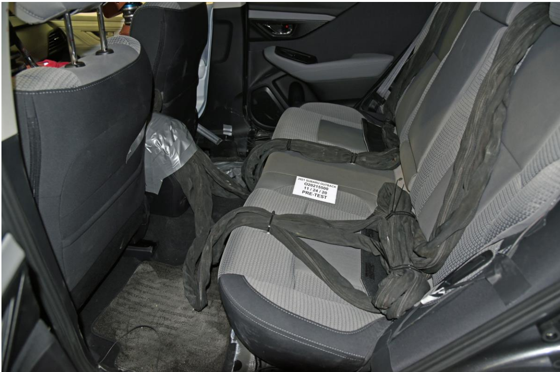
FIGURE 28. Pre-Test Dummy Cable Routing
