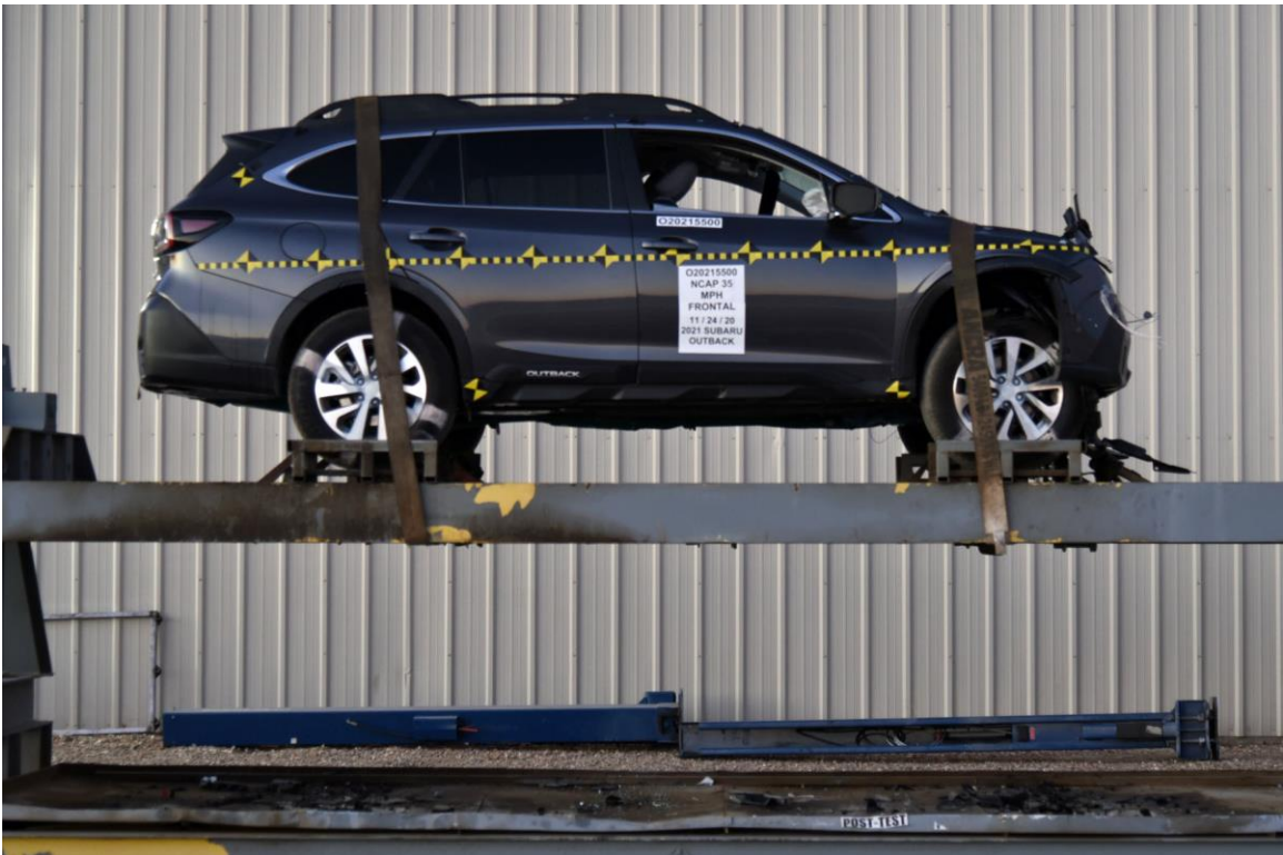
FIGURE 81. Vehicle at 360° on Static Rollover Device
