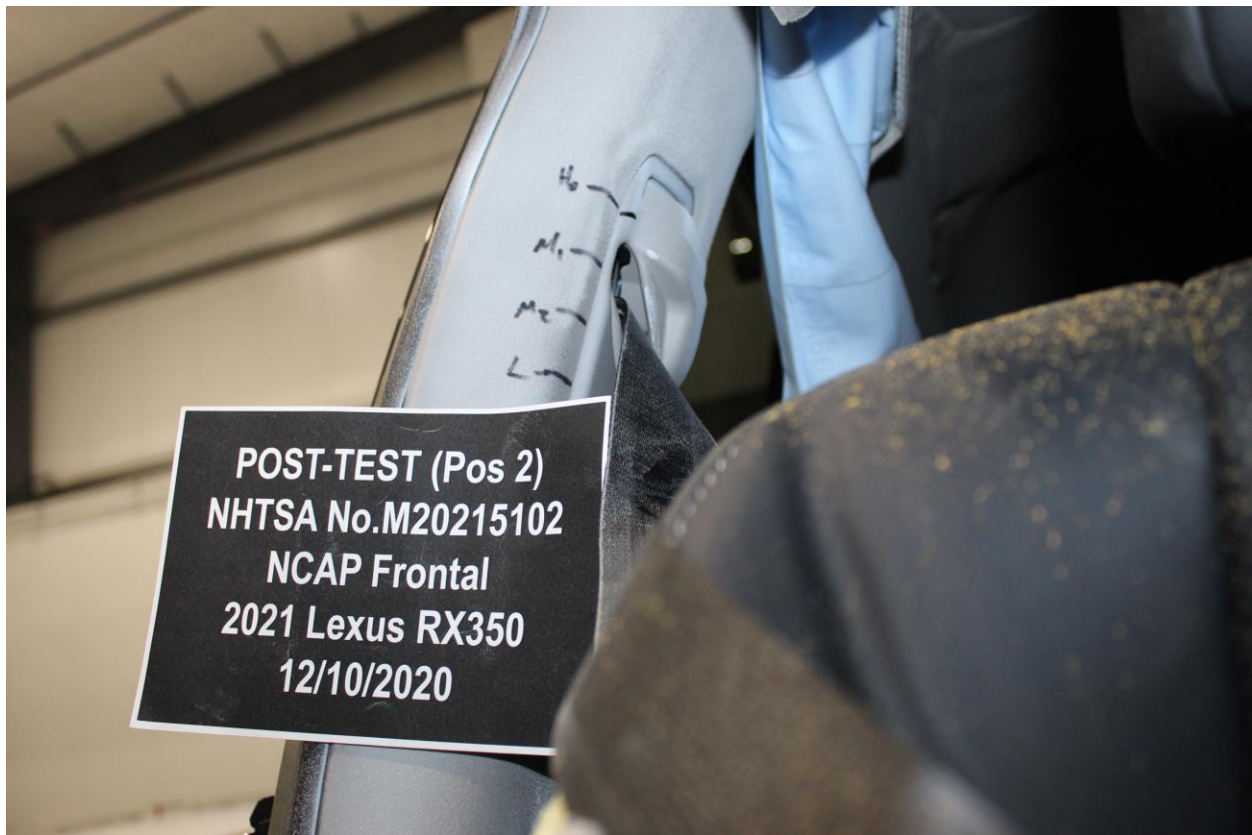
Figure A-62: Post-Test View of Belt Anchorage for Passenger Dummy
