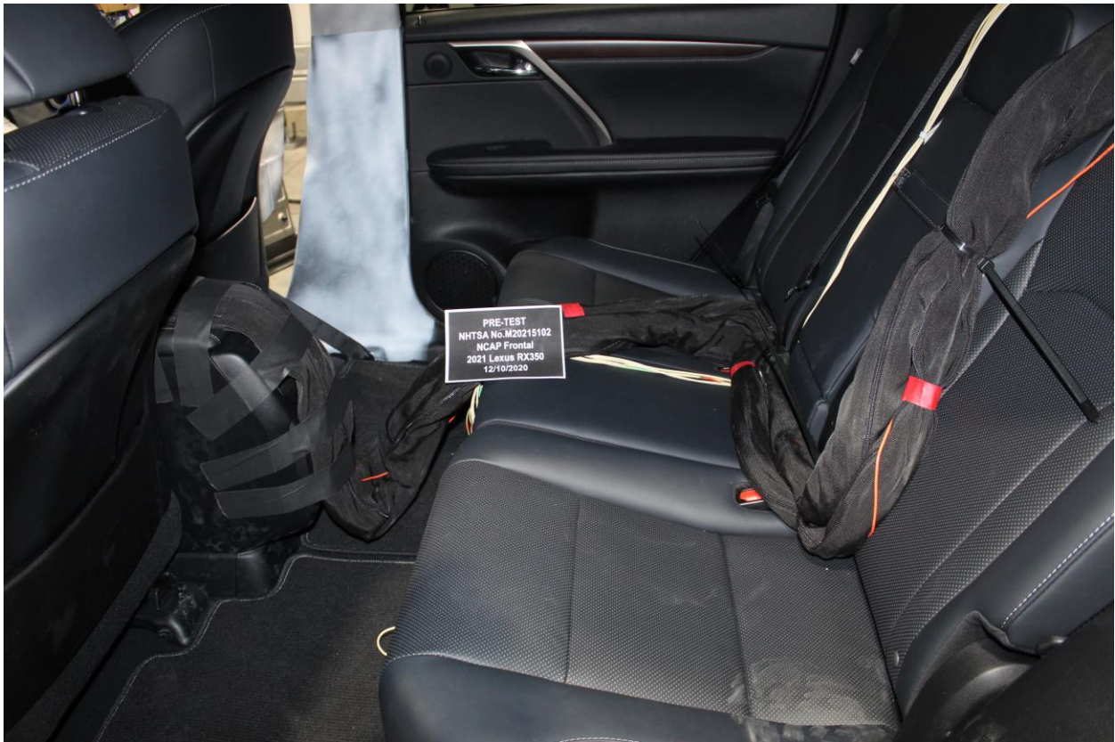
Figure A-28: Pre-Test Dummy Cable Routing
